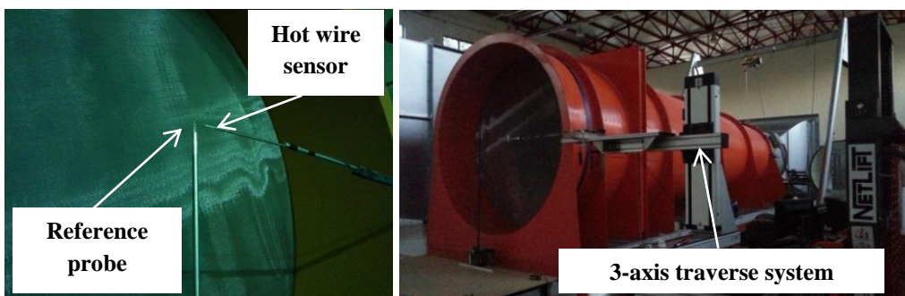
Figure 2.11: Hotwire sensor and reference velocity probe at the jet centerline (left), wind tunnel setup with 3-axis traverse system (right)
