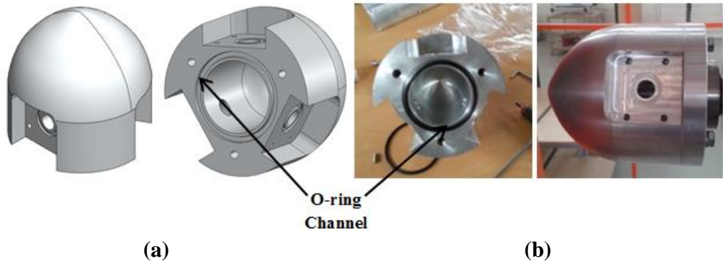
Figure 2.17: (a) Rendered CAD of pressurized hub, (b) pressurized hub after production
