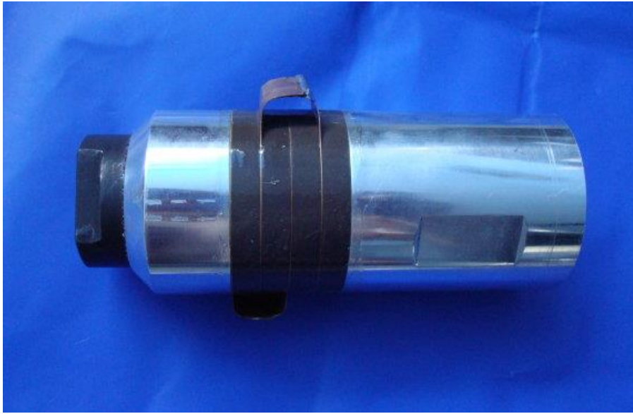
Figure 35 – The transducer used in the set-up
