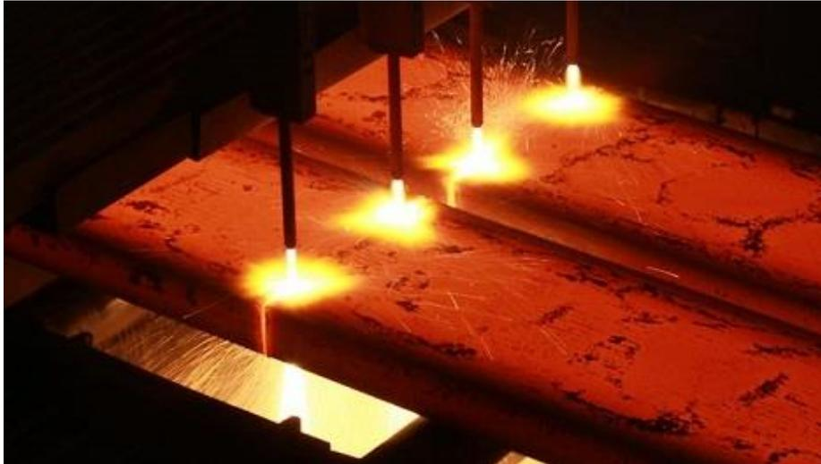
Figure 1.11 Oxy-fuel cutting of a continuous casting slab [43]
