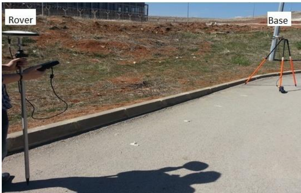
Figure 84 – 5meters Distance Test Setup
