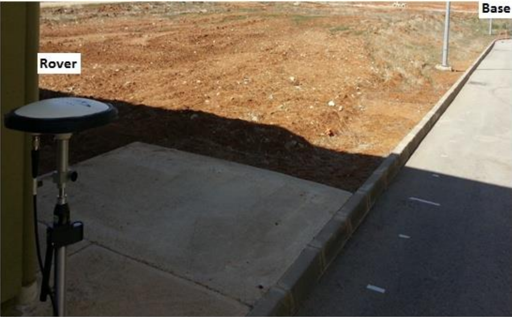
Figure 94 - 50 meters Distance Test Setup
