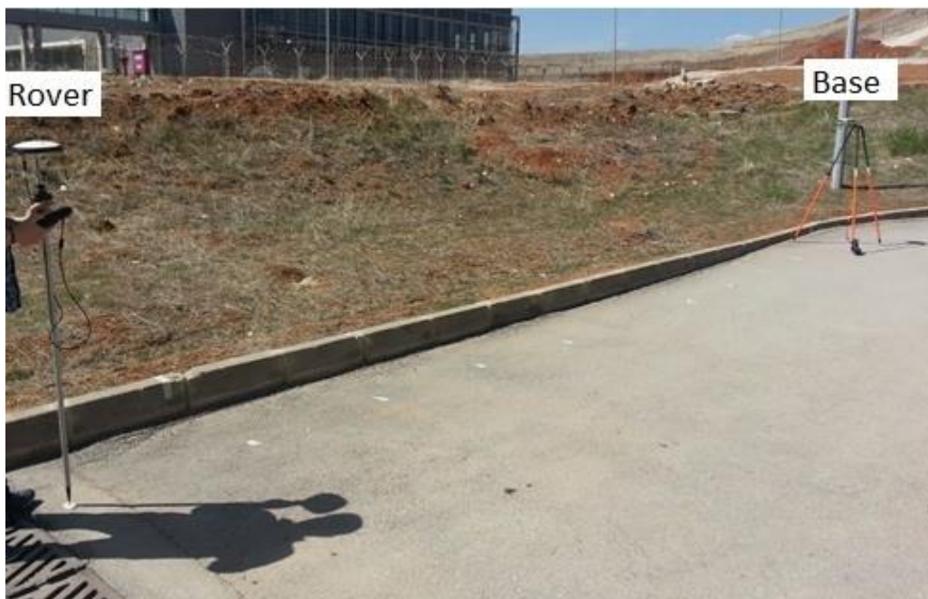
Figure 86 - 10 meters Distance Test Setup
