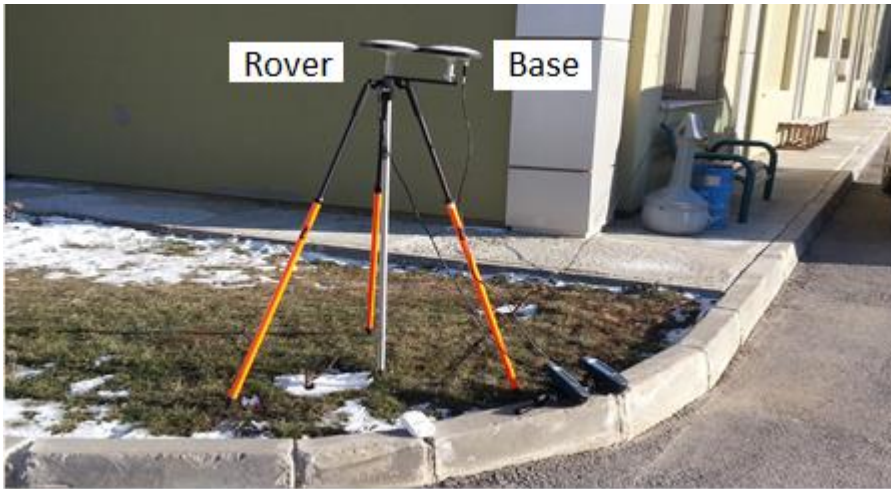
Figure 70 - Test Setup (20cm Baseline Distance)
