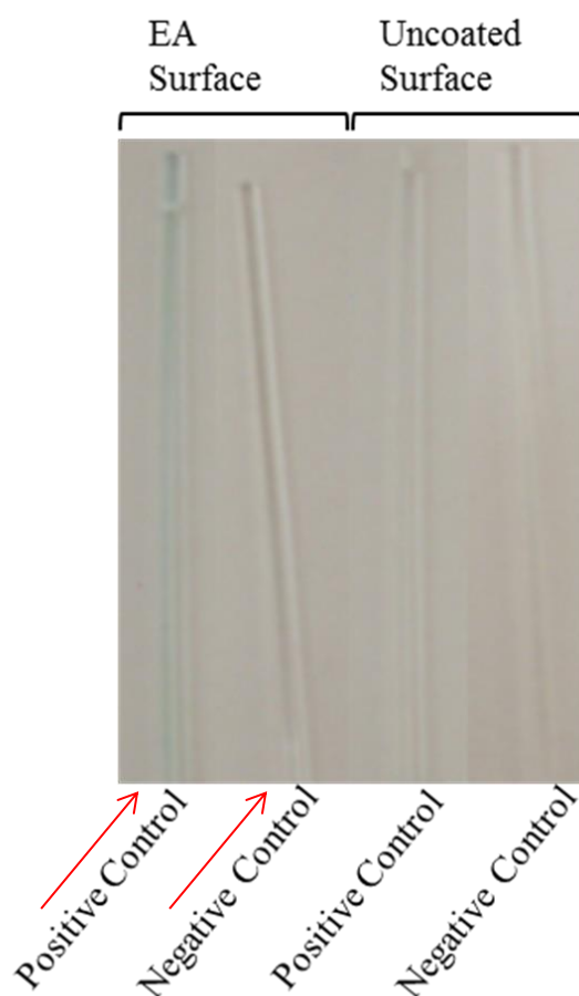
Figure 3. 25 Visual signal observation from HRP-TMB reaction on EA coated and uncoated surfaces. Positive control includes 5' thiol and 3' biotin functionalized probes on surface while the negative control parameter does not contain any oligonucleotide probe.
