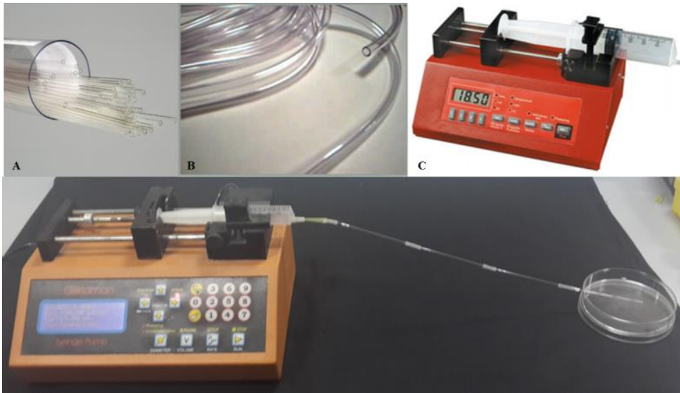
Figure 2. 5 Physical components of the washing platform. A) Glass capillary tubes with an interior diameter of 1,1 mm, B) Plasting tubing material to connect the capillaries each other during filling and washing steps via syringe pump,C) automated syringe pump. Assembly of the components are also given in the image.
