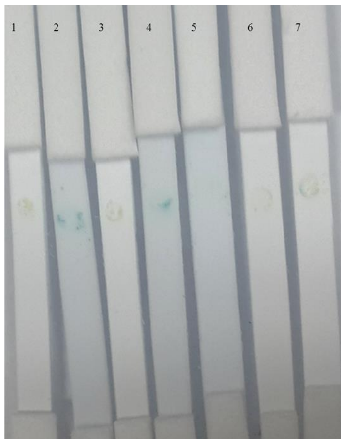
Figure 3. 47 Visualization of HRP catalyzed oxidation of TMB previously embedded in silica nanoparticles on nitrocellulose membrane based lateral flow strips. Reaction is dependent on the hybridization of surface immobilized oligonucleotide with a complementary probe, and design of “strip1” is used which was previously described in Figure 3.43. 1) surface oligonucleotide immobilized TMB embedded silica particles on strip, H_2O_2 delivery through sample pad, 2) surface oligonucleotide immobilized TMB embedded silica particles on strip, H_2O_2 +complementary probe delivery through sample pad, 3) surface oligonucleotide immobilized TMB embedded silica particles on strip, H_2O_2 +uncomplementary probe delivery through sample pad, 4) surface oligonucleotide immobilized TMB embedded silica particles on strip H_2O_2 +MM1 probe delivery through sample pad, 5) surface oligonucleotide immobilized TMB embedded silica particles on strip H_2O_2 +MM2 probe delivery through sample pad, TMB embedded silica particles without surface oligonucleotide on strip, 6) surface oligonucleotide immobilized TMB embedded silica particles on strip H_2O_2 +MM3 probe delivery through sample pad, 7) TMB embedded silica particles without surface oligonucleotide on strip, H_2O_2 delivery through sample pad.
