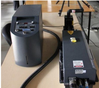
Figure 23-a. New Wave Solo PIV 120 XT-532 nm
