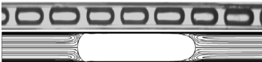
Figure 4. Top: Bubbles visualized in Taylor flow. Bottom: Schematics for the circulations in liquid slugs. Taken from [21], used with permission of Wiley&Sons.
