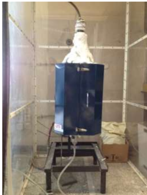
Figure 3.7 The picture of the reactor (located in the furnace) used in the study
