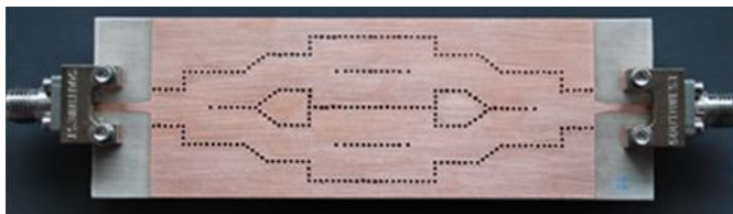
Figure 3.40: The photograph of the produced 1 x 4 Y & Y-Junction SIW power divider using back-to-back configuration
