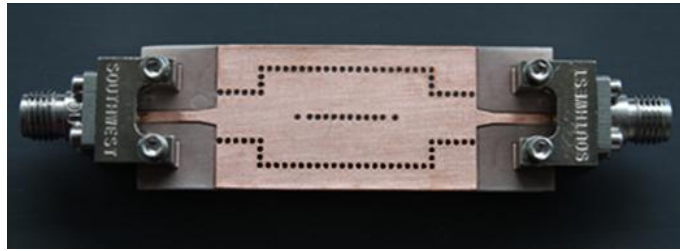
Figure 3.22: The photograph of the produced 1 x 2 Y-Junction SIW power divider using back-to-back configuration
