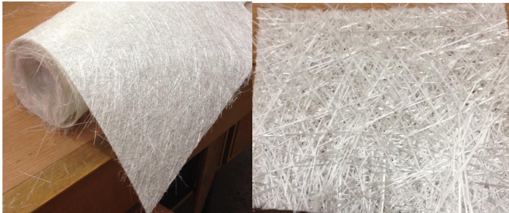
Figure 2.3 Chopped strand glass fiber mat used as the reinforcement in the production experiments
