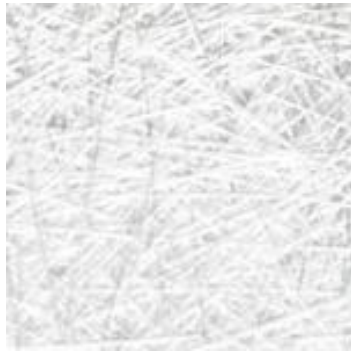
Chopped fiberglass mat (unwoven) Twill weave glass fiber fabric
