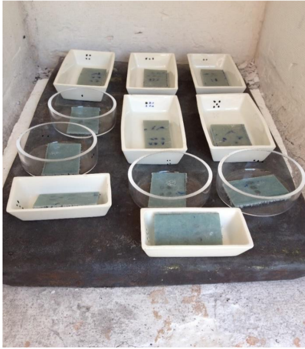
Figure 2.26 The composite samples that are to be sintered, placed in sintering furnace
