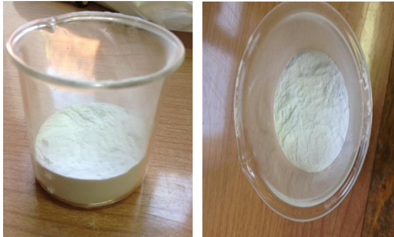
Figure 2.2 Images of the spherical glass particles (Microperl 050-20-215) used as particle fillers in the production experiments
