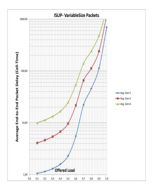
Figure 6.5: ISLIP-Variable Sized Packets, End-to-End Delays
