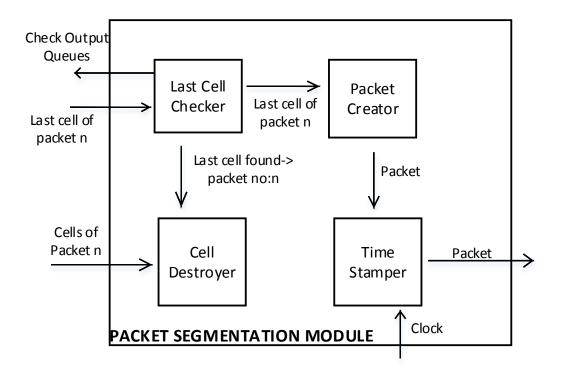
Figure 4.9: Packet Reassembly Submodules
