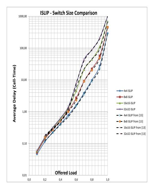
Figure 6.2: ISLIP Algorithm – Effect of Switch Size on Delay Performance
