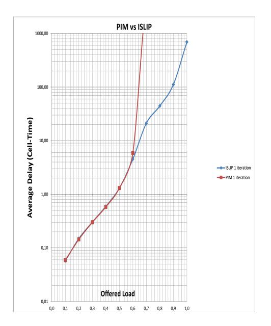
Figure 6.4: Parallel Iterative Matching vs ISLIP
