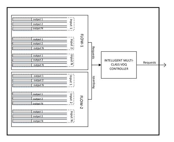
Figure 5.1: New Multi-Class VOQ structure with IMC
