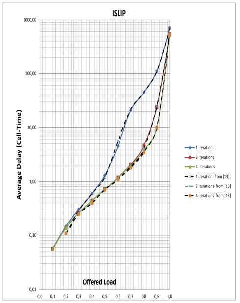
Figure 6.1: ISLIP Algorithm – Effect of Maximum Iteration Number on Delay Performance
