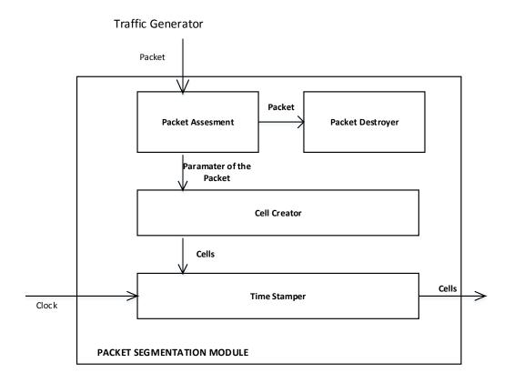
Figure 4.2: Packet Segmentation Submodules
