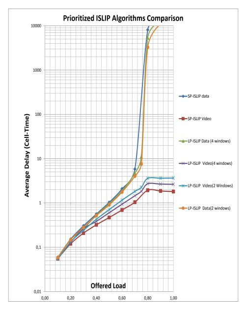
Figure 6.6: 30% video-70% data - Flow Delays
