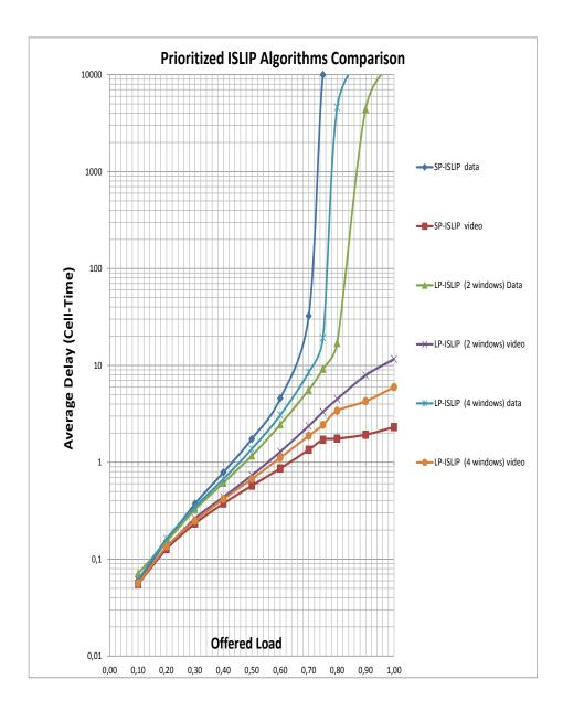
Figure 6.7: 70% video-30% data -Flow Delays
