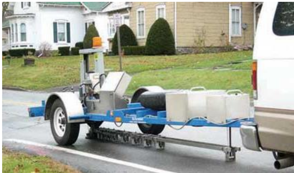
Figure 8 Trailer Mounted FWD Device (“Cornell Local Roads Program” 2005)
