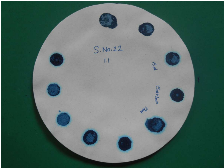
Figure 3.4. Methylene Blue Test Result (Sample No:22)
