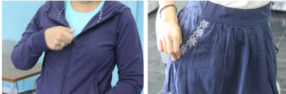
Figure 5.19 Increasing or decreasing the volume by sliding the zip or swiping fingers through the edge of the skirt's pocket
