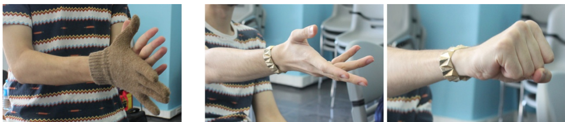
Figure 5.23 Playing and pausing songs: Gloves sensing the clapping of the hands; the bracelet sensing the muscular movements specific to the each hand gesture which corresponds to play and pause in order, from left to right
