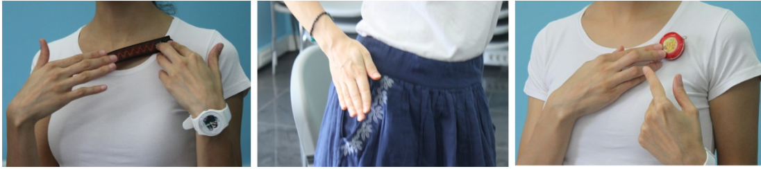
Figure 5.15 Pausing and playing the song by a tap on the flat necklace, a tap on the skirt, touching on the front flat surface of the brooch
