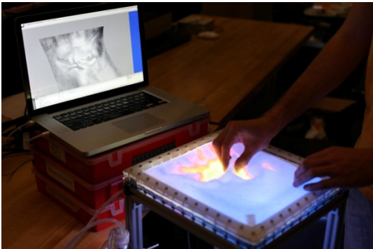
Figure 2.12 Tunable Clay: Malleable interface used for 3d modelling which use optical sensing technology (MIT Media Lab, 2012).
