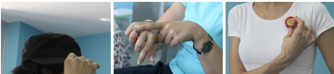
Figure 5.18 Skipping to the next or previous song by turning the hat, turning the circular piece on the ring and turning the brooch in clockwise or counterclockwise.
