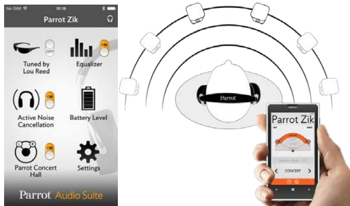
Figure 3.26 Parrot Audio Suite App where users activate or deactivate Active Noise Cancellation, Concert Hall Mode and adjust audio frequency through Equalizer (Parrot, 2014).
