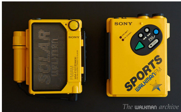
Figure 3.9 Solar powered (on the left) and the waterproof (on the right) Walkmans (Stereo2go, 2014).
