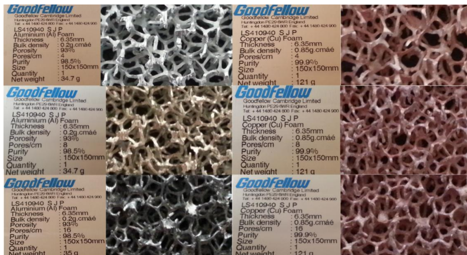
Figure 4.2 Pictures of the metal foams and packages
