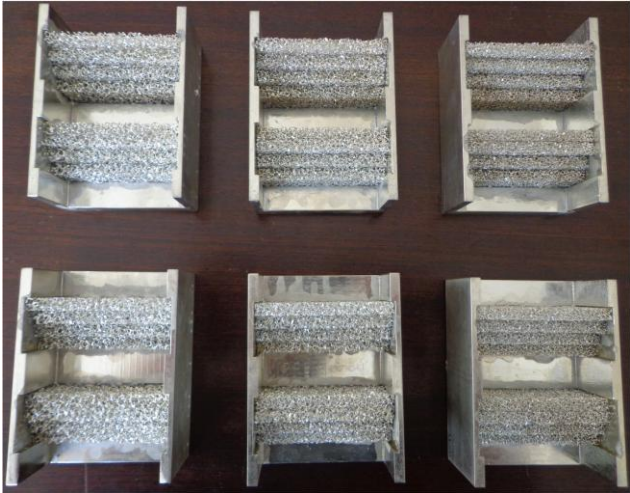
Figure 4.7 Pictures of foam embedded heat sinks
