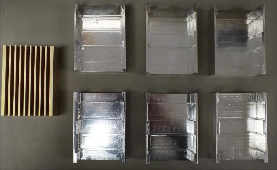
Figure 3.6 Photograph of test specimen chassis after coating process
