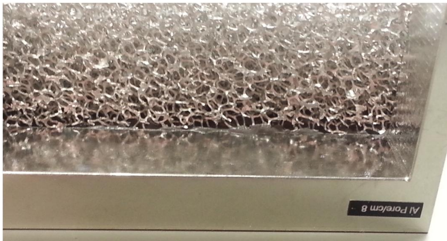
Figure 3.10 Junction of foam to chassis before melting
