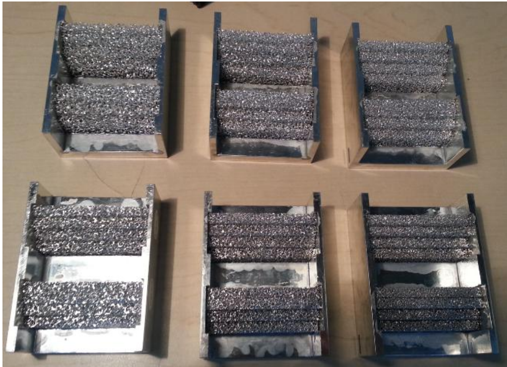
Figure 3.14 Final form of soldered metal foam test specimens
