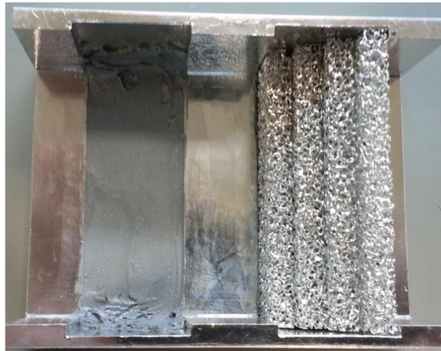
Figure 3.9 Cream solder application process after one side of foam located
