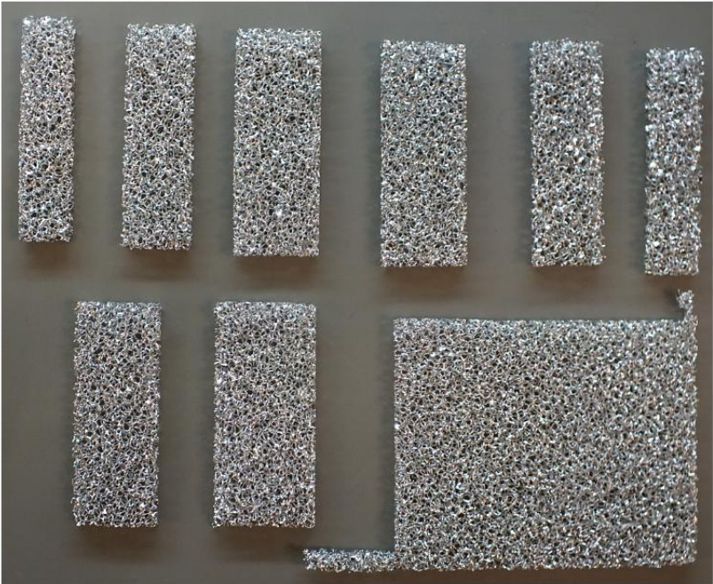
Figure 3.7 Photograph of metal foams after coating process
