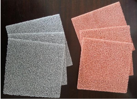
Figure 4.3 Pictures of the metal foams
