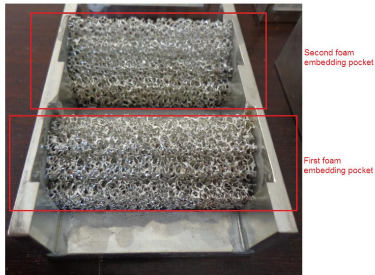
Figure 4.8 Pictures of the foam soldered pockets
