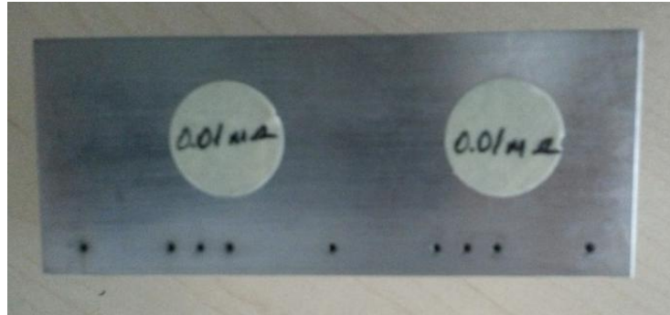
Figure 3.4 Specimen holes after deep drilling
