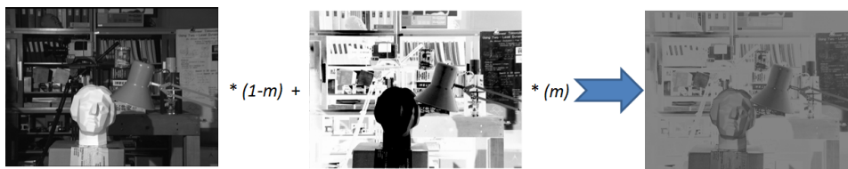
Figure 4.4: Figure illustrating the method for generating images of different multi-modality. m : the multi-modality level scale ( m=0.5 in this case) Left image : Original Tsukuba image from Middlebury image database Middle image : Cosine transformed image Right image : Generated image of multi-modality level m=0.5
