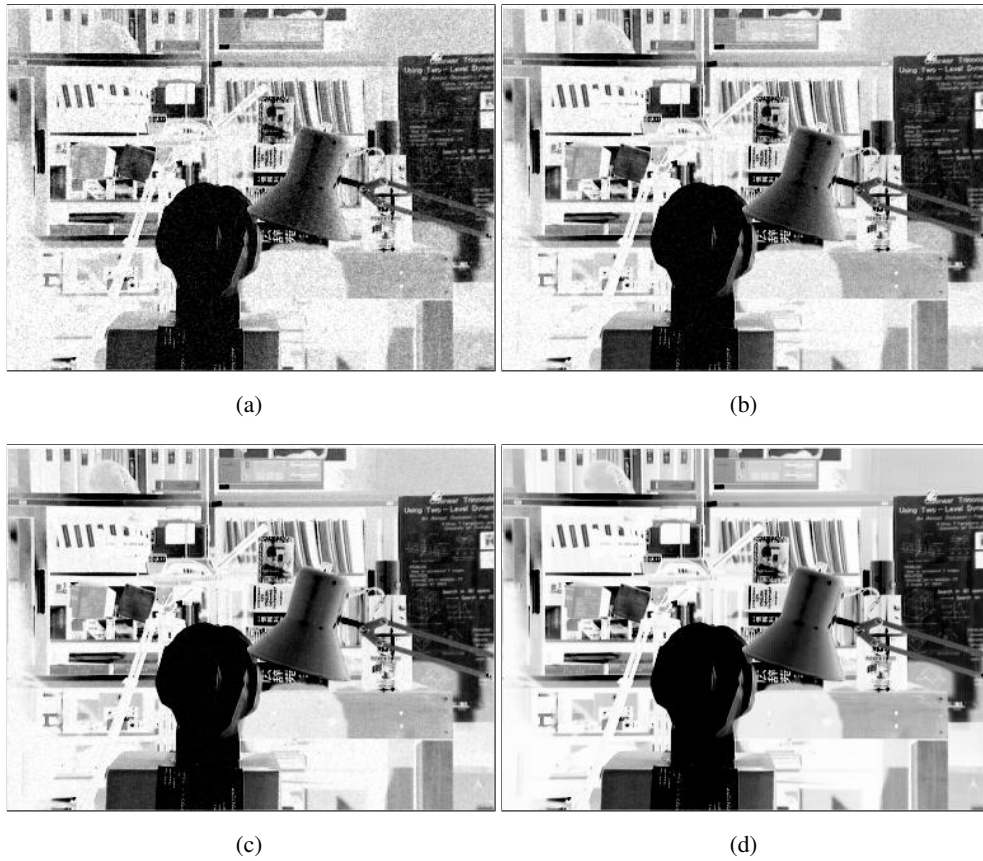
Figure 4.8: Different noise levels applied to left Tsukuba image in Dataset #1. (a) Noise level n = 10 ( \sigma = 20.0 ) (b) Noise level n = 6 ( \sigma = 12.0 ) (c) Noise level n = 3 ( \sigma = 6.0 ) (d) Noise level n = 0 ( \sigma = 0.0 ) the noiseless cosine transformed left image.
