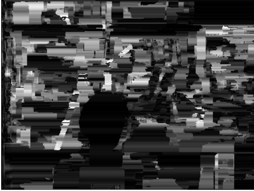
Figure 5.5: Cost Confidences for Tsukuba image pair (scaled and truncated to [0..255] range for the sake of visibility).
