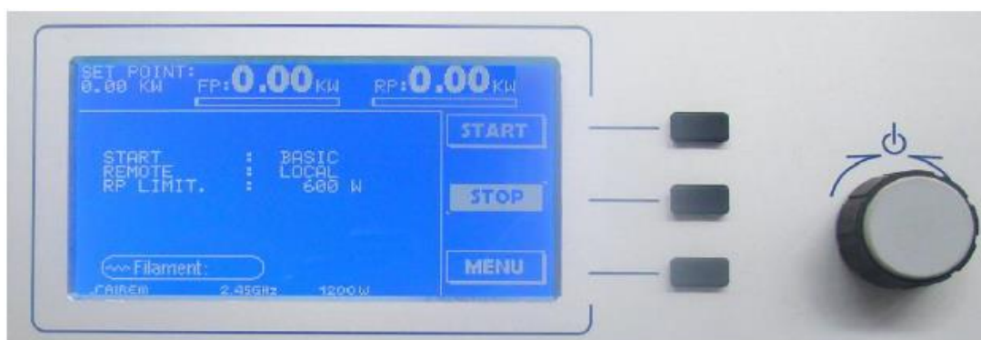
Figure B.2. Front panel of the power supply
