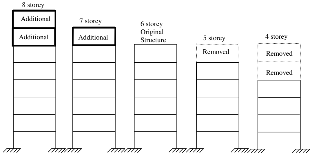
Figure 4.8. Modification of Height Ratio of the Structures
