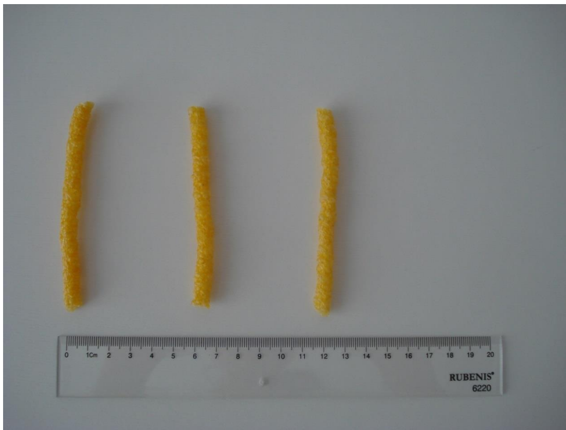
Figure 7. Images of the extrudates extruded with 25 \pm 0.5\% moisture content of feed at 130^{\circ}\text{C} forth zone temperature and at 225 rpm with feed flow rate of 36 g/min ( 14.57 \pm 0.01\% moisture and 8.52 \pm 0.61 mm diameter).
