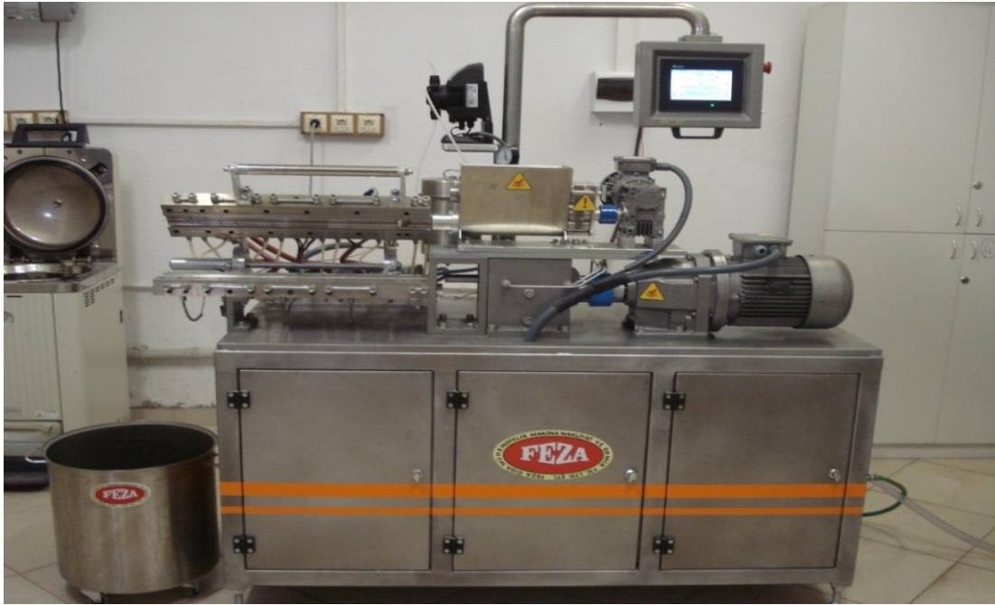
Figure 4. Laboratory scale co-rotating twin screw extruder used in the study.
