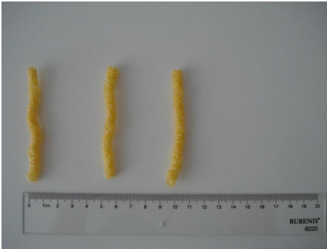
Figure 8. Images of the extrudates extruded with 25 \pm 0.5\% moisture content of feed at 160^\circ\text{C} forth zone temperature and at 225 rpm with feed flow rate of 36 g/min ( 14.27 \pm 0.02\% moisture, 6.96 \pm 0.53 mm diameter).
