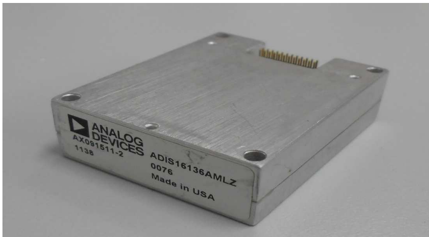
Figure 2.8: The ADIS16136 sensor is shown in the metallic casing. The sensor has same connections as ADIS16488 and hence can be used with same evaluation board.
