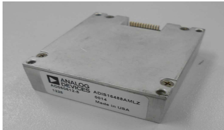
Figure 2.6: ADIS16488 IMU with metallic casing. This protective casing limits the operation of this sensor by heating up.
