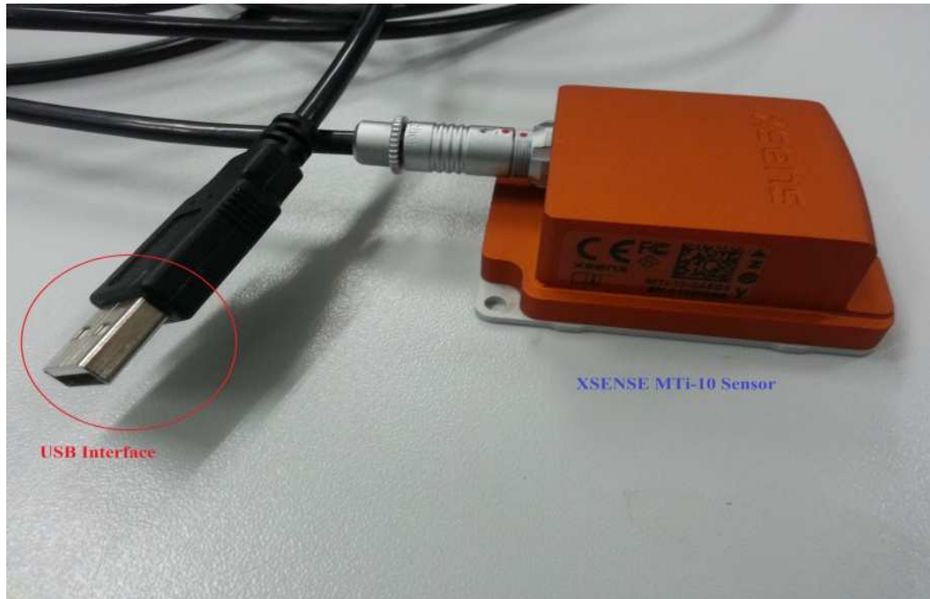
Figure 2.11: The figure shows the XSENS sensor and its USB interface. No evaluation board is required for data acquisition from this sensor.
