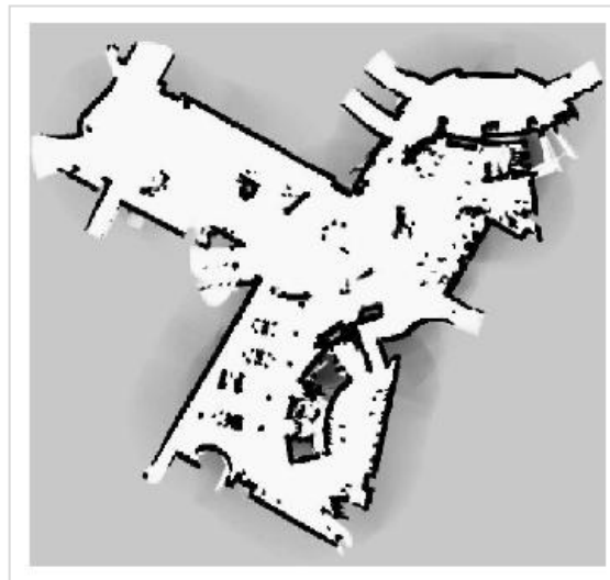
Figure 2-4 A sample map with occupancy grids [1].
