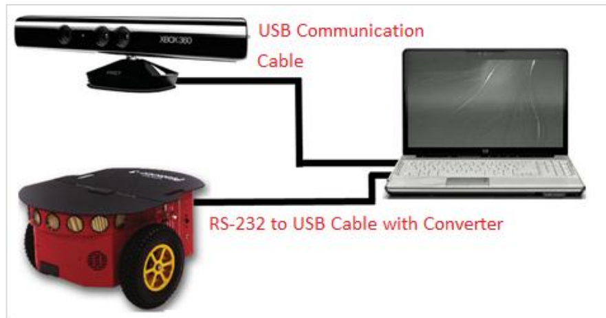
Figure 3-7 The robot system, computer and sensor connection
