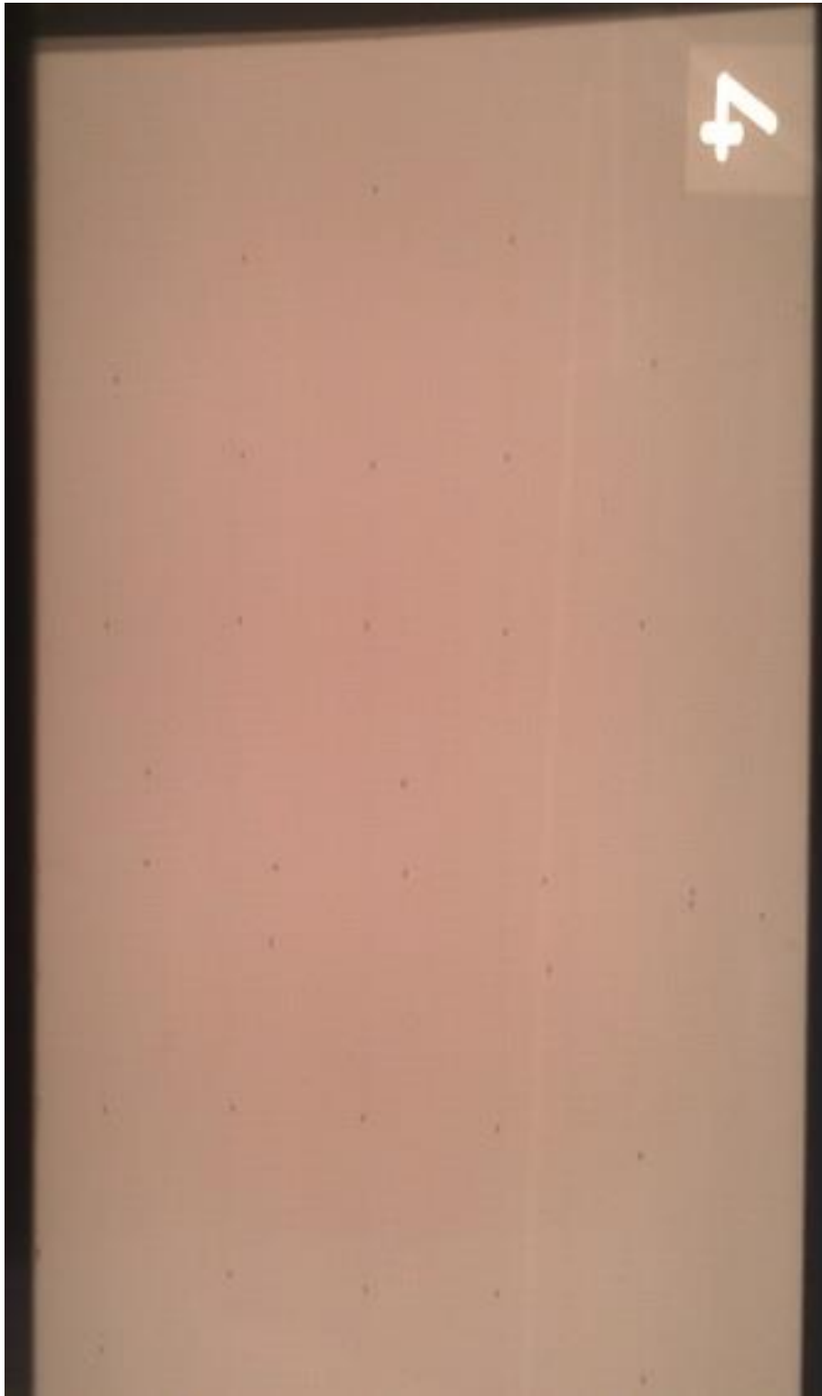
Figure 3.16. X-ray photo of the fourth horizontal resin infusion sample containing holes.0.3
