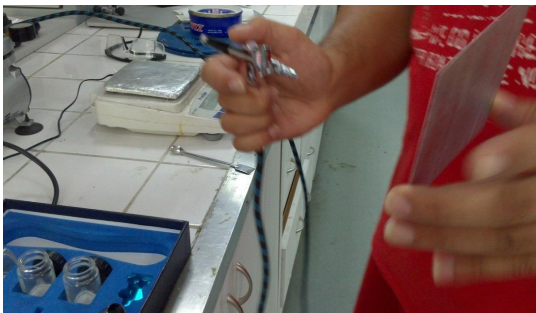
Figure 3.18. Silane treatment of aluminum substrates..0.5
