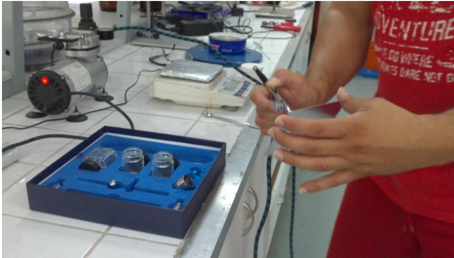
Figure 3.8. Spraying of the prepared silane solution to the aluminum surfaces.0.1
