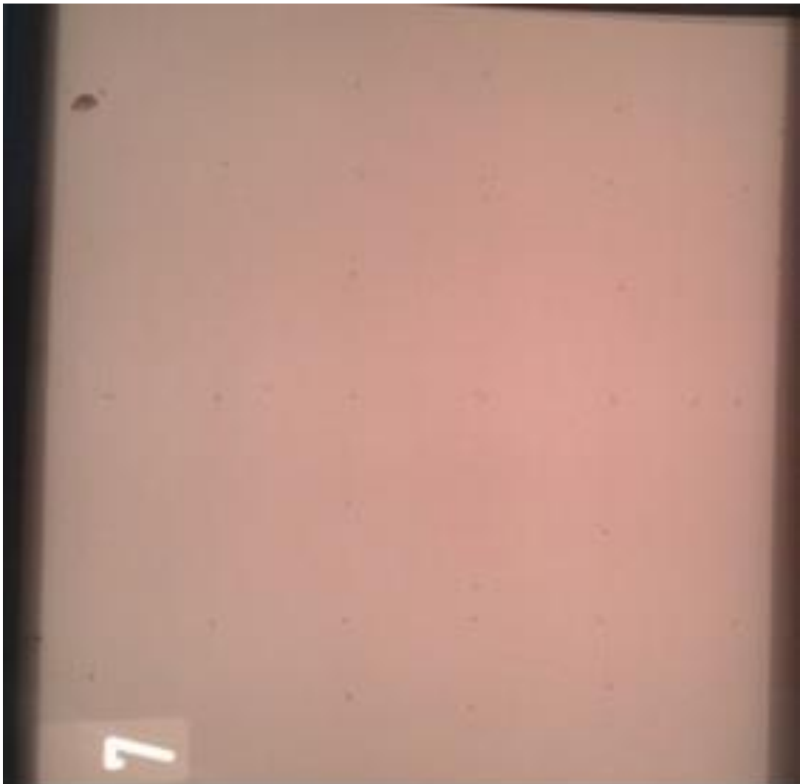
Figure 3.22. Horizontal resin infusion sample containing holes as shown.0.4
