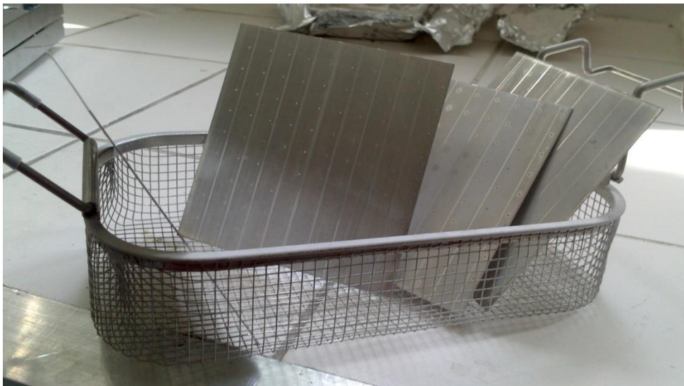
Figure 3.6. 2024 T3 Aluminum alloy sheets used in this study. 0.1
