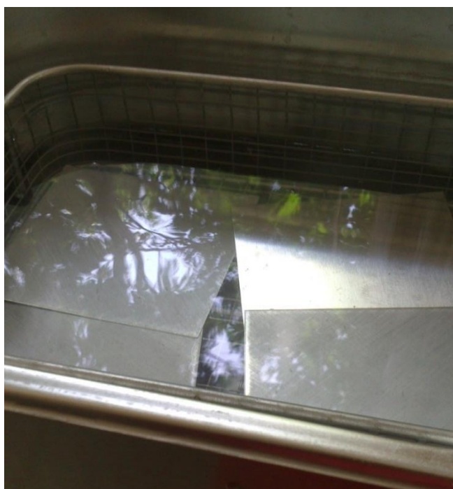
Figure 3.17. Ultrasonic cleaning of aluminum substrates after sand paper abrasion.0.4
