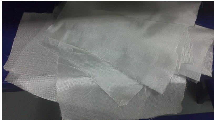
Figure 3.7. Glass fiber woven fabrics used in this study. Figure 2
