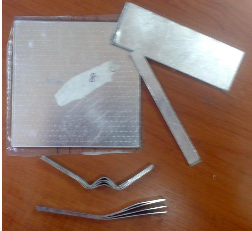
Figure 3.20. Fiber metal laminate composites sliced with micro cutter.0.2
