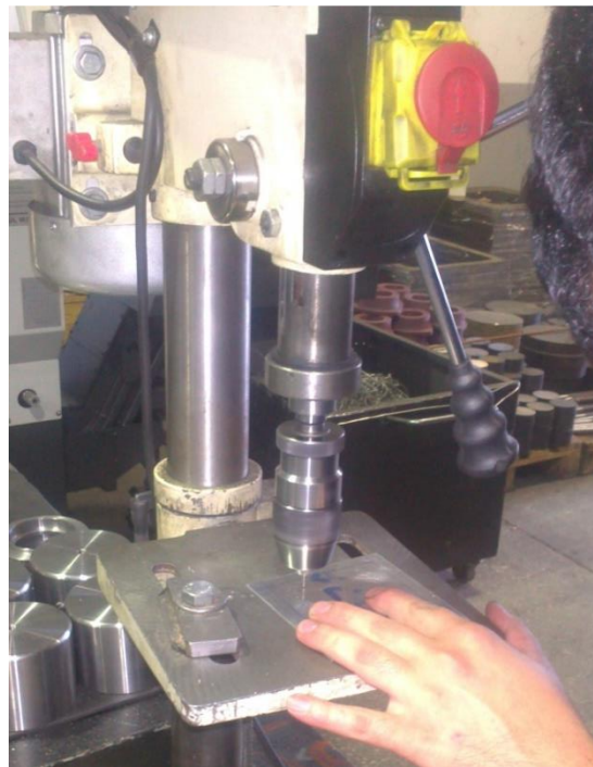
Figure 3.14. Drilling of holes on 2024 T3 aluminum alloy.0.1
