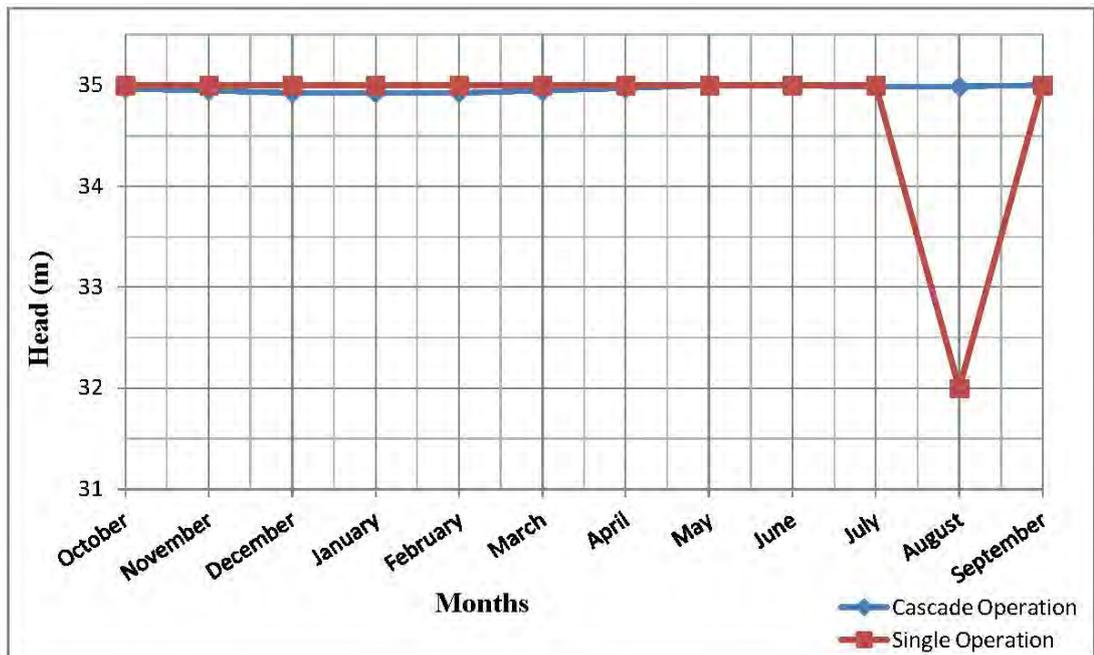
Figure 4-22: Operation head for B2 with average flow data
