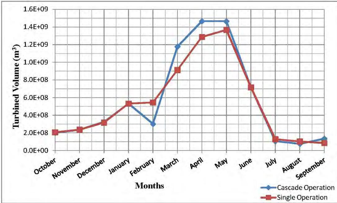
**Figure 4-47:** Turbined volume for UK with maximum flow data with spillway upper bound
