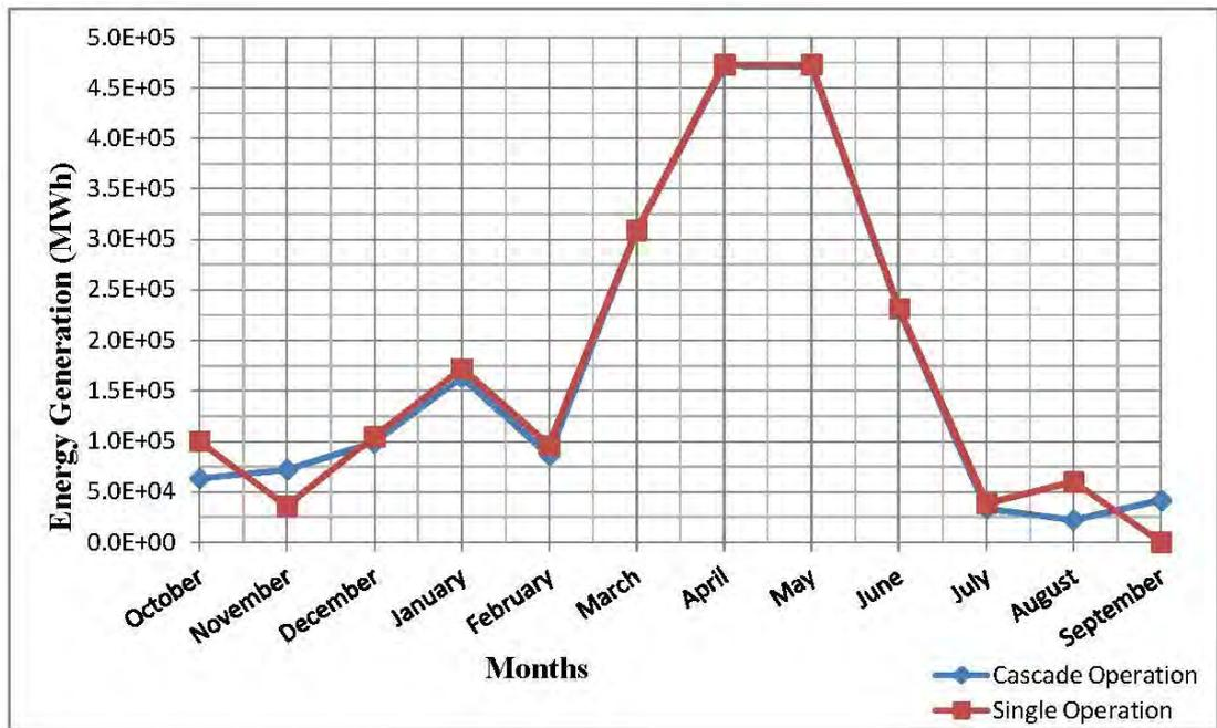
**Figure 4-39:** Energy generation for UK with maximum flow data without spillway upper bound
