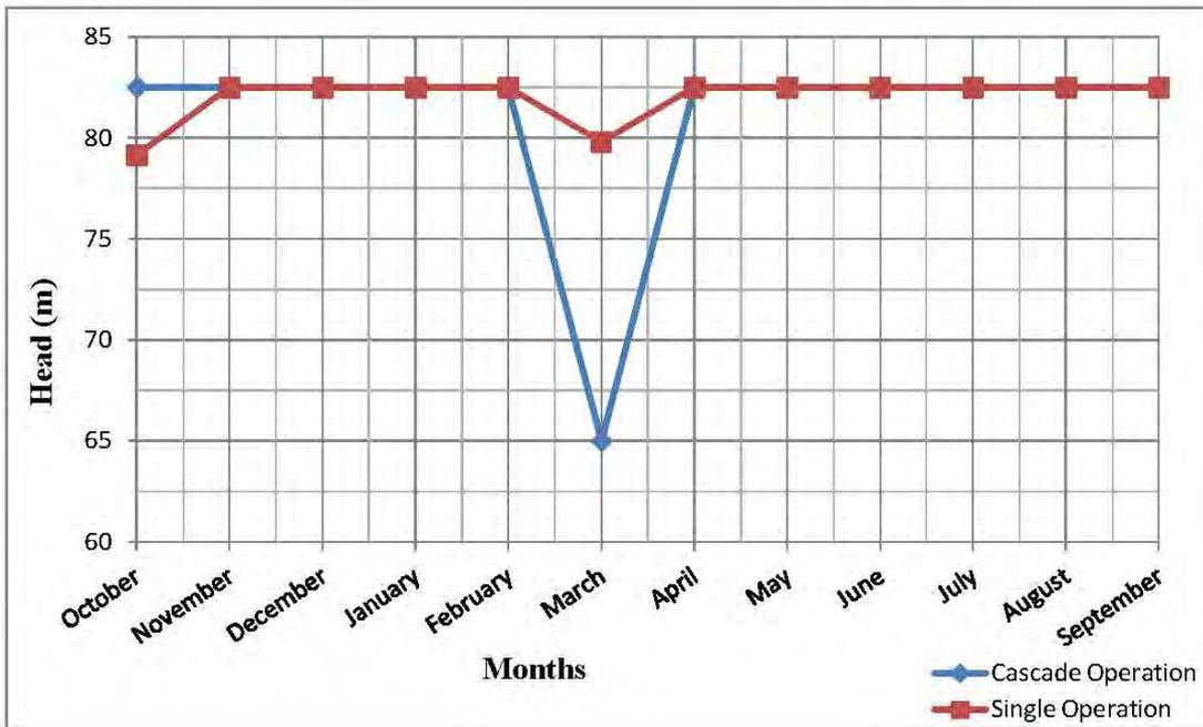
Figure 4-44: Operation head for LK with maximum flow data with spillway upper bound
