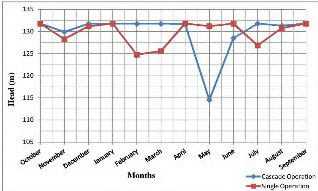
Figure 4-19: Operation head for UK with average flow data
