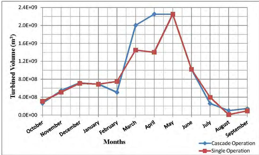
**Figure 4-49:** Turbined volume for B1 with maximum flow data with spillway upper bound
