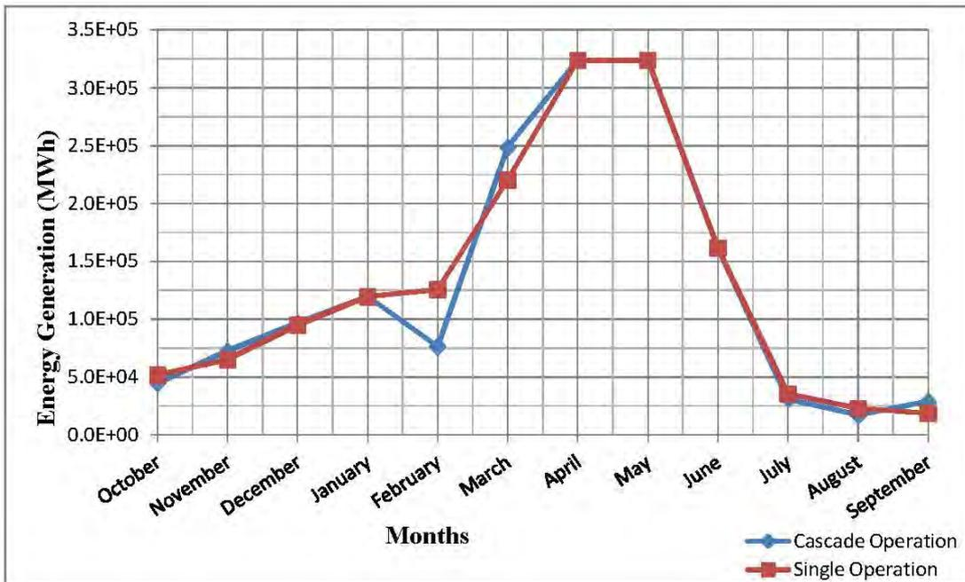
**Figure 4-52:** Energy generation for LK with maximum flow data with spillway upper bound
