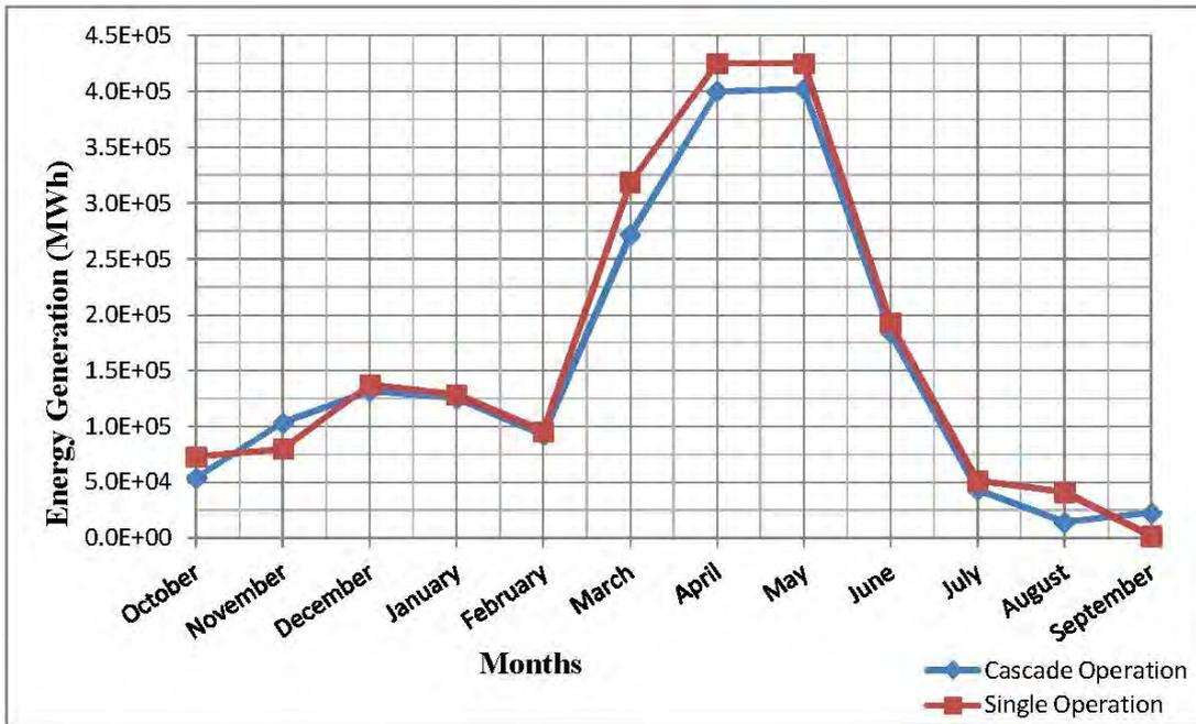
**Figure 4-41:** Energy generation for B1 with maximum flow data without spillway upper bound
