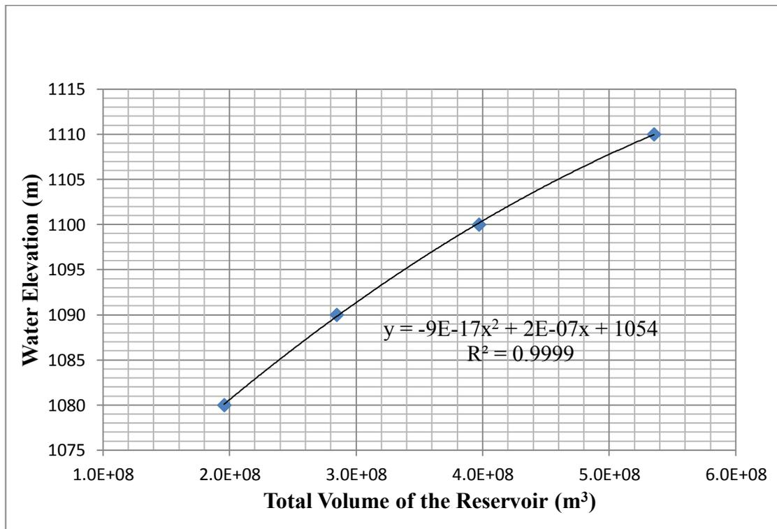
**Figure 4-4:** Water elevation vs. volume curve for LK
