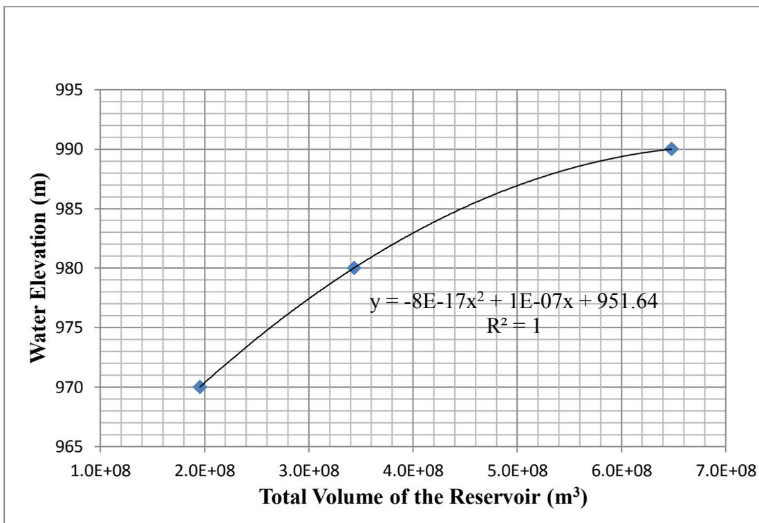
**Figure 4-5:** Water elevation vs. volume curve for B1
