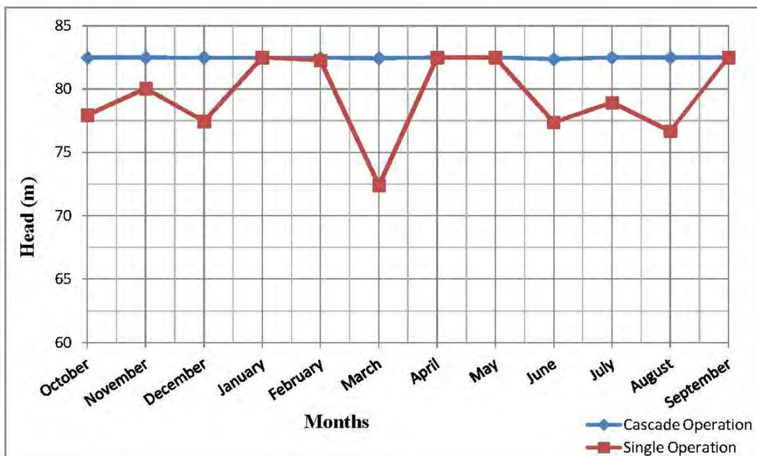
Figure 4-20: Operation head for LK with average flow data
