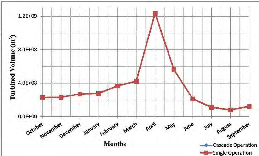
Figure 4-14: Turbined volume for B2 with minimum flow data
