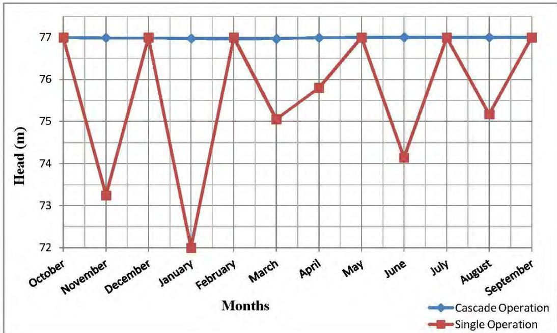
Figure 4-21: Operation head for B1 with average flow data
