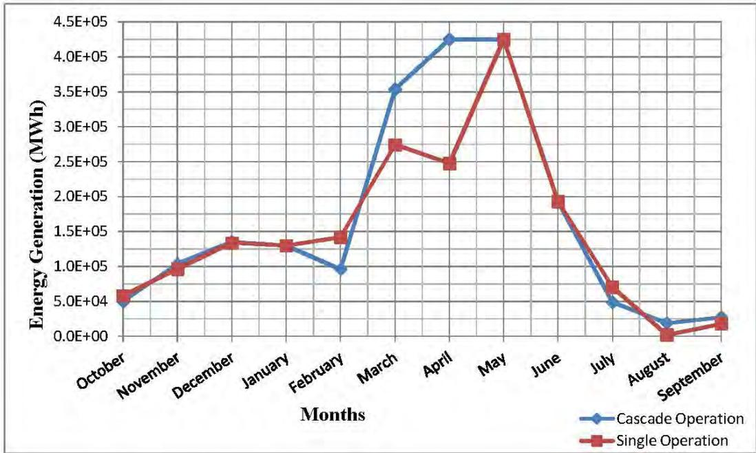
**Figure 4-53:** Energy generation for B1 with maximum flow data with spillway upper bound
