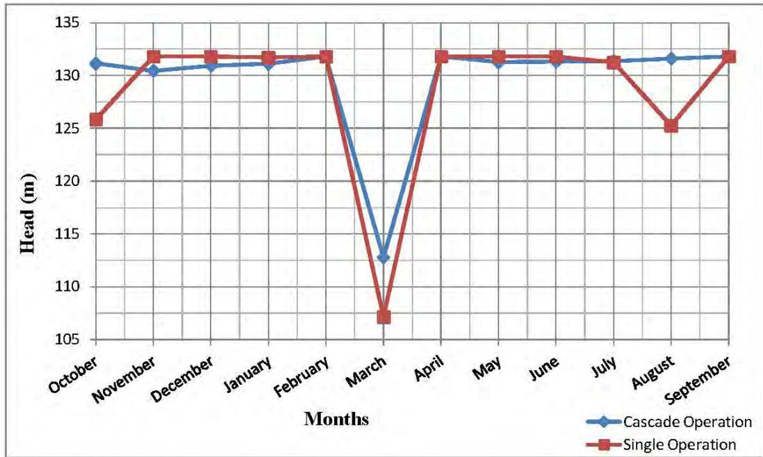
**Figure 4-31:** Operation head for UK with maximum flow data without spillway upper bound
