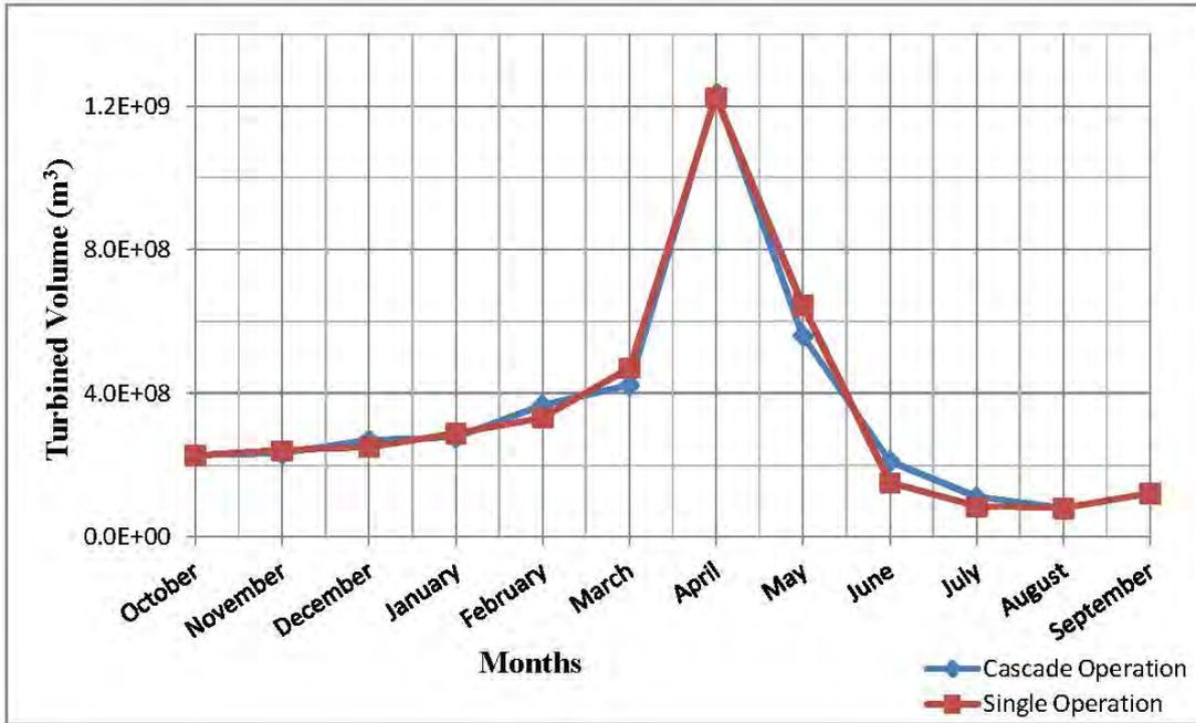
Figure 4-13: Turbined volume for B1 with minimum flow data
