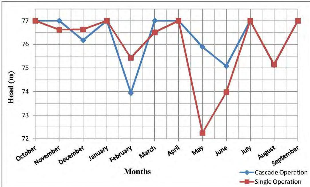
Figure 4-9: Operation head for B1 with minimum flow data
