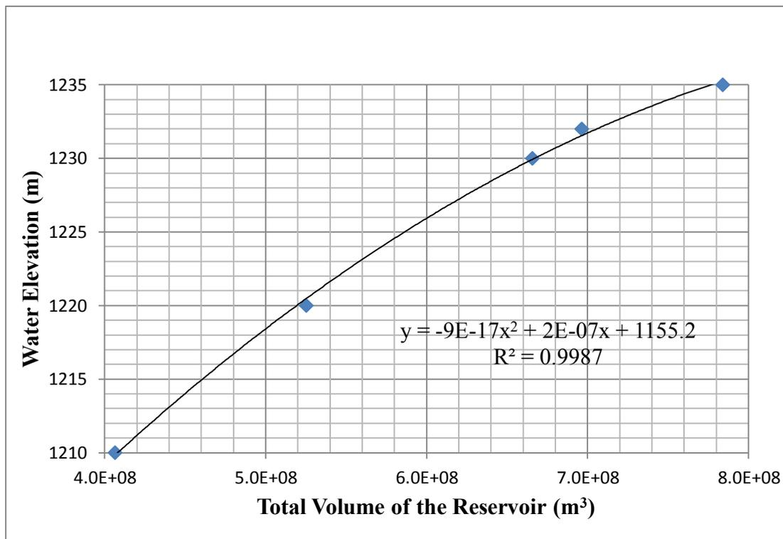
**Figure 4-3:** Water elevation vs. volume curve for UK
