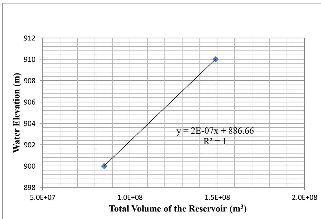
**Figure 4-6:** Water elevation vs. volume curve for B2
