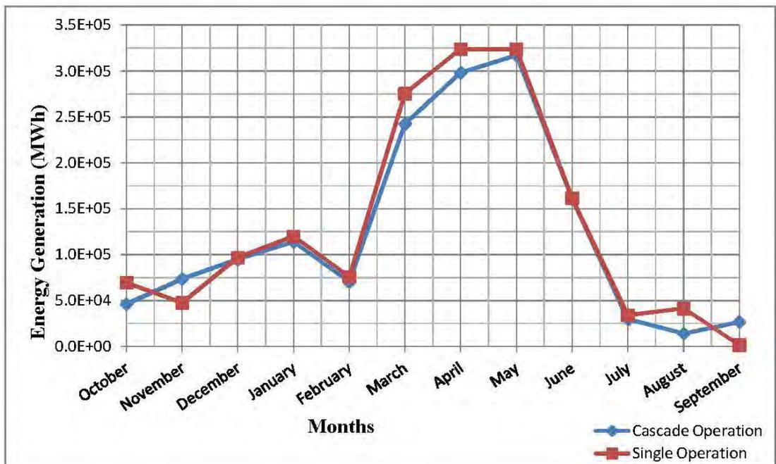
**Figure 4-40:** Energy generation for LK with maximum flow data without spillway upper bound
