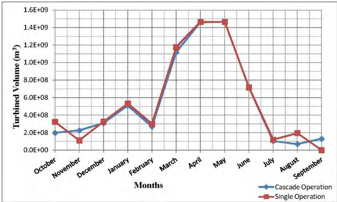
Figure 4-35: Turbined volume for UK with maximum flow data without spillway upper bound
