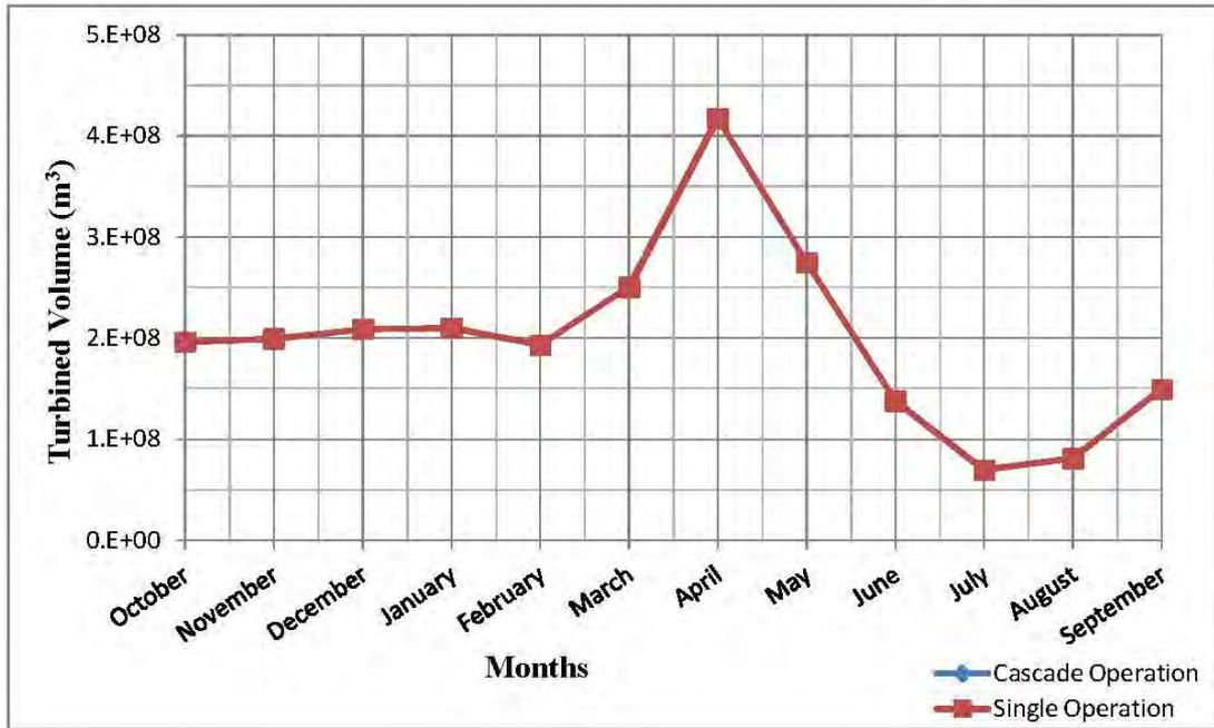
Figure 4-11: Turbined volume for UK with minimum flow data
