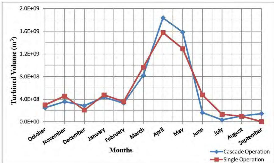
Figure 4-26: Turbined volume for B2 with average flow data
