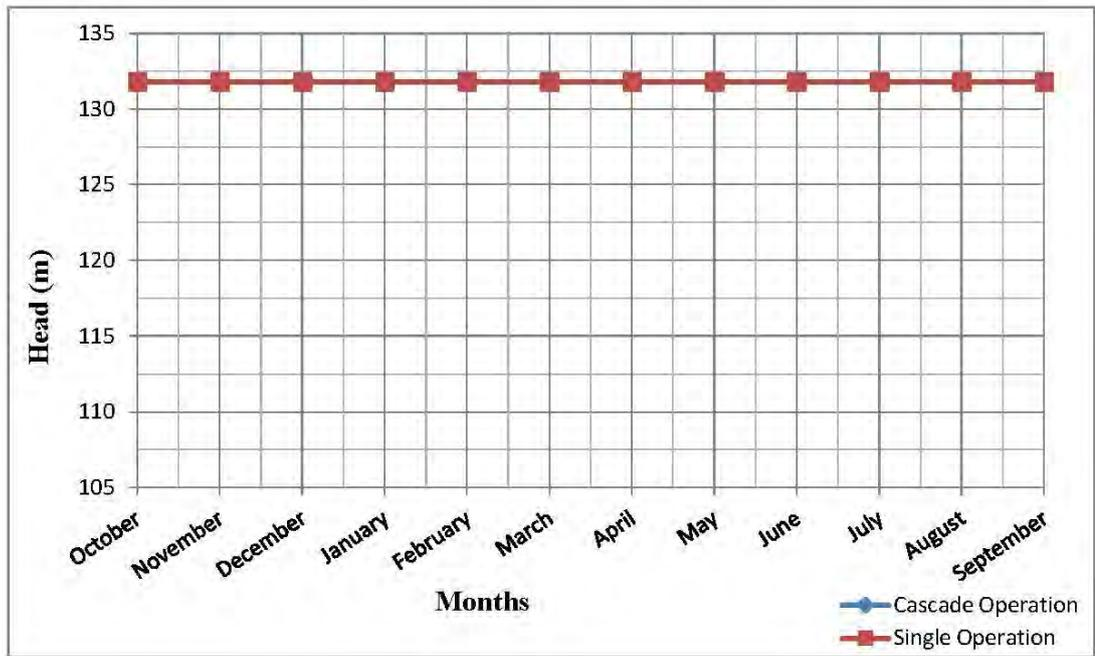
Figure 4-7: Operation head for UK with minimum flow data
