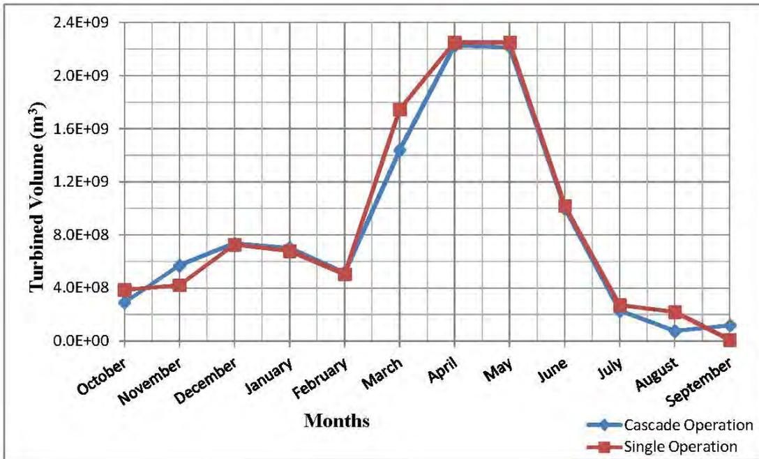
Figure 4-37: Turbined volume for B1 with maximum flow data without spillway upper bound
