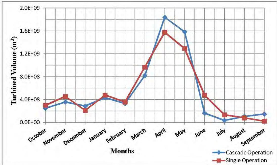
Figure 4-25: Turbined volume for B1 with average flow data
