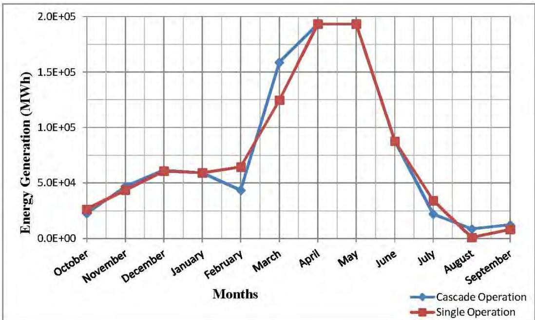
**Figure 4-54:** Energy generation for B2 with maximum flow data with spillway upper bound
