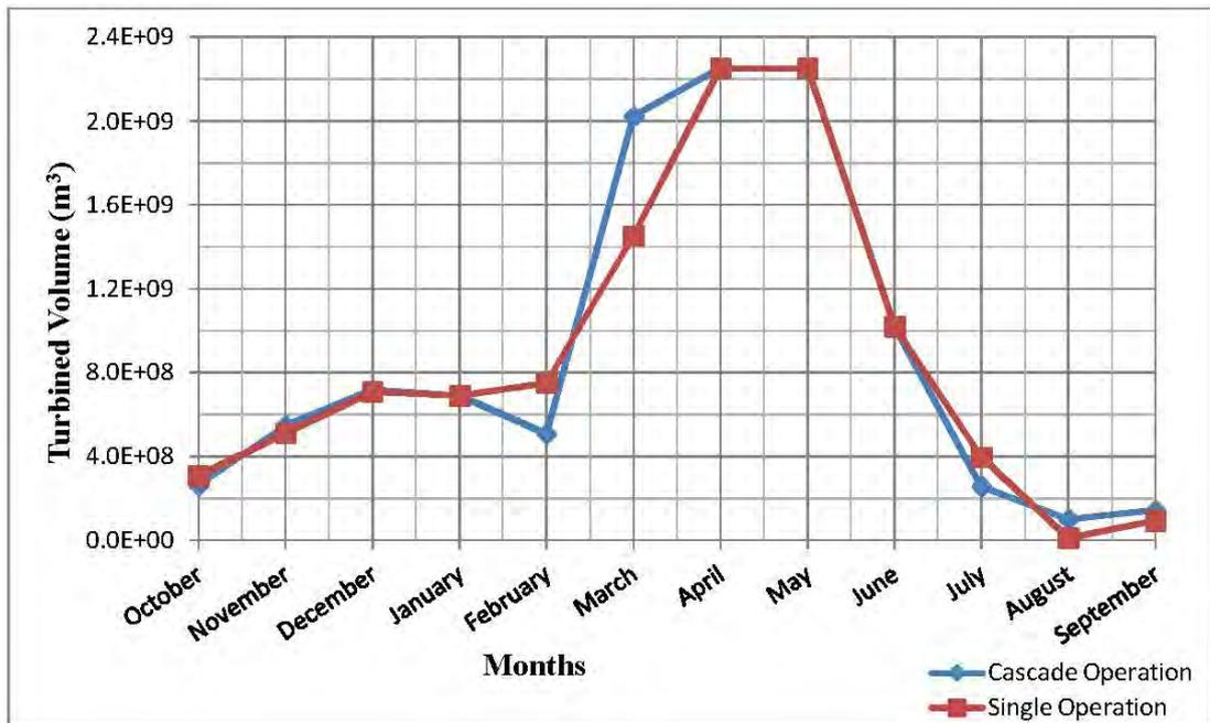
**Figure 4-50:** Turbined volume for B2 with maximum flow data with spillway upper bound
