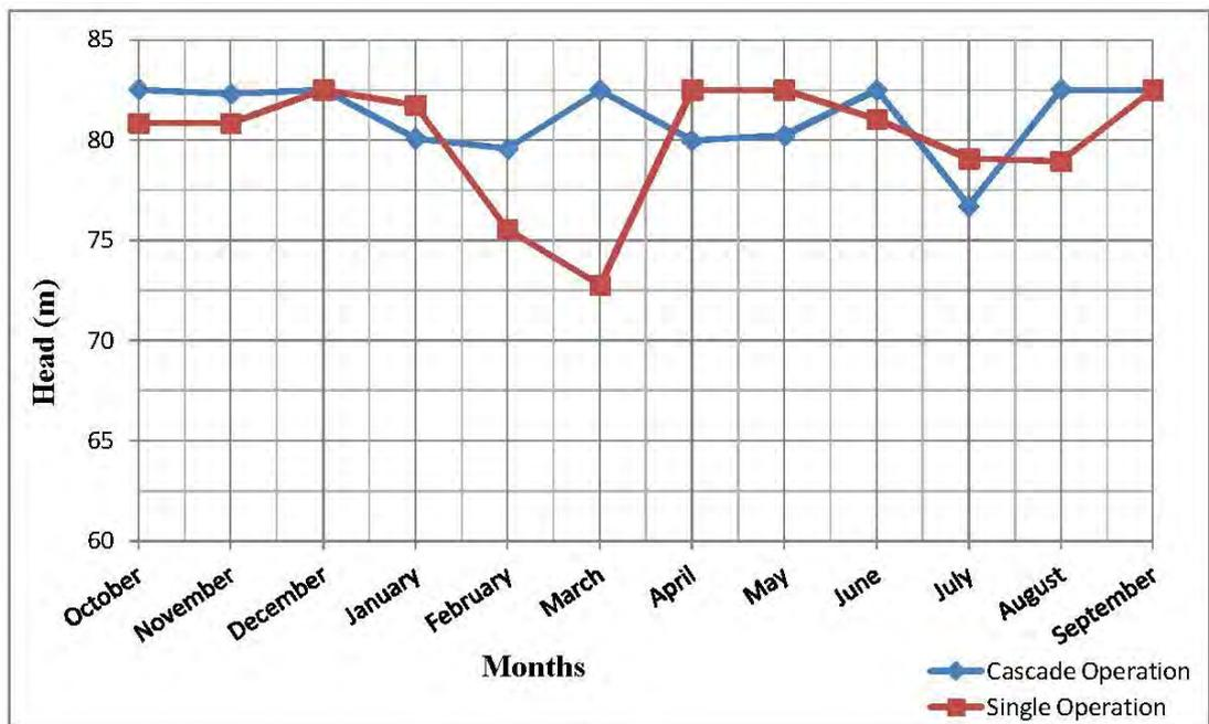
Figure 4-8: Operation head for LK with minimum flow data
