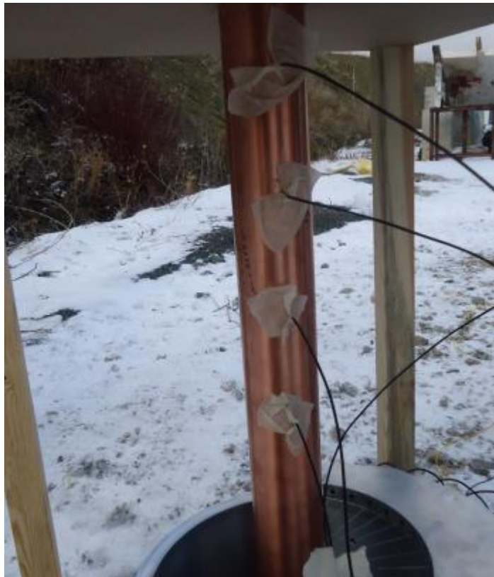
Figure 3-10 Optical Probes and Fiber Optic Cables that are used for Measuring the Detonation Velocity of the Explosive
