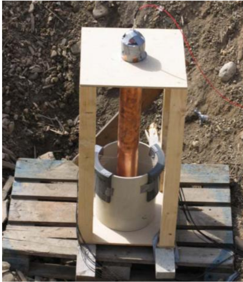
Figure 2-5 Cylinder Expansion Test Setup Used by Esen et al. [5]
