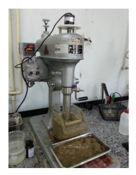
Figure 7: Denver-Sub A Laboratory Flotation Machine
