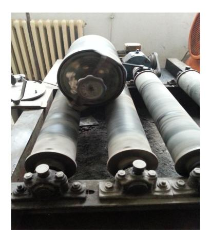
Figure 9: Laboratory Rod Mill
