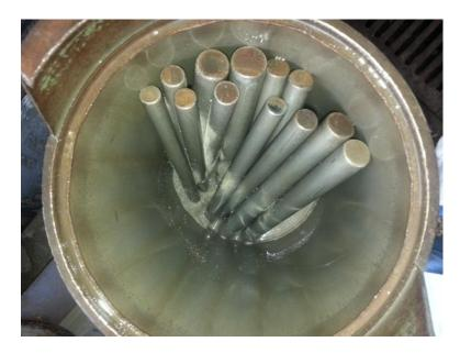
Figure 10: Grinding Mill Charge
