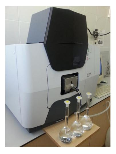
Figure 14: Atomic Absorption Spectrophotometer (AAS)
