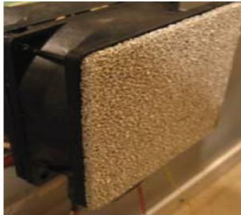
Figure 3 – An axial fan with an inlet diffuser [6]
