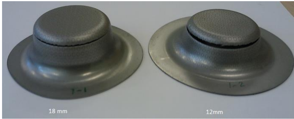
Figure 7.12. The fractured specimens in the 18 and 12 mm punch travels for DKP6112 material
