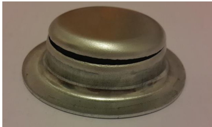
Figure 7.13. The fractured cup in 14.5 mm of punch travel for AA5450 material
