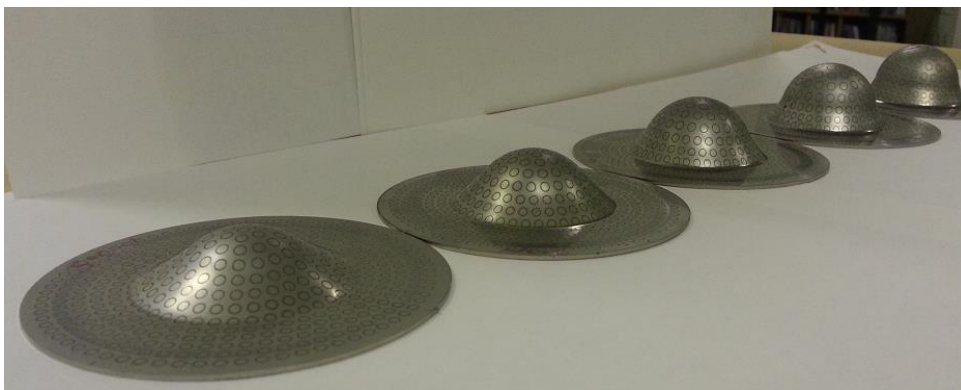
Figure 7.6. Various specimens with different heights deformed in the Erichsen test for SS304 material
