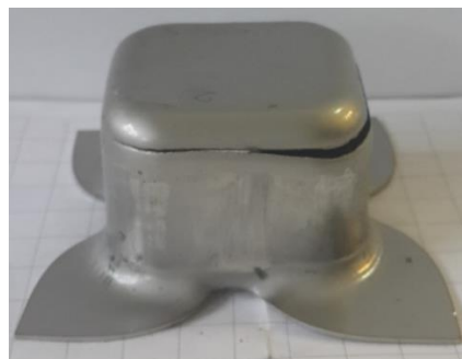
Figure 7.16. The fractured part in the square cup drawing of DKP6112 material
