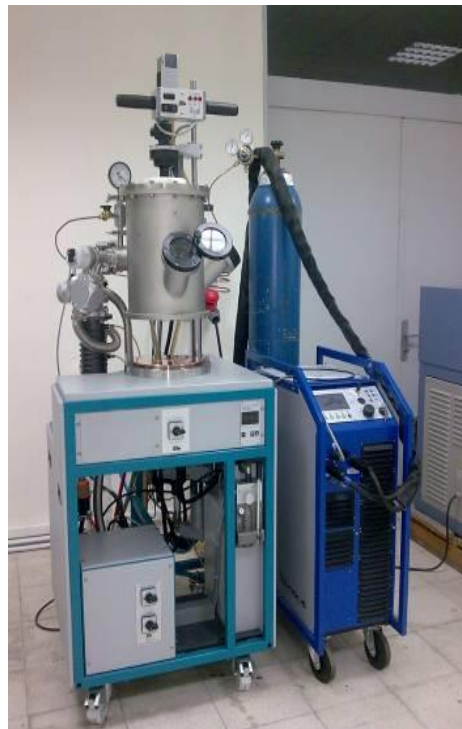
Figure 3.1 The arc-melter used for fabrication of samples.
