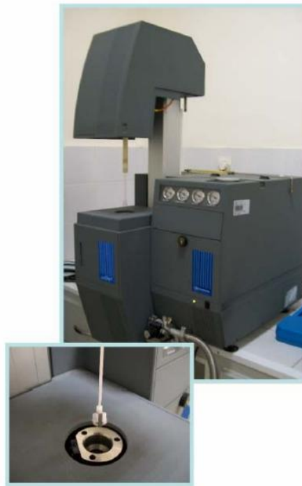
Figure 3.3 Setaram Setsys–16/18 DSC used in the thermal analysis measurements.
