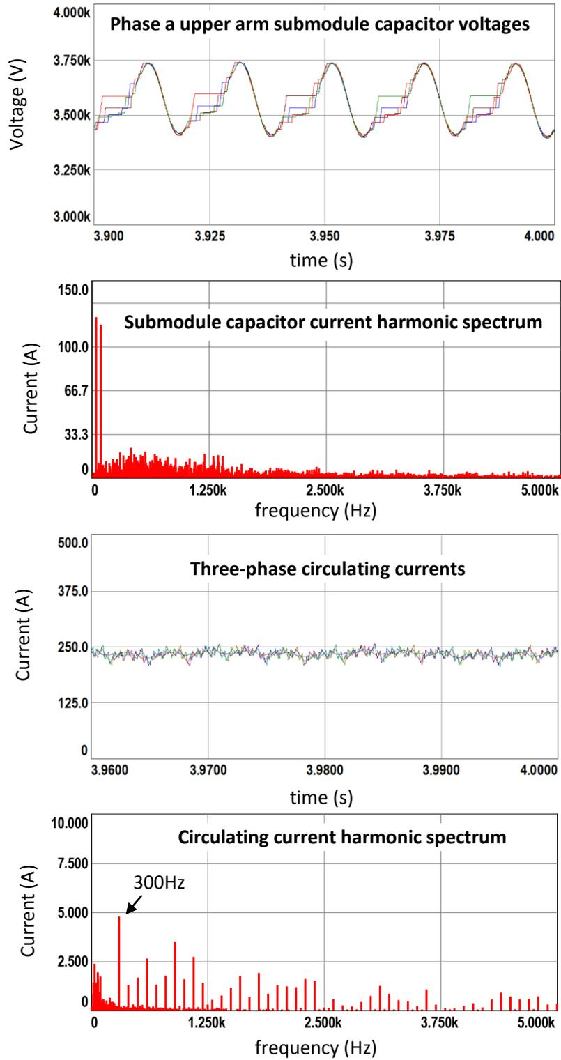
Figure 7.2 (continued) Simulation results for S&S method with N+1 level  $V_{ph}$ , full load
