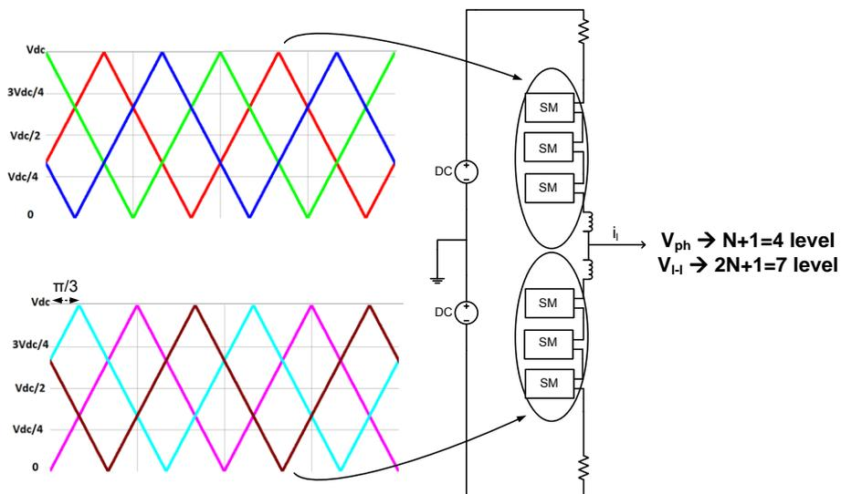
Figure 4.12 Carrier sets for N+1 level phase voltage of phase-shift method with odd number of submodules
