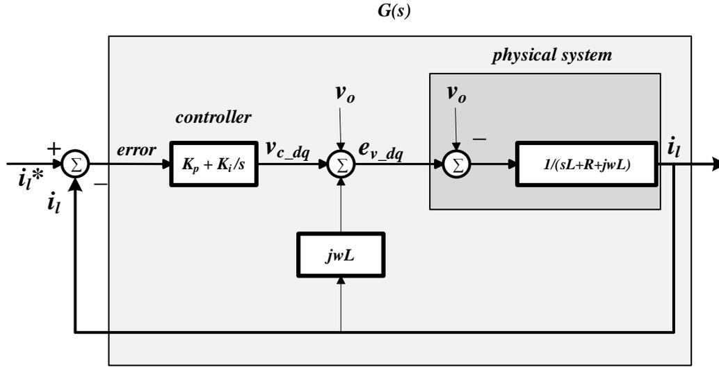
Figure 6.5 Feed forward of output dq current coupling term and output voltage of the converter
