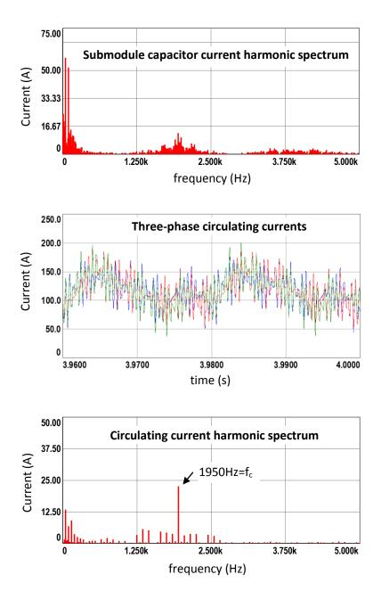
Figure 7.16 (continued) Simulation results for CR method with 2N+1 level  $V_{\text{ph}},$  half load
