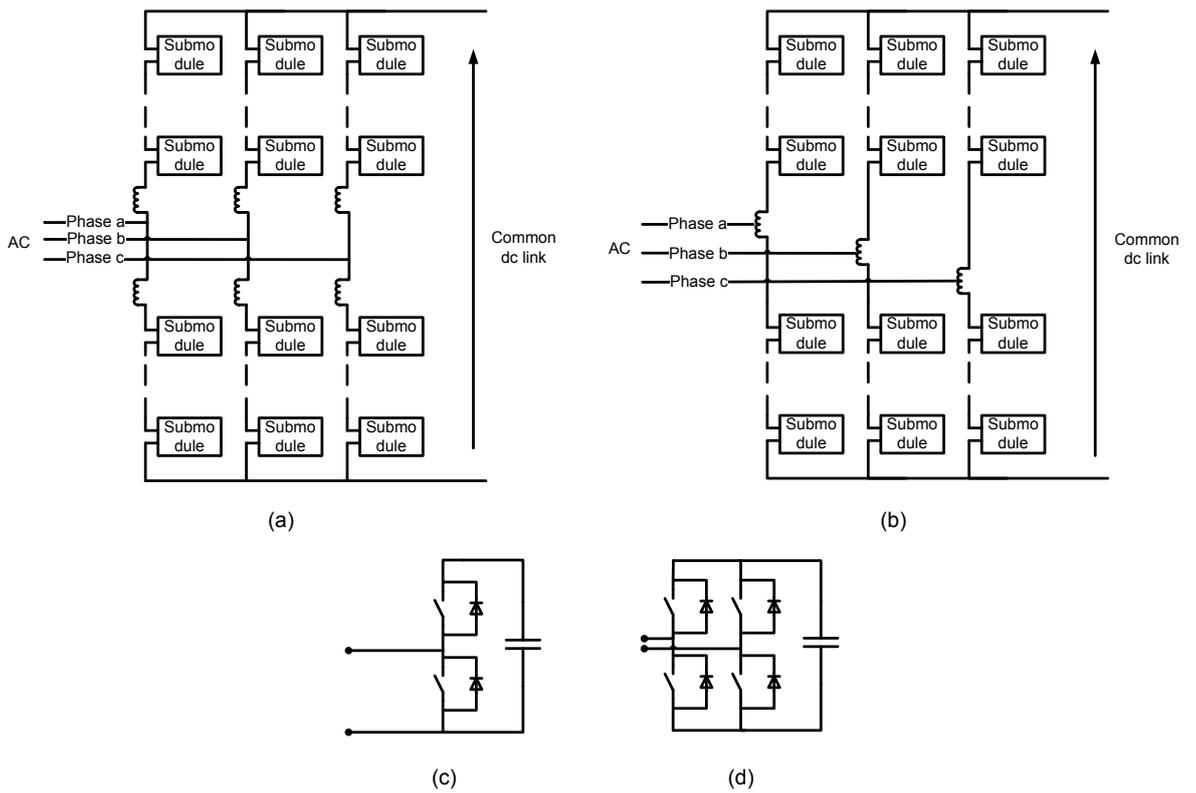
Figure 2.4 Possible circuit configurations of DSCC and DSBC (a) Power circuit using coupled arm inductors (b) Power circuit using non-coupled arm inductors (c) Chopper cell (DSCC) (d) Bridge cell (DSBC)
