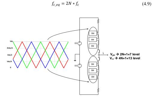
Figure 4.17 Carrier sets for 2N+1 level phase voltage of phase-shift method with odd number of submodules
