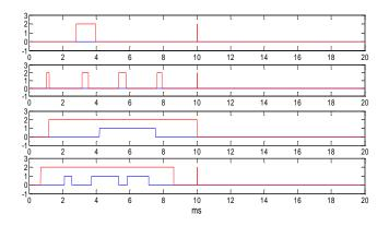
Figure 4.24 Switching pulse patterns of APOD for (ma=0.1, mf=3), (ma=0.1, mf=9), (ma=0.9, mf=3) and (ma=0.9, mf=9) from the top to the bottom
