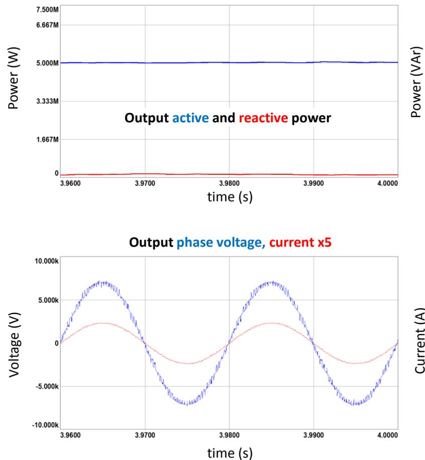
Figure 7.17 Simulation results for PSCB method with  $2N+1$  level  $V_{ph}$ , half load
