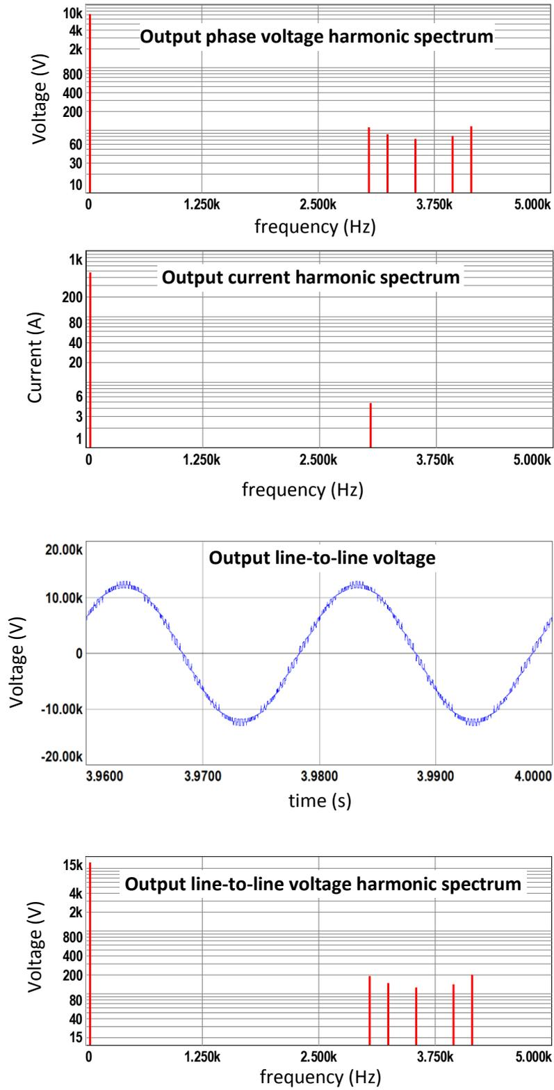
Figure 7.15 (continued) Simulation results for S&S-RS method with  $2N+1$  level  $V_{ph}$ , half load
