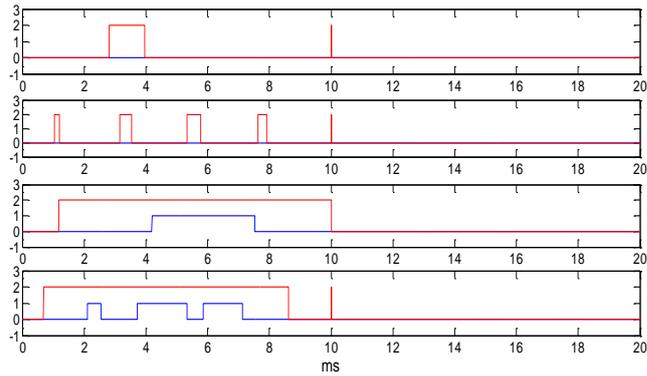
Figure 4.24 Switching pulse patterns of APDOD for  $(m_a=0.1, m_f=3)$ ,  $(m_a=0.1, m_f=9)$ ,  $(m_a=0.9, m_f=3)$  and  $(m_a=0.9, m_f=9)$  from the top to the bottom
