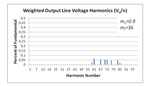
Figure 4.47 Weighted line voltage harmonics of POD for 2N+1 level V<sub>ph</sub>
