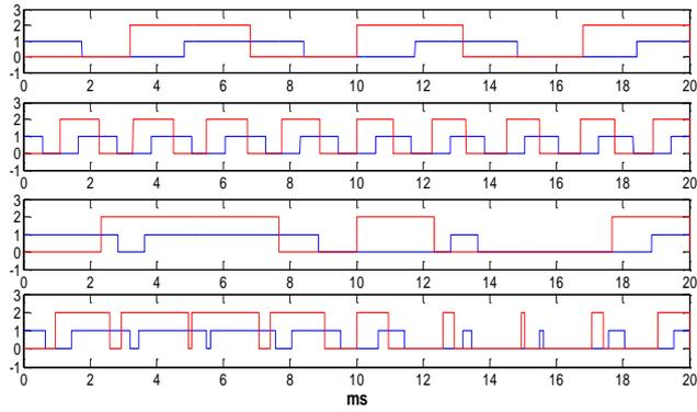
Figure 4.21 Switching pulse patterns of PS for  $(ma=0.1, mf=3)$ ,  $(ma=0.1, mf=9)$ ,  $(ma=0.9, mf=3)$  and  $(ma=0.9, mf=9)$  from the top to the bottom
