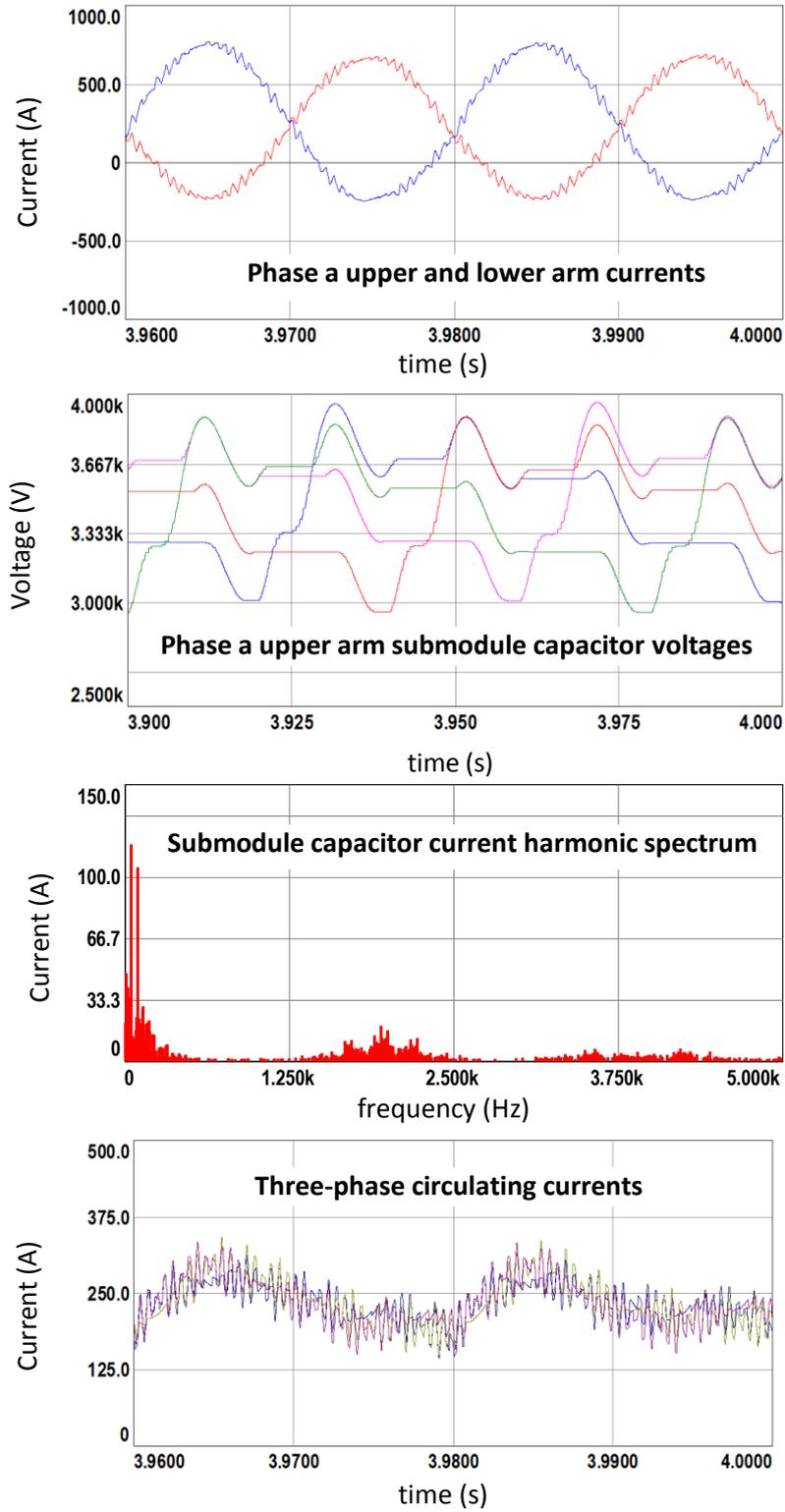
Figure 7.8 (continued) Simulation results for CR method with  $2N+1$  level  $V_{ph}$ , full load
