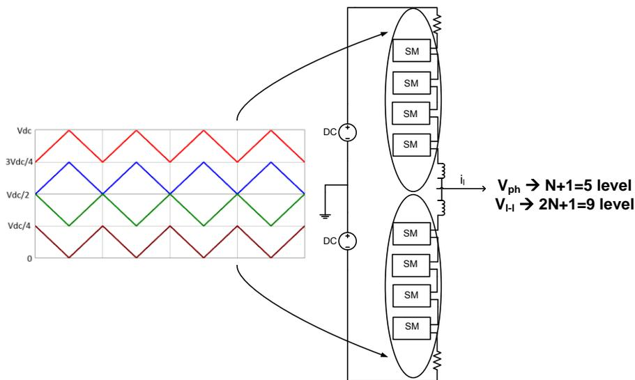
Figure 4.10 Carrier set for N+1 level phase voltage of POD method
