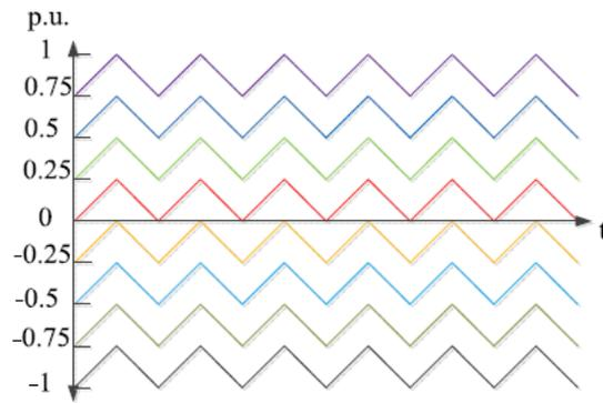
Figure 4.2 Phase disposition (PD) method
