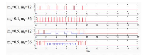
Figure 4.28 Switching pulse patterns of APOD
