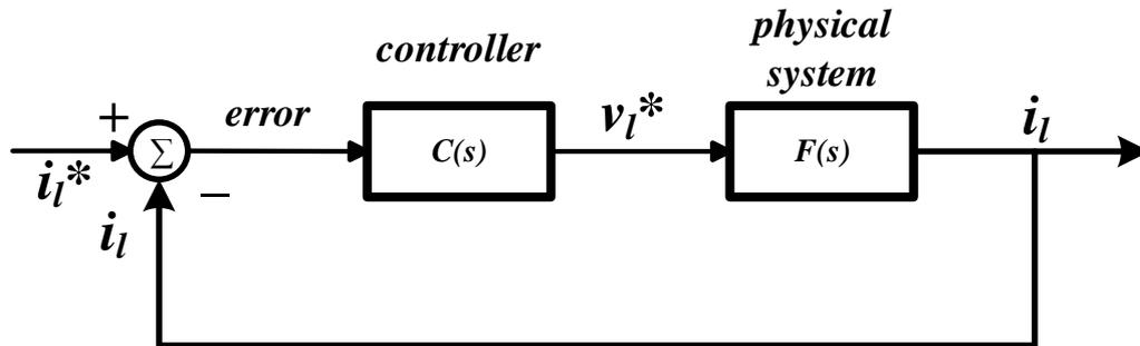
Figure 6.2 Overview of the output current PI controller and physical system
