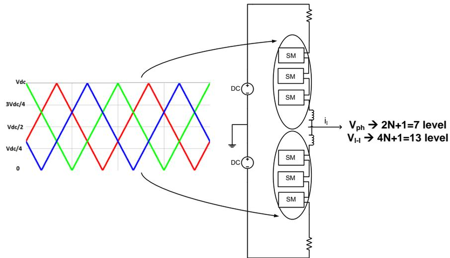
Figure 4.17 Carrier sets for  $2N+1$  level phase voltage of phase-shift method with odd number of submodules
