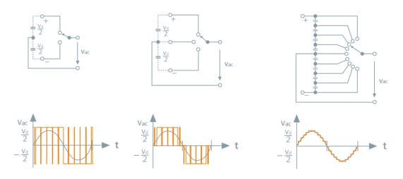
Figure 1.2 Output voltage synthesis concepts of two, three and multilevel converters [4]
