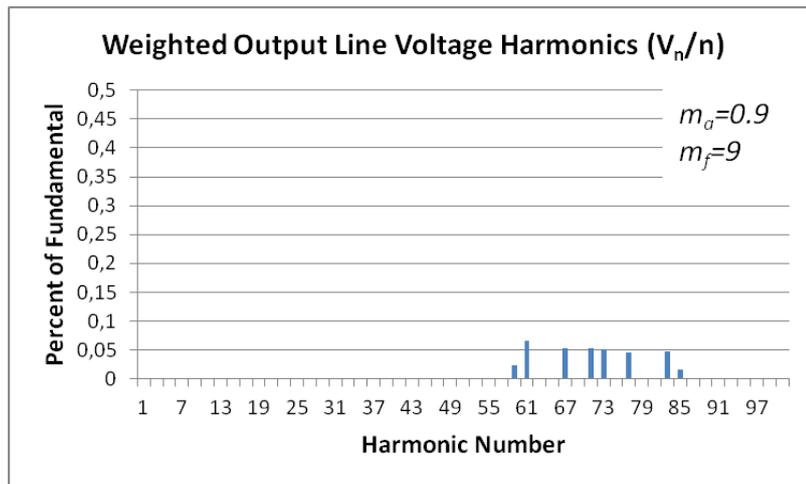
Figure 4.45 Weighted line voltage harmonics of PS for  $2N+1$  level  $V_{ph}$
