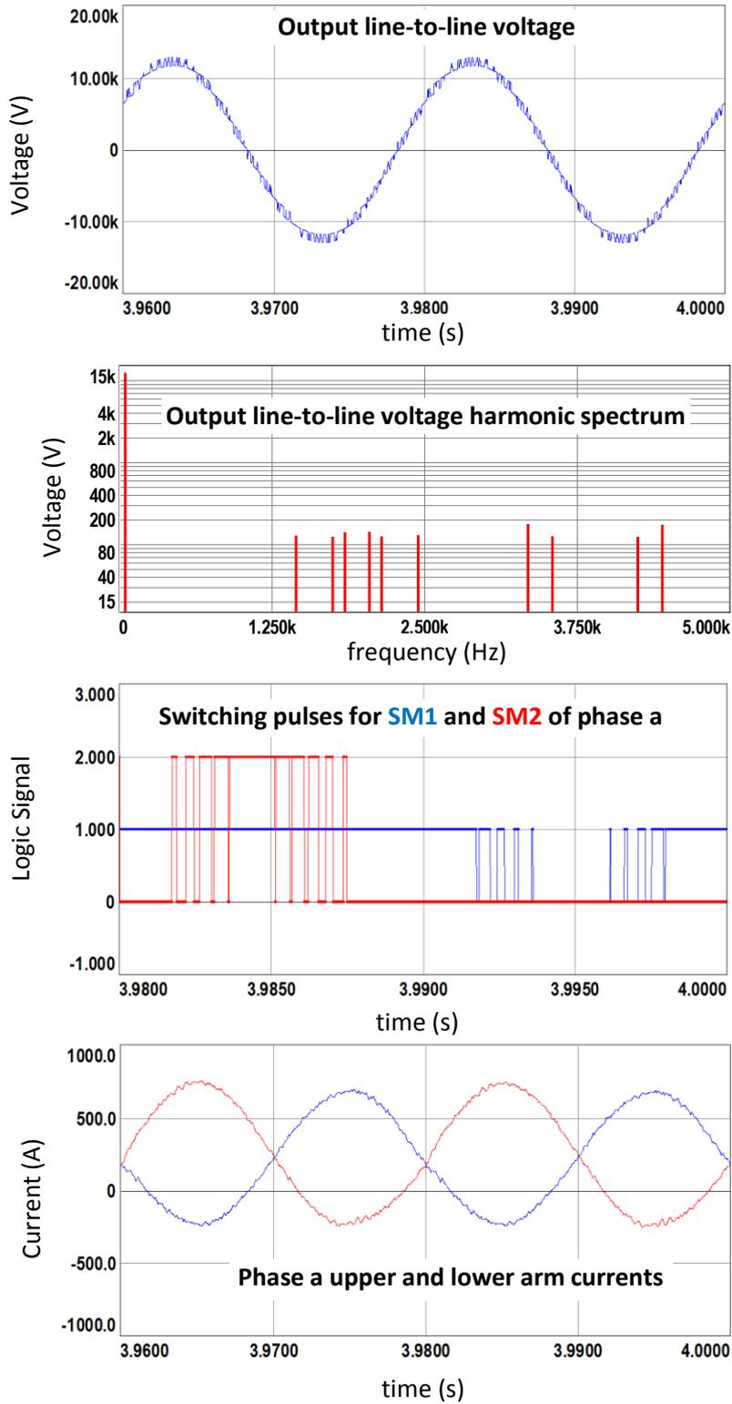
Figure 7.4 (continued) Simulation results for CR method with  $N+1$  level  $V_{ph}$ , full load
