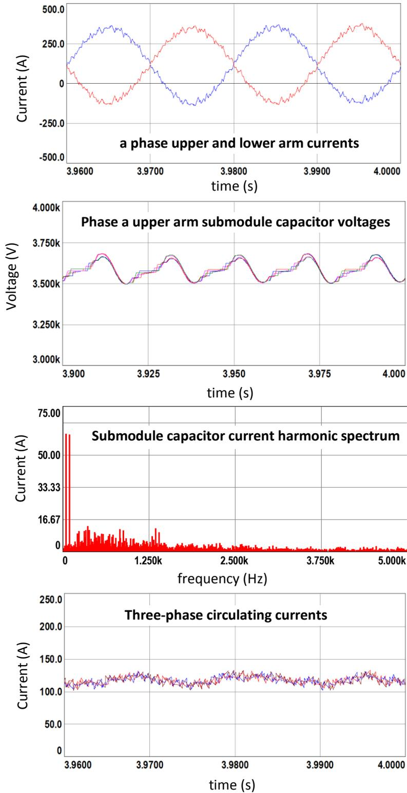
Figure 7.10 (continued) Simulation results for S&S method with N+1 level  $V_{ph}$ , half load
