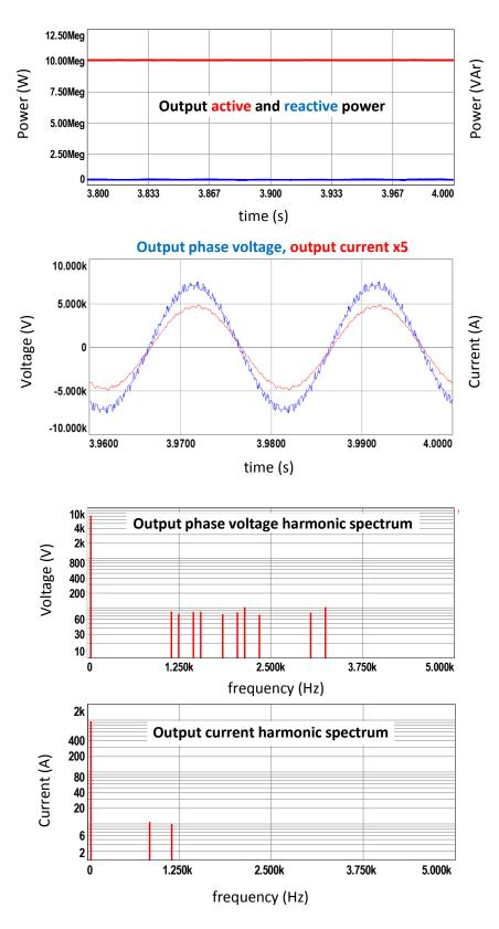
Figure 7.2 Simulation results for S&S method with N+1 level  $V_{\text{ph}}\text{, full load}$
