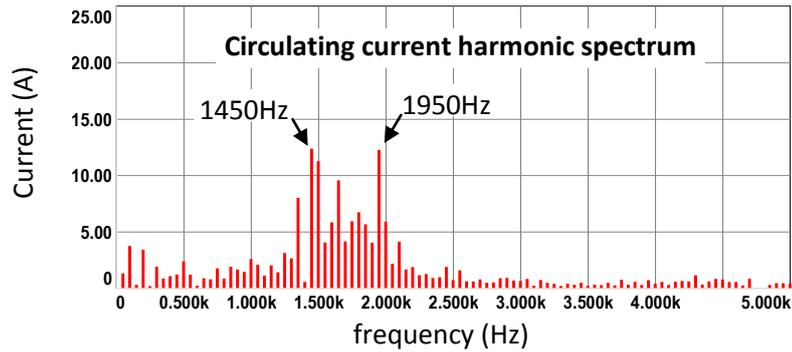
Figure 7.9 (continued) Simulation results for PSCB method with  $2N+1$  level  $V_{ph}$ , full load
