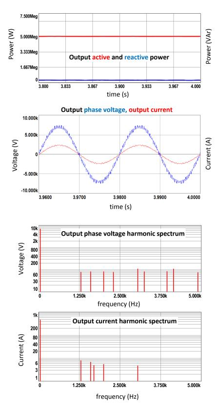
Figure 7.11 Simulation results for S&S-RS method with N+1 level  $V_{\text{ph}}\text{, half load}$
