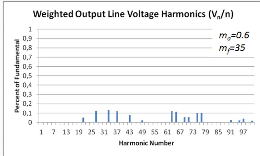
Figure 4.38 Weighted line voltage harmonics of PD for N+1 level  $V_{ph}$
