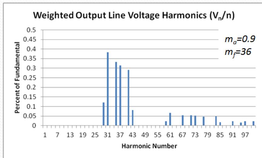
Figure 4.36 Weighted line voltage harmonics of APOD for N+1 level  $V_{ph}$
