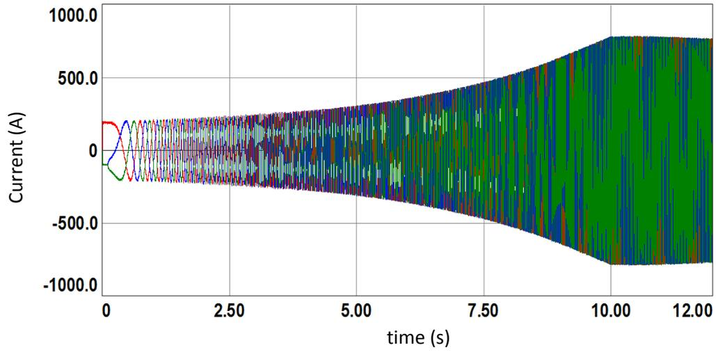
Figure 8.5 Three-phase stator currents of the induction machine
