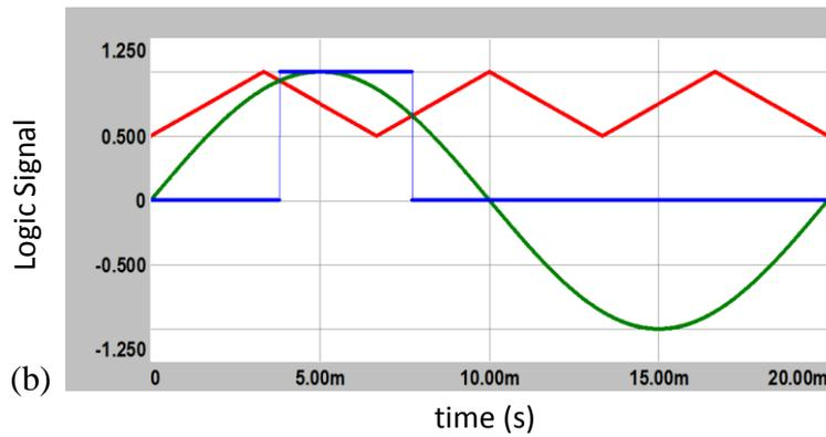
Figure 4.20 Carrier, reference and switching pulse signals for (a) PS and (b) PD methods for  $m_a=1$  and  $m_f=3$
