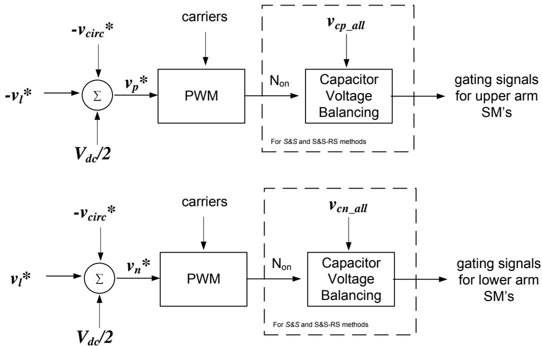
Figure 6.13 Block diagram for generation of reference signals and the remaining process for obtaining gate signals of submodules
