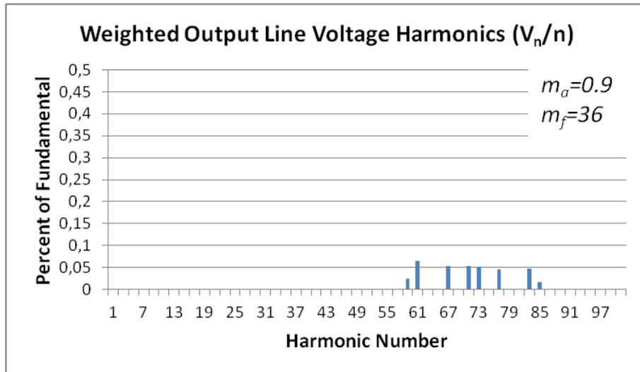
Figure 4.47 Weighted line voltage harmonics of POD for  $2N+1$  level  $V_{ph}$
