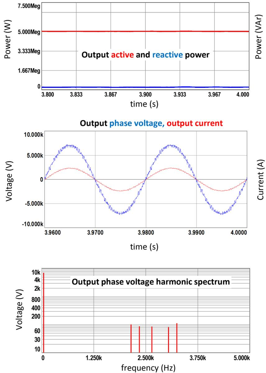
Figure 7.14 Simulation results for S&S method with  $2N+1$  level  $V_{ph}$ , half load
