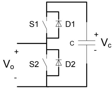
Figure 2.8 Half-bridge (chopper) circuit
