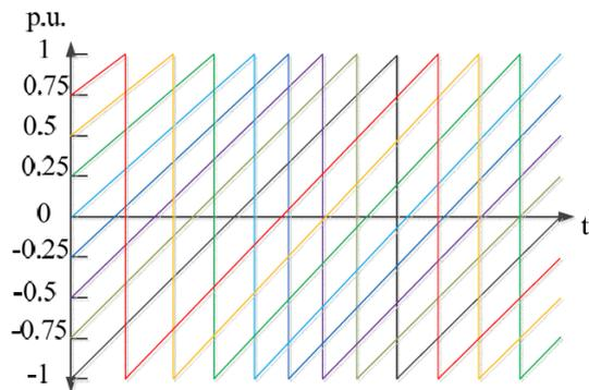
Figure 4.6 Sawtooth rotation method
