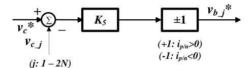
Figure 6.16 Balancing control of PSCB control
