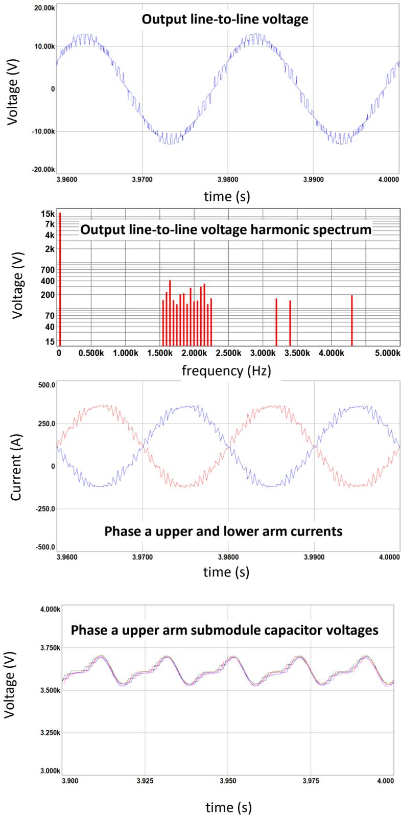
Figure 7.13 (continued) Simulation results for PSCB method with  $N+1$  level  $V_{ph}$ , half load
