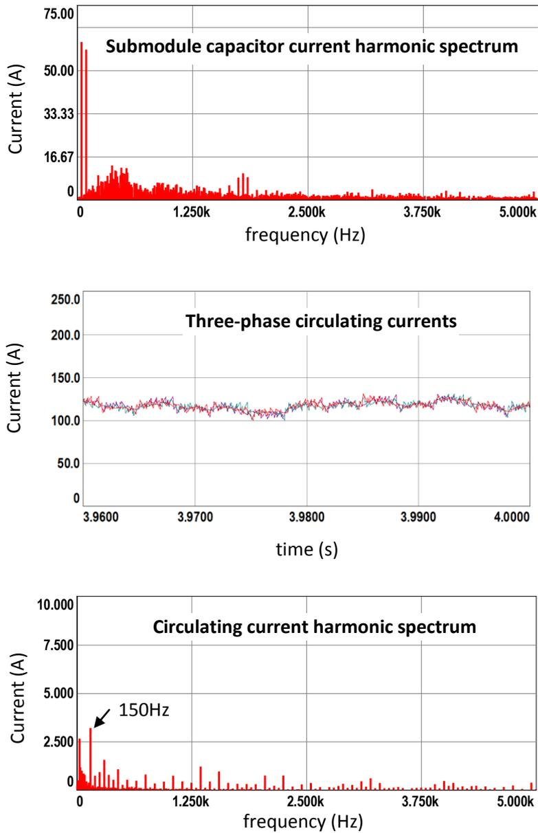
Figure 7.11 (continued) Simulation results for S&S-RS method with N+1 level  $V_{ph}$ , half load
