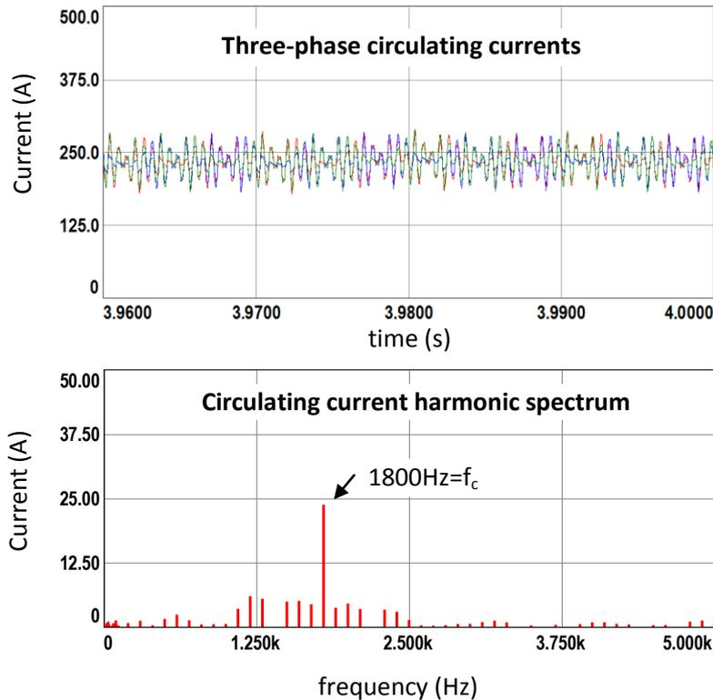
Figure 7.7 (continued) Simulation results for S&S-RS method with  $2N+1$  level  $V_{ph}$ , full load
