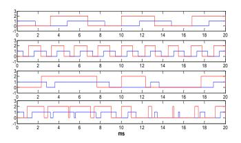
Figure 4.21 Switching pulse patterns of PS for (ma=0.1, mf=3), (ma=0.1, mf=9), (ma=0.9, mf=3) and (ma=0.9, mf=9) from the top to the bottom
