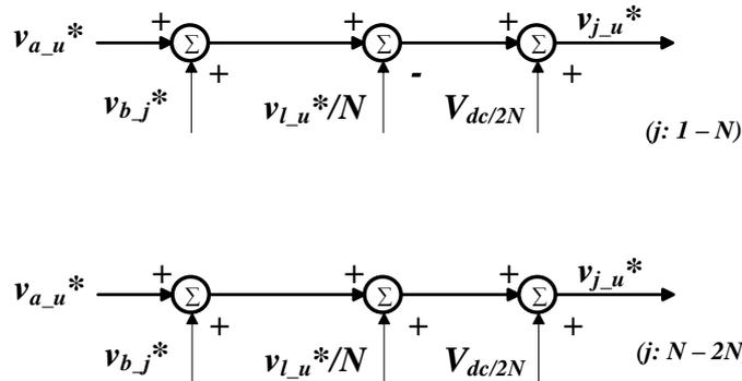
Figure 6.17 Reference signal generation for upper and lower arm submodules
