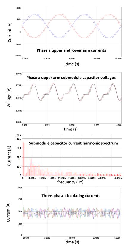
Figure 7.9 (continued) Simulation results for PSCB method with 2N+1 level  $V_{\text{ph}}, \\ full load$
