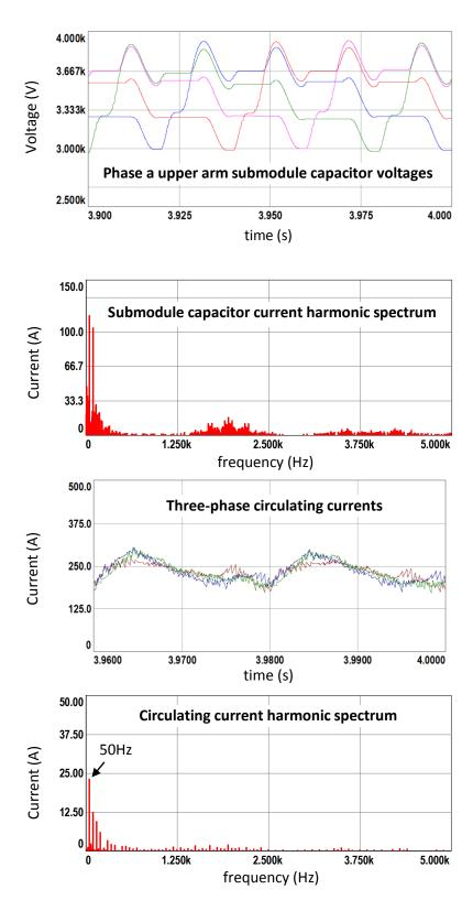
Figure 7.4 (continued) Simulation results for CR method with N+1 level  $V_{\text{ph}}\text{, full load}$
