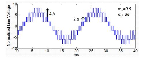
Figure 4.31 Normalized line voltage of POD for N+1 level  $V_{ph}$
