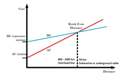
Figure 1.3 Cost estimations for ac and HVDC transmission by distance [3]
