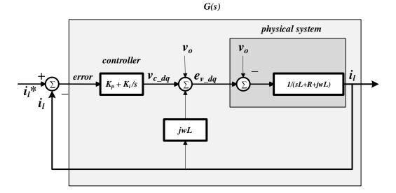
Figure 6.5 Feed forward of output dq current coupling term and output voltage of the converter
