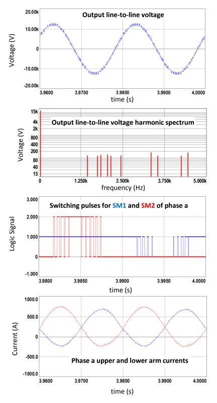
Figure 7.4 (continued) Simulation results for CR method with N+1 level  $V_{\text{ph}}\text{, full load}$
