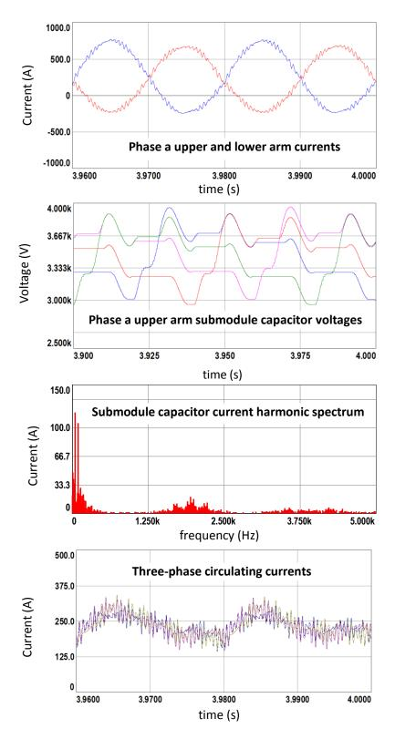
Figure 7.8 (continued) Simulation results for CR method with 2N+1 level  $V_{\text{ph}}\text{, full load}$
