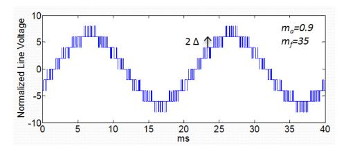
Figure 4.30 Normalized line voltage of PD for N+1 level  $V_{ph}$
