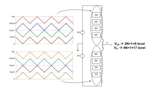
Figure 4.15 Carrier sets for 2N+1 level phase voltage of POD method
