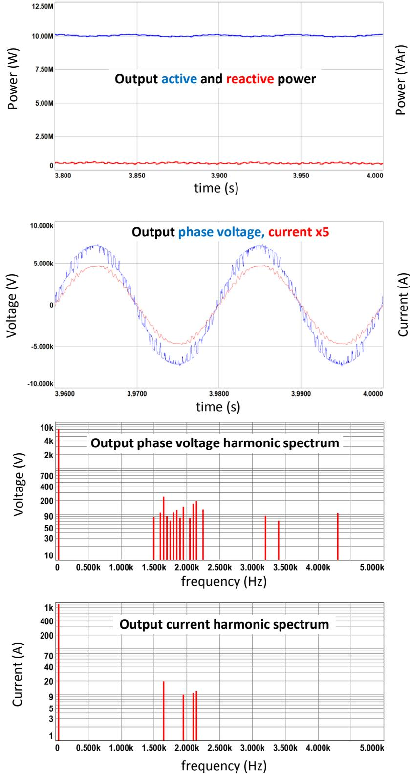
Figure 7.5 Simulation results for PSCB method with N+1 level  $V_{ph}$ , full load
