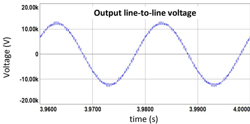
Figure 7.7 (continued) Simulation results for S&S-RS method with  $2N+1$  level  $V_{ph}$ , full load
