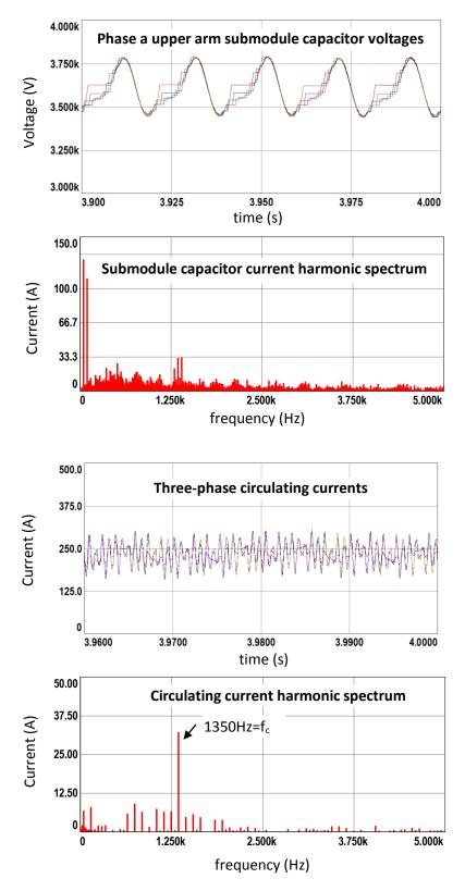
Figure 7.6 (continued) Simulation results for S&S method with 2N+1 level  $V_{\text{ph}}\text{, full load}$
