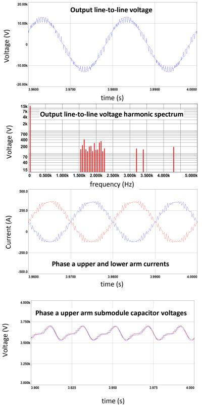
Figure 7.13 (continued) Simulation results for PSCB method with N+1 level  $V_{\text{ph}}, \\ half load$
