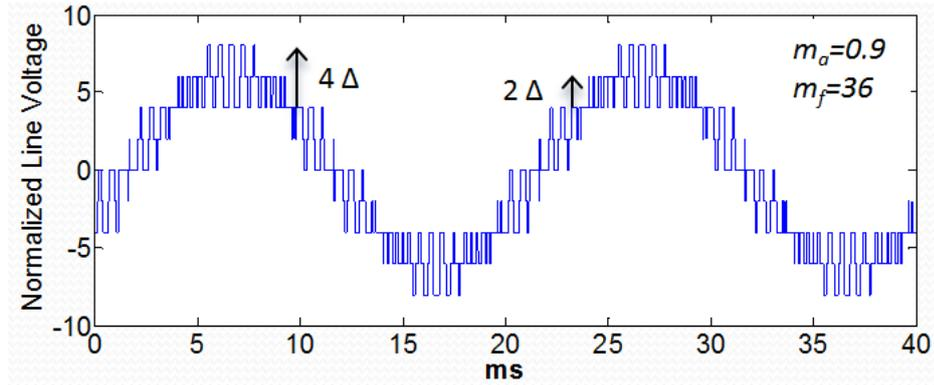
Figure 4.32 Normalized line voltage of APOD for N+1 level  $V_{ph}$
