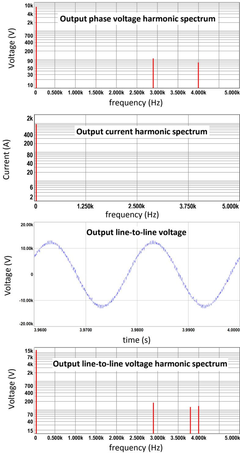
Figure 7.9 (continued) Simulation results for PSCB method with  $2N+1$  level  $V_{ph}$ , full load
