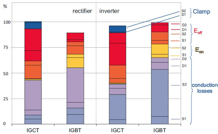
Figure 2.13 Normalized semiconductor losses at the top and semiconductor losses of a MMC submodule splitted in its components for  $P=850\text{MW}$ ,  $Q=350\text{MVar}$ ,  $f_{\text{switch}}=150\text{Hz}$ ,  $V_{\text{dc}} = 600\text{kV}$  at the bottom [40]
