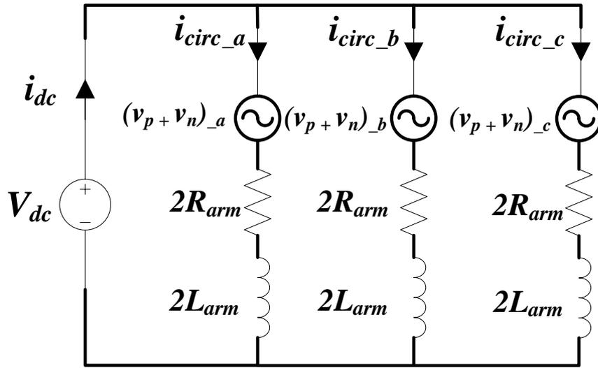
Figure 6.11 Circulating current equivalent circuit of MMC
