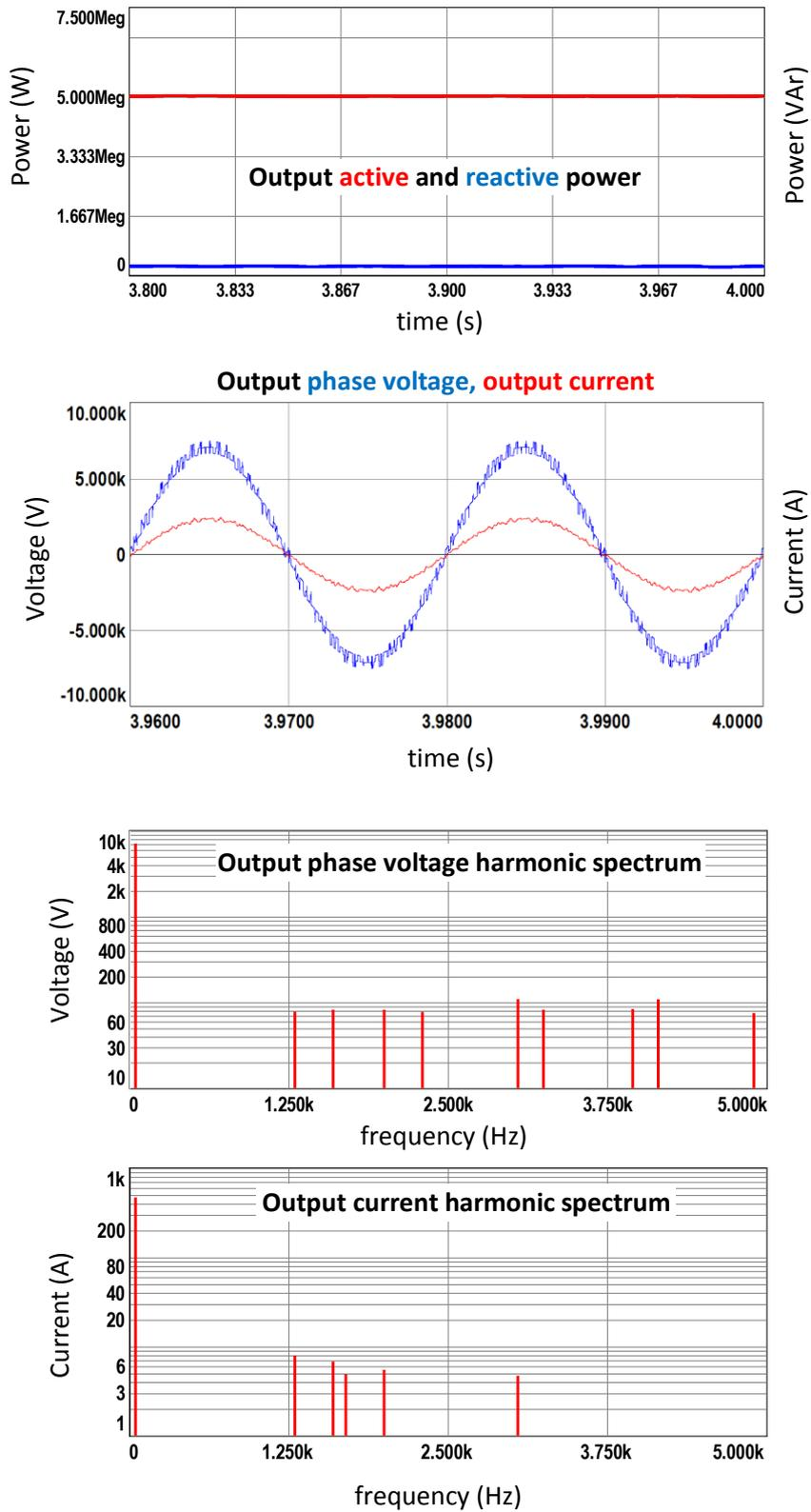
Figure 7.11 Simulation results for S&S-RS method with N+1 level  $V_{ph}$ , half load
