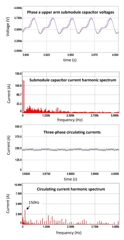
Figure 7.3 (continued) Simulation results for S&S-RS method with N+1 level  $V_{\text{ph}}, \\ full \ \text{load}$
