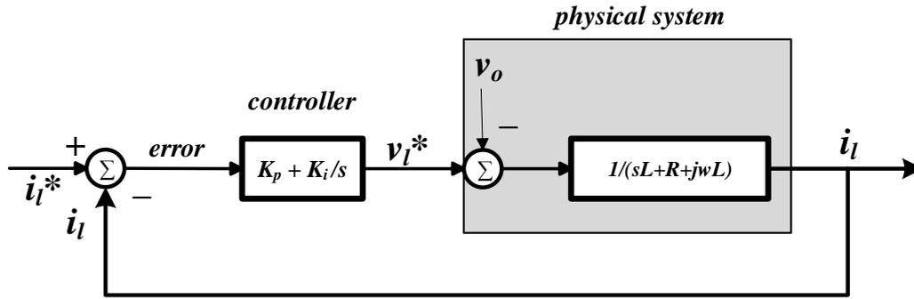
Figure 6.4 Overview of the output current PI controller and physical system with output voltage
