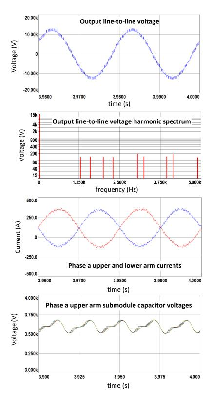
Figure 7.11 (continued) Simulation results for S&S-RS method with N+1 level  $V_{\text{ph}}, \\ half load$
