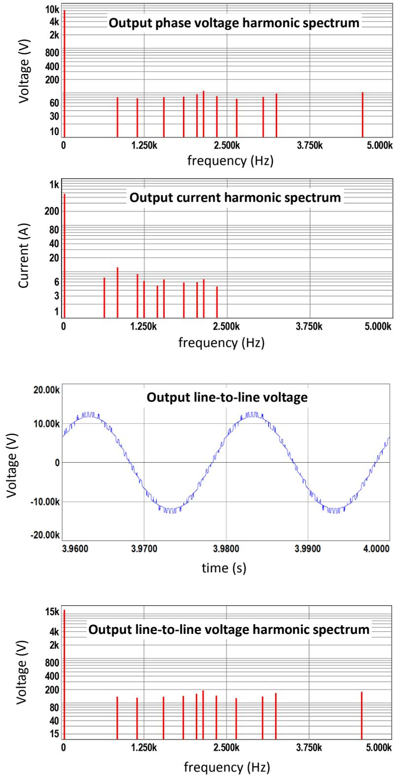
Figure 7.10 (continued) Simulation results for S&S method with N+1 level  $V_{ph}$ , half load
