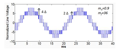
Figure 4.32 Normalized line voltage of APOD for N+1 level V<sub>ph</sub>
