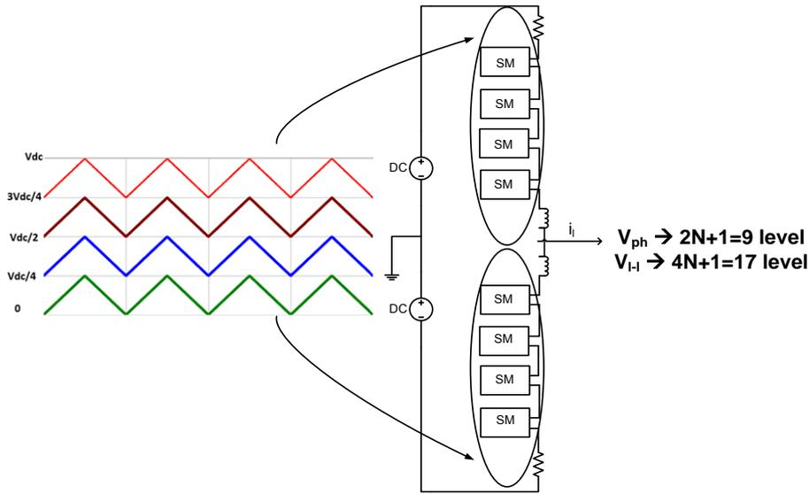
Figure 4.14 Carrier set for  $2N+1$  level phase voltage of PD method
