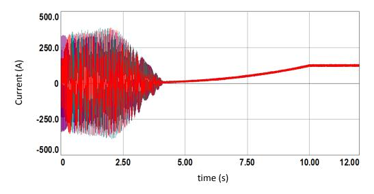
Figure 8.8 Three-phase circulating currents of MMC motor drive
