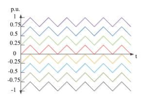
Figure 4.2 Phase disposition (PD) method
