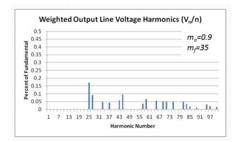
Figure 4.34 Weighted line voltage harmonics of PD for N+1 level V<sub>ph</sub>
