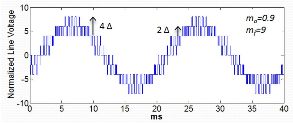
Figure 4.29 Normalized line voltage of PS for N+1 level  $V_{ph}$
