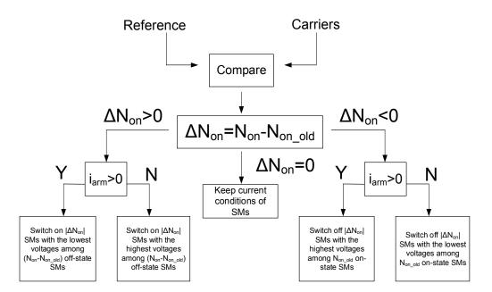
Figure 6.9 Determination of inserted or bypassed submodules for sort and select method with reduced number of switching
