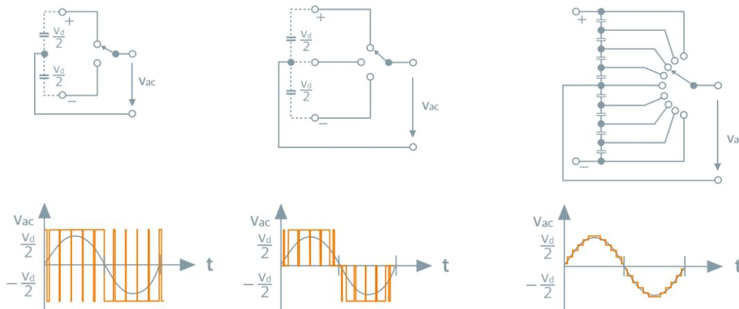
Figure 1.2 Output voltage synthesis concepts of two, three and multilevel converters [4]
