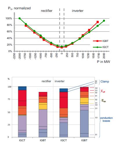
Figure 2.13 Normalized semiconductor losses at the top and semiconductor losses of a MMC submodule splitted in its components for P=850MW, Q=350MVar,  $f_{switch}$ =150Hz,  $V_{dc}$  = 600kV at the bottom [40]
