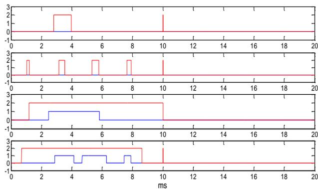
Figure 4.23 Switching pulse patterns of POD for  $(ma=0.1, mf=3)$ ,  $(ma=0.1, mf=9)$ ,  $(ma=0.9, mf=3)$  and  $(ma=0.9, mf=9)$  from the top to the bottom
