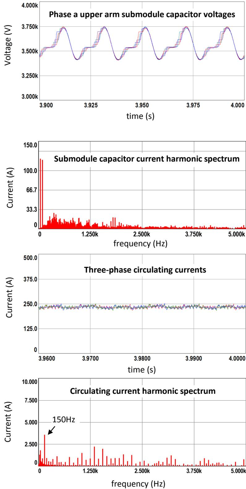
Figure 7.3 (continued) Simulation results for S&S-RS method with N+1 level  $V_{ph}$ , full load
