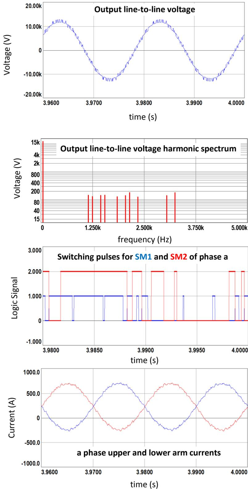
Figure 7.2 (continued) Simulation results for S&S method with N+1 level  $V_{ph}$ , full load
