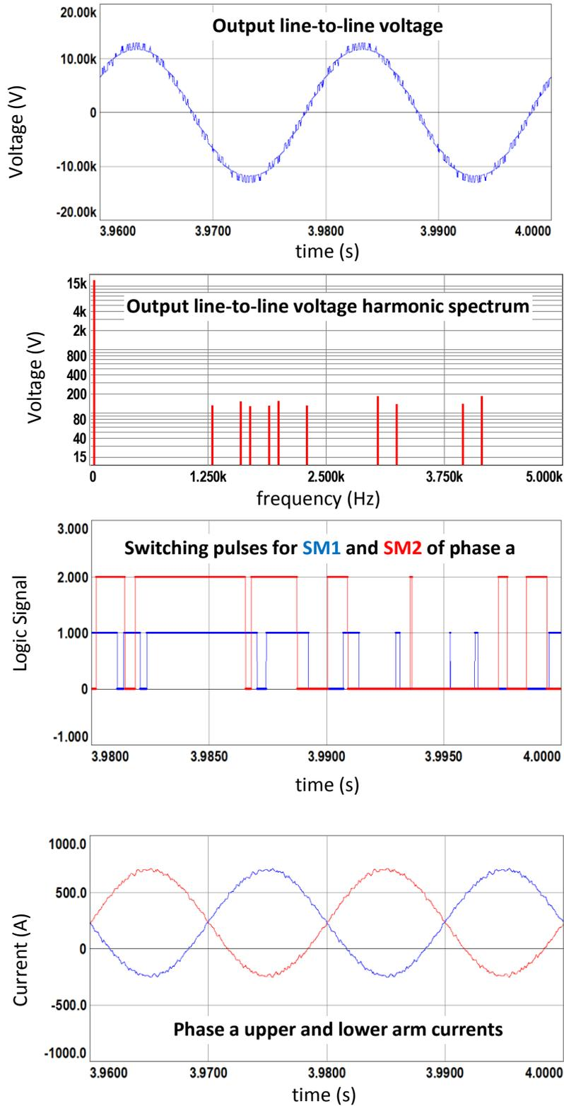
Figure 7.3 (continued) Simulation results for S&S-RS method with N+1 level  $V_{ph}$ , full load
