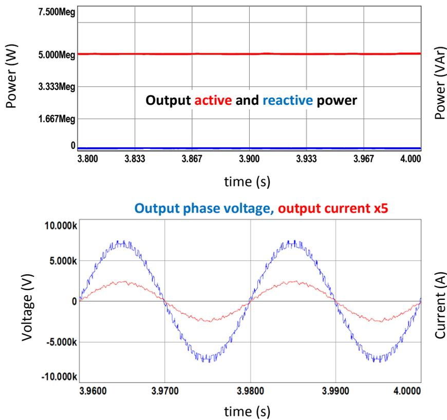
Figure 7.10 Simulation results for S&S method with N+1 level  $V_{ph}$ , half load
