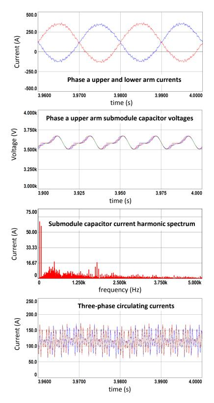
Figure 7.15 (continued) Simulation results for S&S-RS method with 2N+1 level  $V_{\text{ph}}, \\ \text{half load}$
