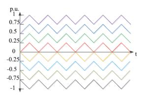
Figure 4.3 Phase opposition disposition (POD) method
