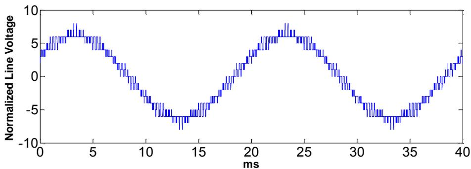
Figure 4.41 Normalized line voltage of PS for  $2N+1$  level  $V_{ph}$
