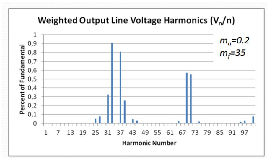
Figure 4.37 Weighted line voltage harmonics of PD for N+1 level  $V_{ph}$
