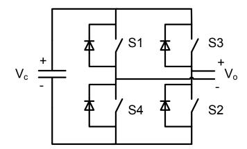
Figure 2.5 The full-bridge circuit topology
