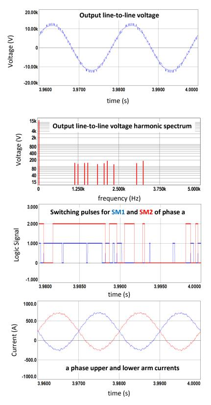
Figure 7.2 (continued) Simulation results for S&S method with N+1 level  $V_{\text{ph}}\text{, full load}$
