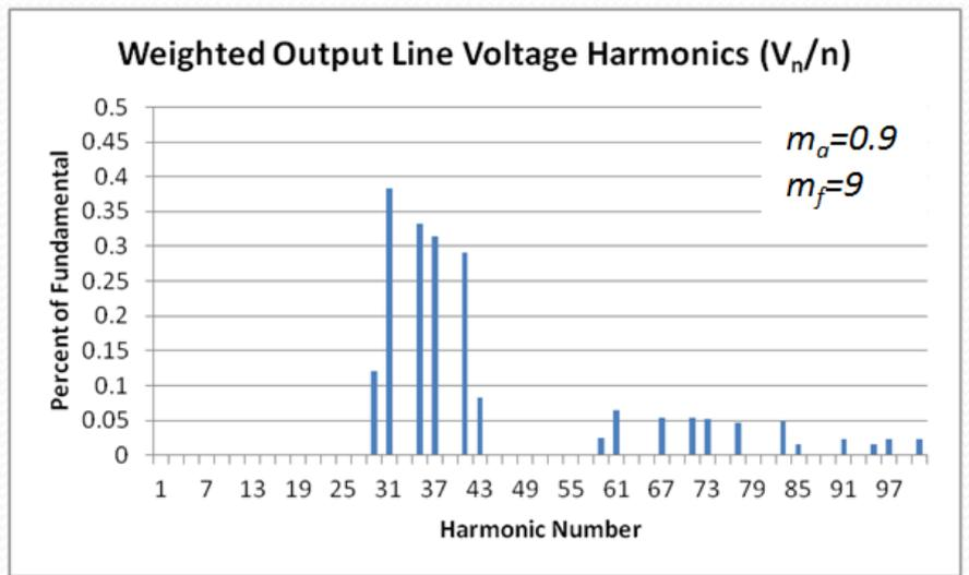
Figure 4.33 Weighted line voltage harmonics of PS for N+1 level  $V_{ph}$
