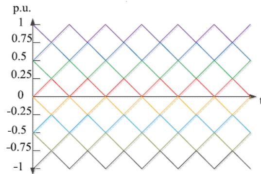
Figure 4.4 Alternative phase opposition disposition (APOD) method
