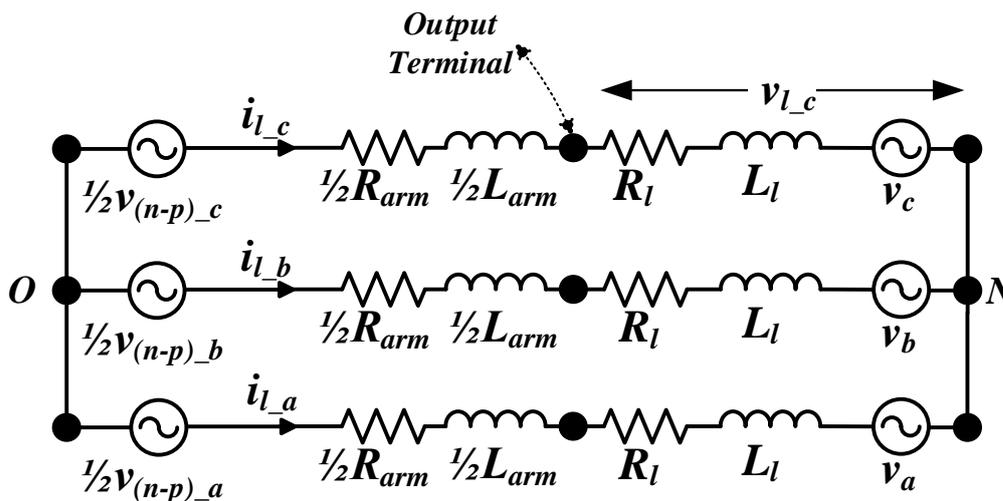
Figure 6.3 Equivalent circuit of MMC in terms of output currents
