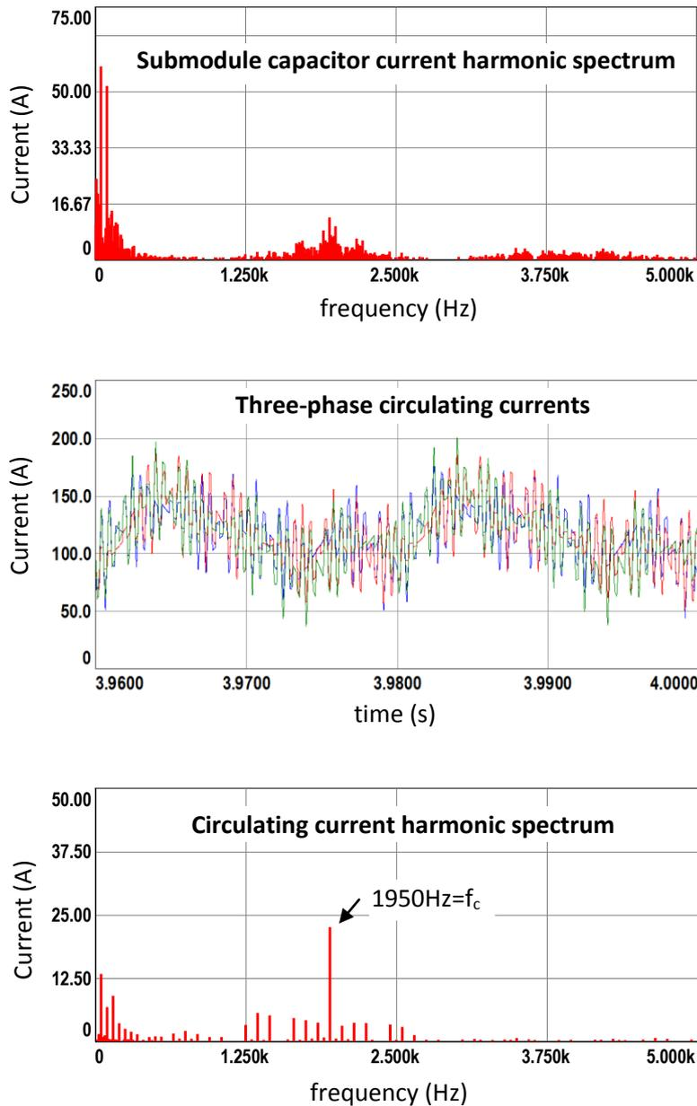
Figure 7.16 (continued) Simulation results for CR method with  $2N+1$  level  $V_{ph}$ , half load
