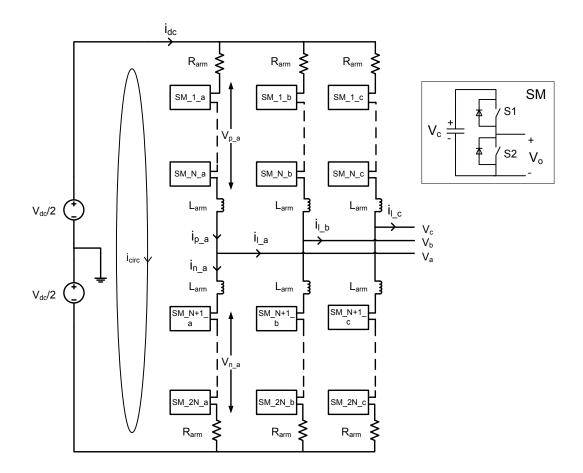
Figure 3.1 Circuit structure of MMC
