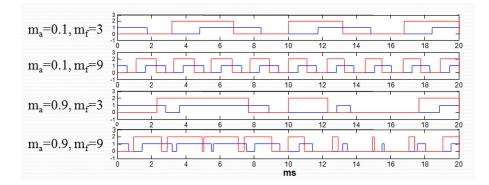
Figure 4.25 Switching pulse patterns of PS
