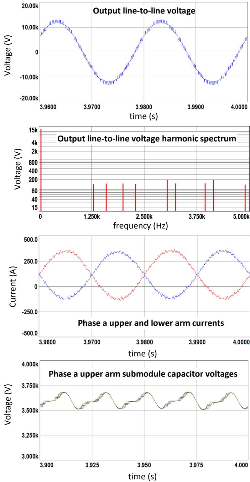
Figure 7.11 (continued) Simulation results for S&S-RS method with N+1 level  $V_{ph}$ , half load
