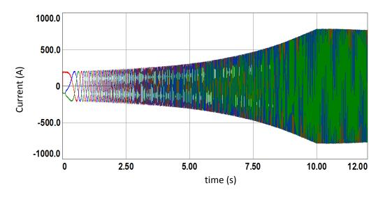
Figure 8.5 Three-phase stator currents of the induction machine
