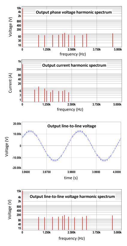
Figure 7.10 (continued) Simulation results for S&S method with N+1 level  $V_{\text{ph}},$  half load
