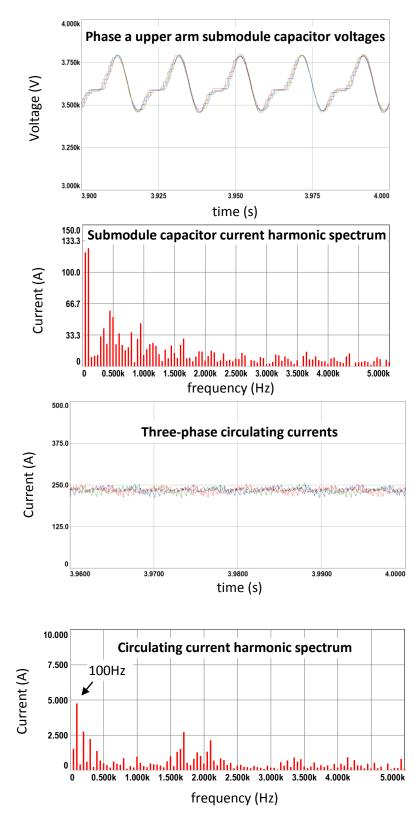
Figure 7.5 (continued) Simulation results for PSCB method with N+1 level  $V_{\mbox{\scriptsize ph}}$  , full load
