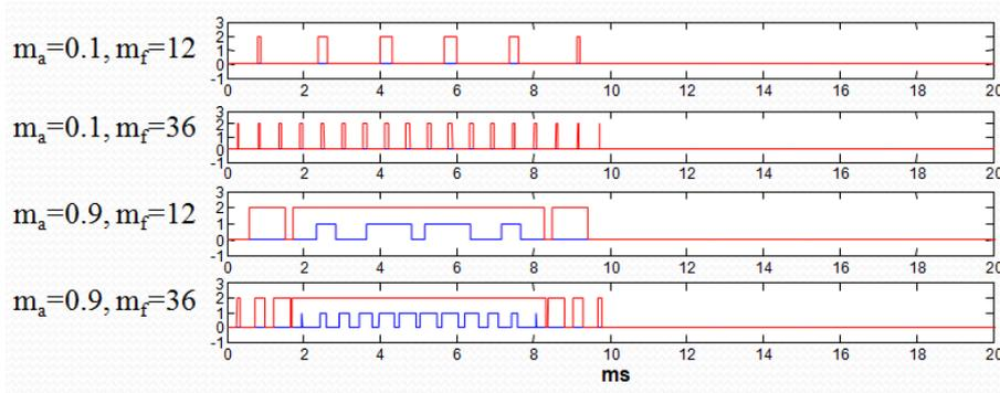
Figure 4.27 Switching pulse patterns of POD
