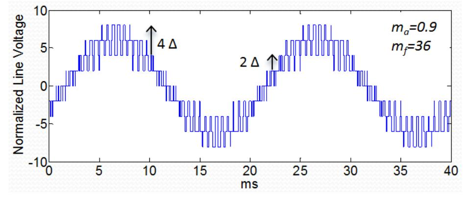
Figure 4.31 Normalized line voltage of POD for N+1 level  $V_{ph}$
