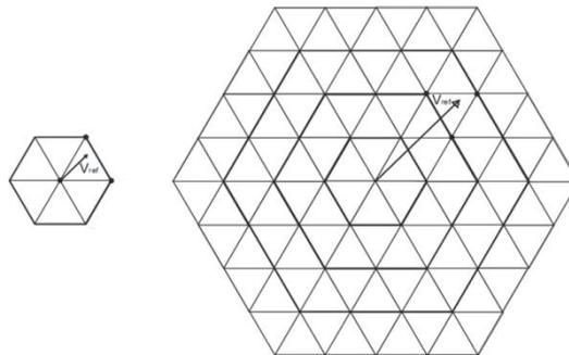
Figure 4.7 Space vector diagrams for two-level converter at left and five-level converter at right
