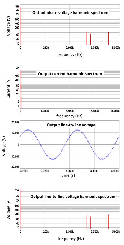
Figure 7.8 (continued) Simulation results for CR method with 2N+1 level  $V_{\text{ph}}\text{, full load}$
