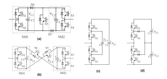
Figure 2.10 (a) The clamp double circuit (b) The five level cross connected circuit (c, d) capacitor-clamped and diode-clamped three-level converters [69]
