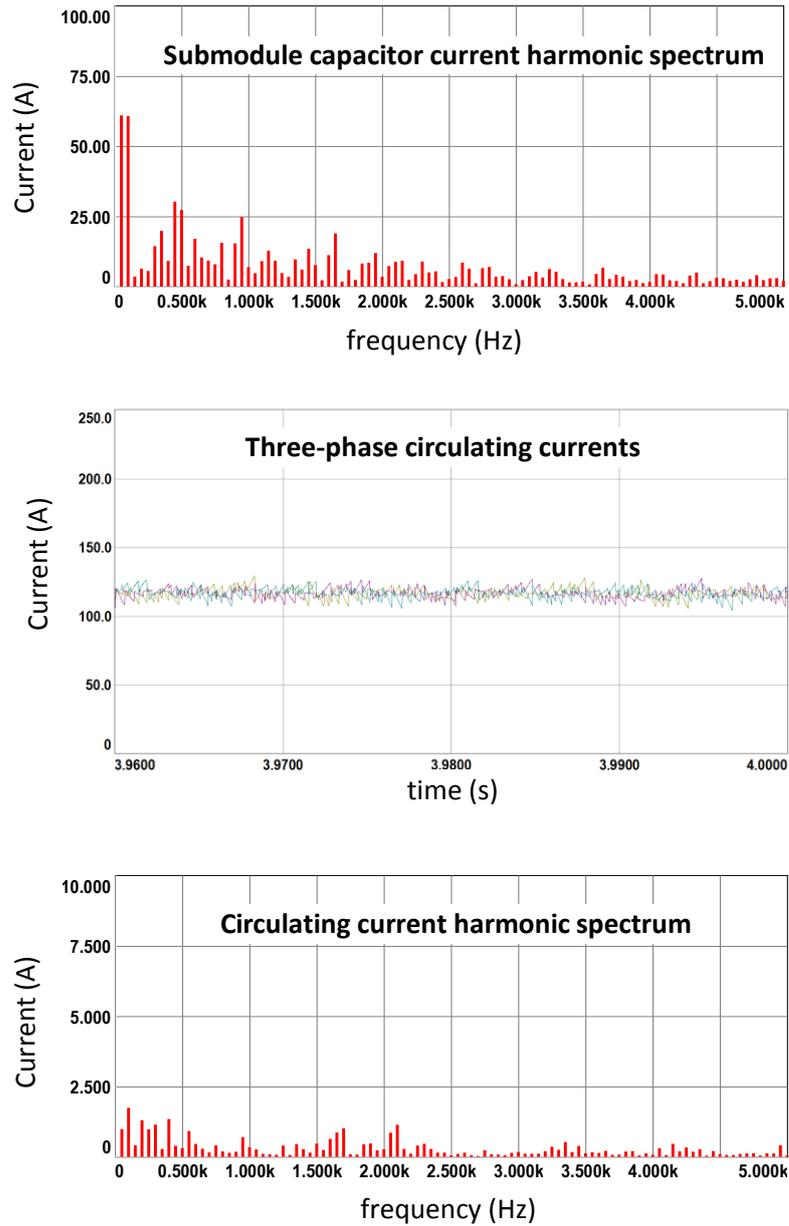
Figure 7.13 (continued) Simulation results for PSCB method with  $N+1$  level  $V_{ph}$ , half load
