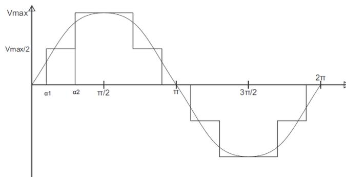
Figure 4.8 Output voltage waveform for a five-level converter, switching angles determined by selective harmonic elimination method
