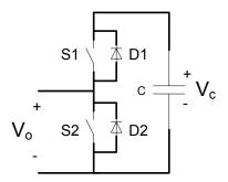
Figure 2.8 Half-bridge (chopper) circuit
