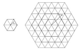
Figure 4.7 Space vector diagrams for two-level converter at left and five-level converter at right
