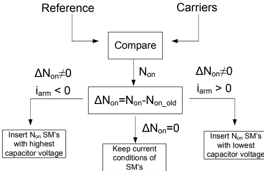
Figure 6.8 Determination of inserted submodules to the current path for sort and select method
