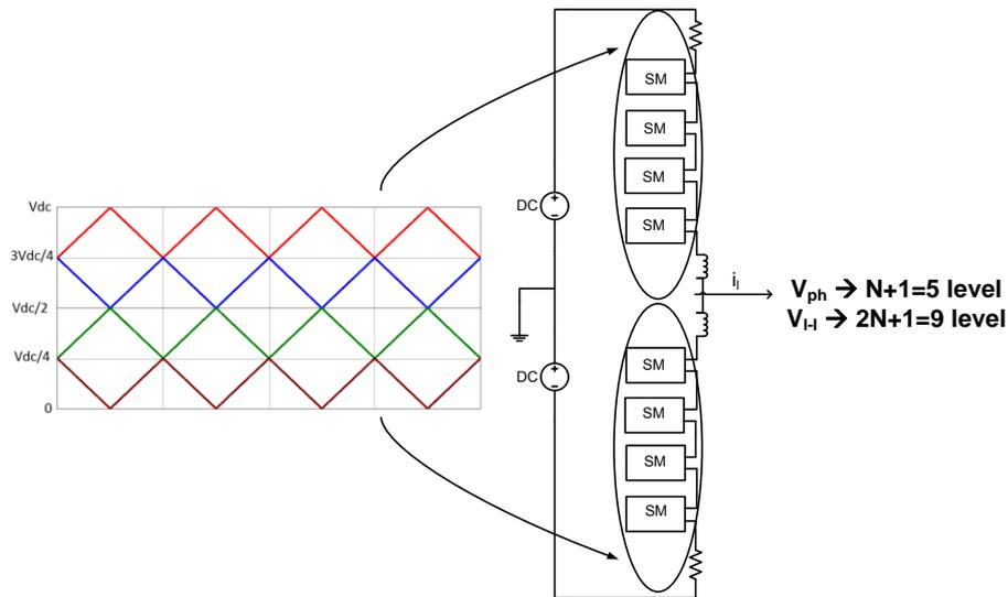
Figure 4.11 Carrier set for  $N+1$  level phase voltage of APOD method
