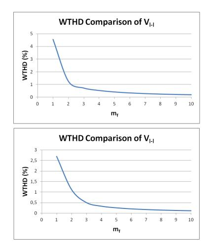
Figure 4.50 WTHD values for changing  $m_f$  and fixed  $m_a$ =0.6 and  $m_a$ =0.9 at the top and at the bottom, valid for all the LS and PS methods for 2N+1 level V<sub>ph</sub>
