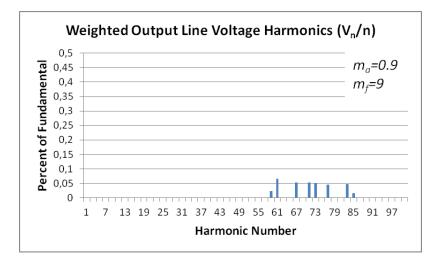
Figure 4.45 Weighted line voltage harmonics of PS for 2N+1 level V<sub>ph</sub>
