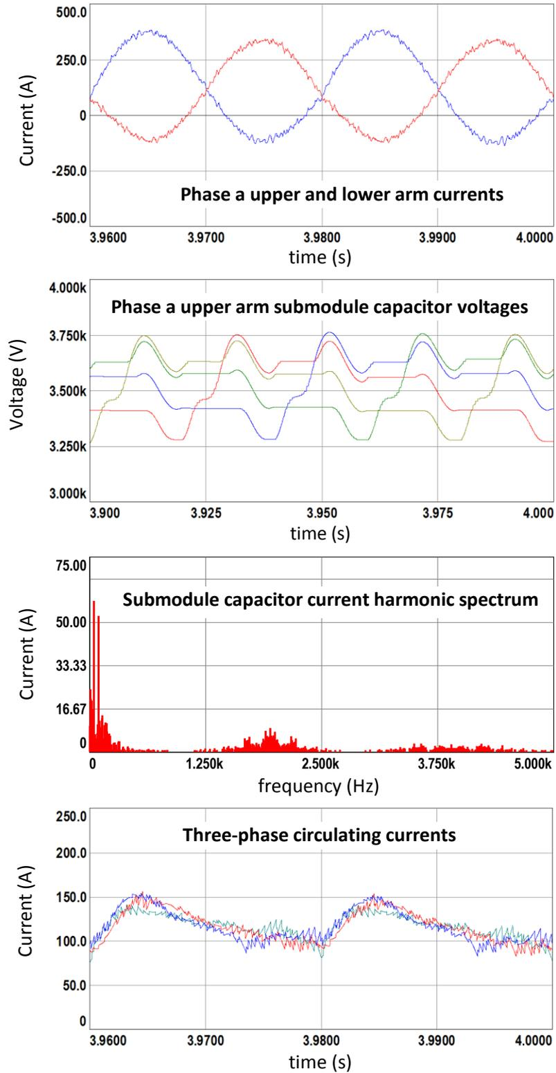
Figure 7.12 (continued) Simulation results for CR method with N+1 level  $V_{ph}$ , half load
