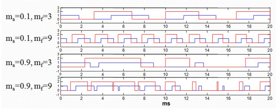
Figure 4.25 Switching pulse patterns of PS
