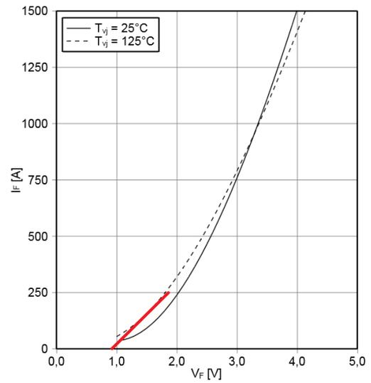
Figure A.1 Linearization of forward voltage and bulk resistance of IGBT at left and diode at right
