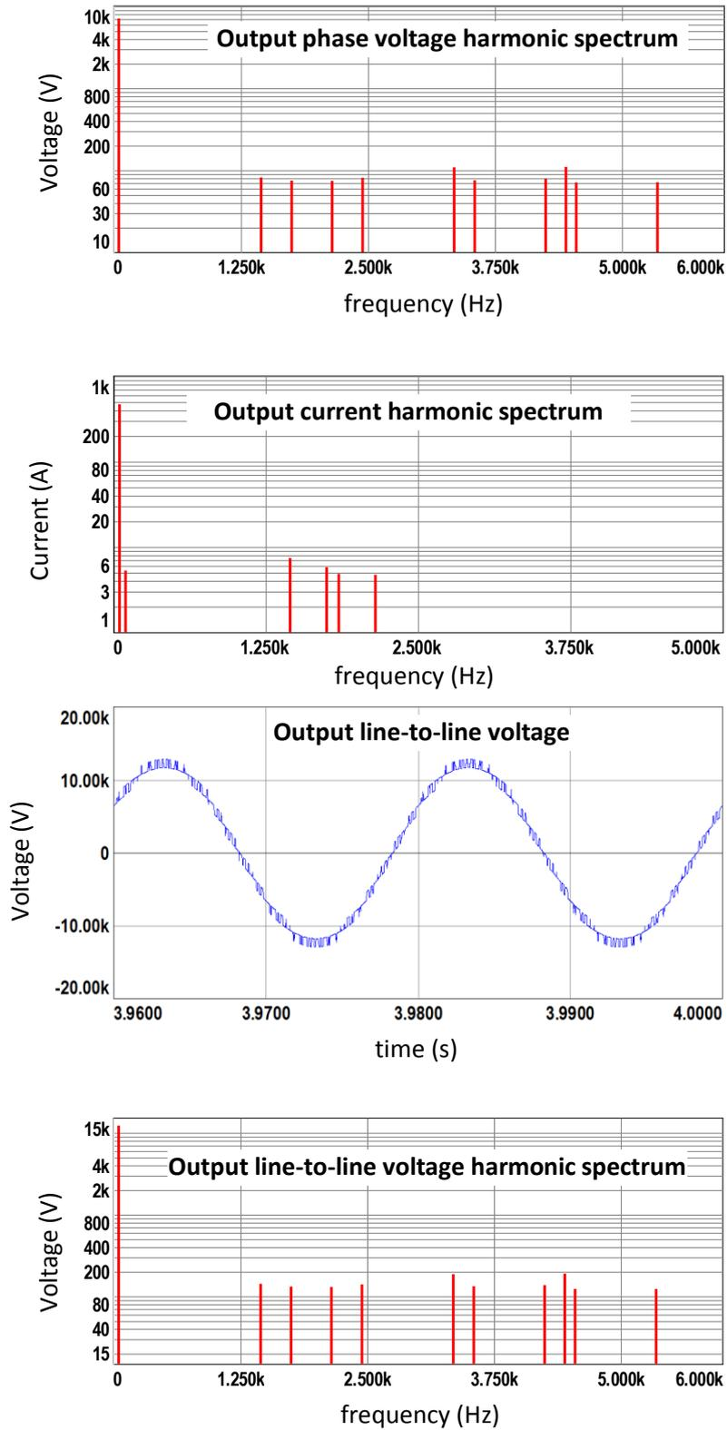
Figure 7.12 (continued) Simulation results for CR method with N+1 level  $V_{ph}$ , half load
