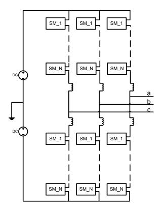
Figure 1.1 Modular multilevel converter
