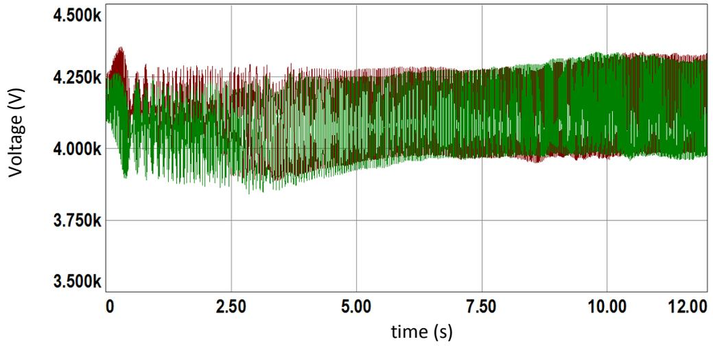
Figure 8.7 Phase a upper and lower arm capacitor voltages of MMC motor drive
