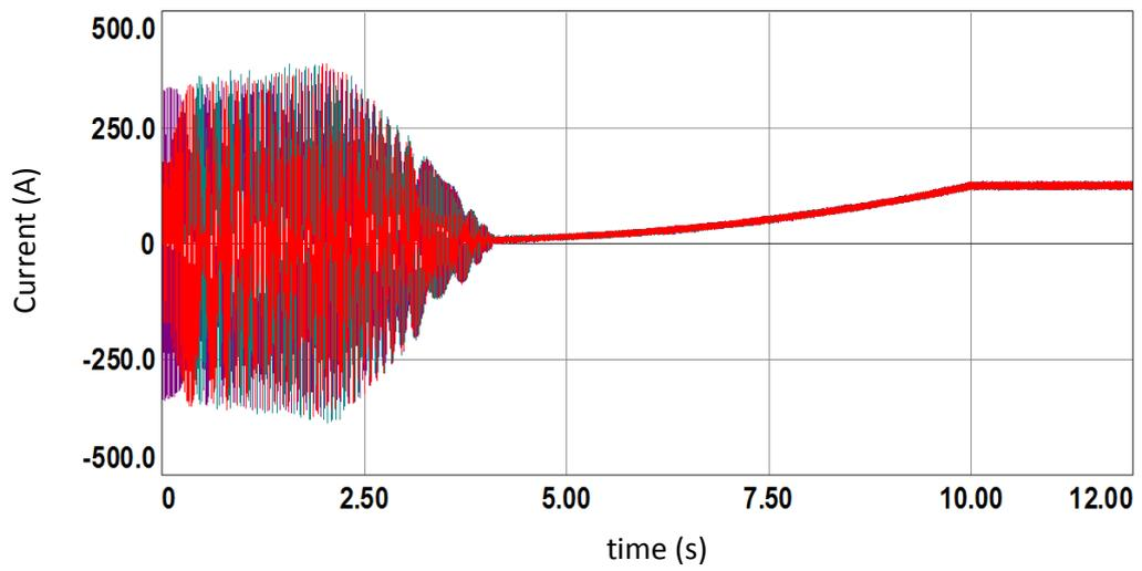
Figure 8.8 Three-phase circulating currents of MMC motor drive
