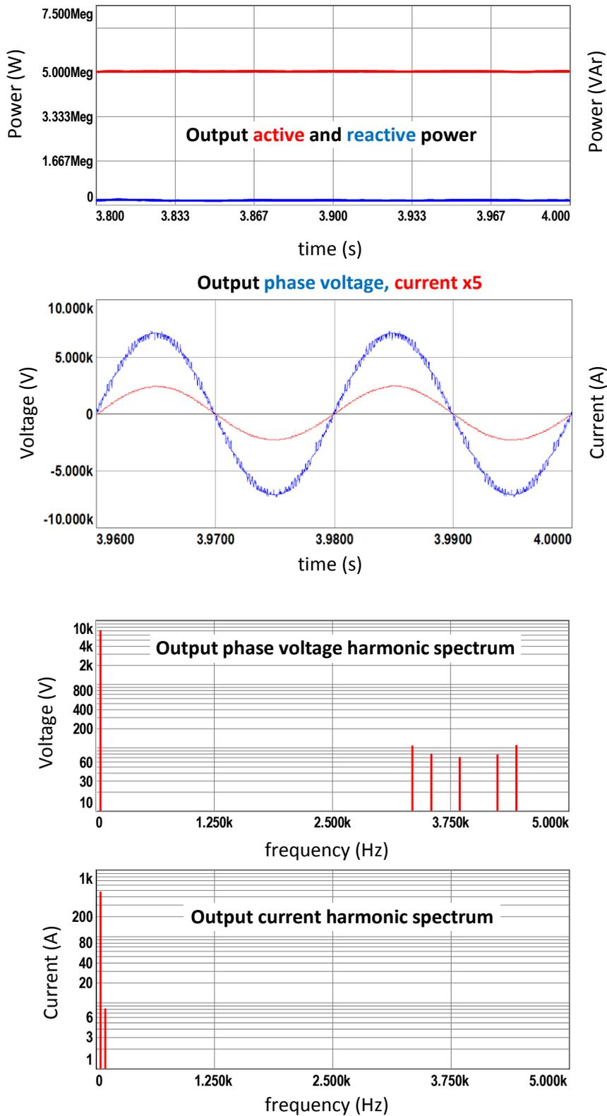
Figure 7.16 Simulation results for CR method with  $2N+1$  level  $V_{ph}$ , half load
