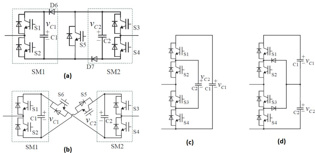
Figure 2.10 (a) The clamp double circuit (b) The five level cross connected circuit (c, d) capacitor-clamped and diode-clamped three-level converters [69]
