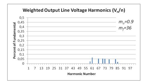
Figure 4.48 Weighted line voltage harmonics of APOD for 2N+1 level V<sub>ph</sub>
