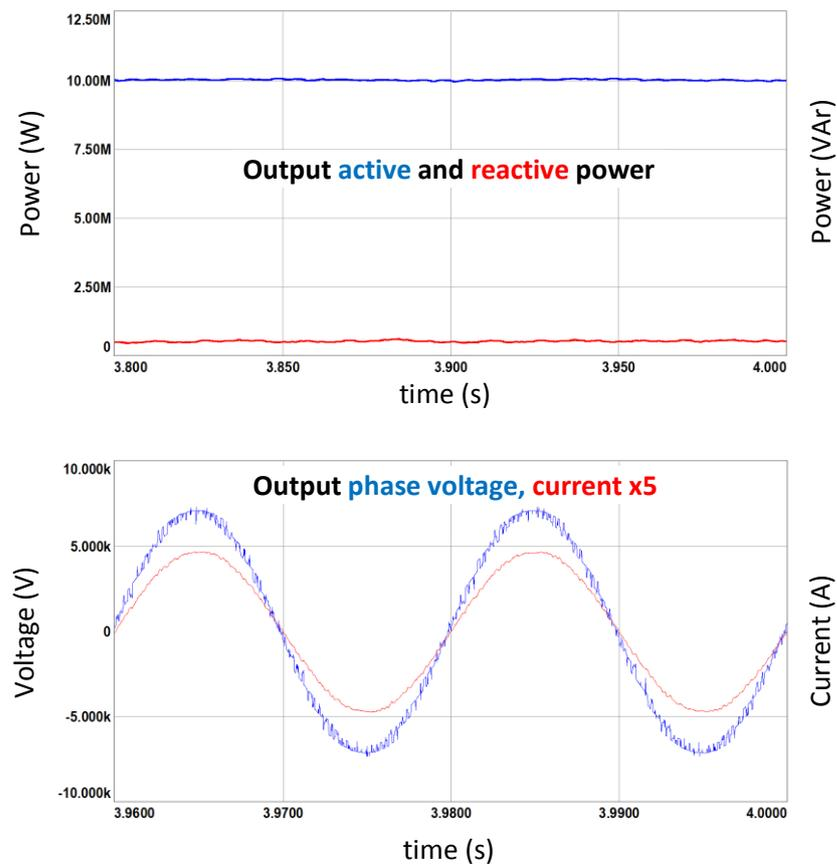
Figure 7.9 Simulation results for PSCB method with  $2N+1$  level  $V_{ph}$ , full load
