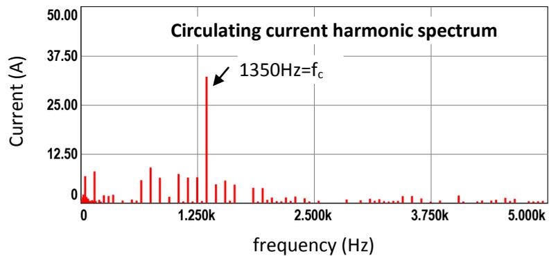
Figure 7.6 (continued) Simulation results for S&S method with  $2N+1$  level  $V_{ph}$ , full load
