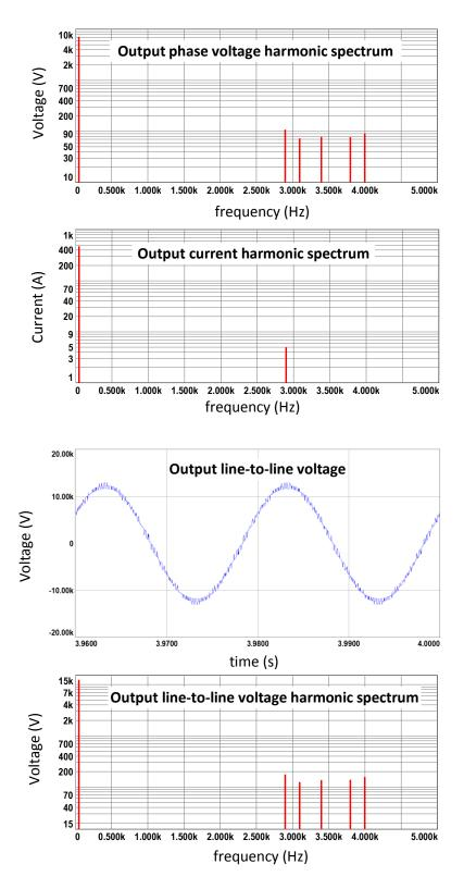
Figure 7.17 (continued) Simulation results for PSCB method with 2N+1 level  $V_{\text{ph}}, \\ half \ \text{load}$
