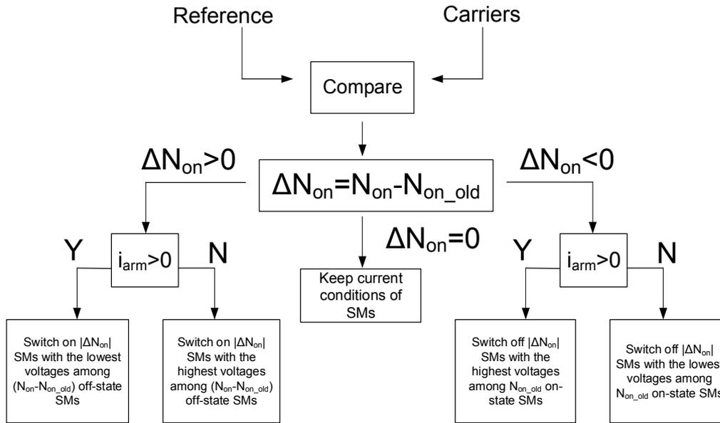
Figure 6.9 Determination of inserted or bypassed submodules for sort and select method with reduced number of switching
