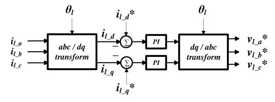
Figure 6.1 Block diagram of active and reactive power control for MMC
