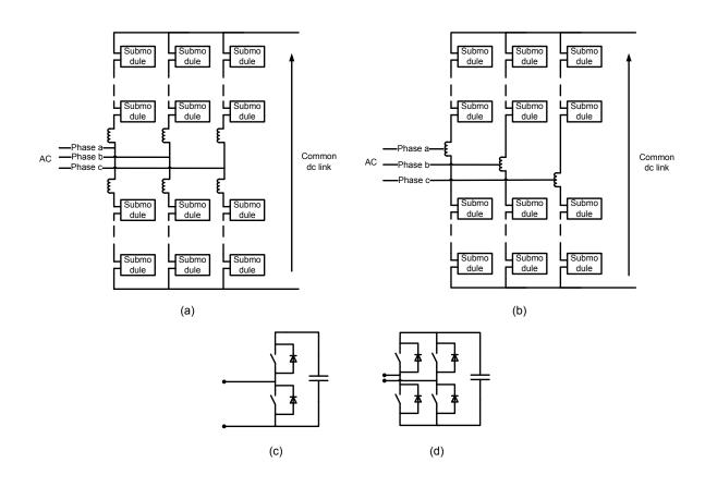
Figure 2.4 Possible circuit configurations of DSCC and DSBC (a) Power circuit using coupled arm inductors (b) Power circuit using non-coupled arm inductors (c) Chopper cell (DSCC) (d) Bridge cell (DSBC)
