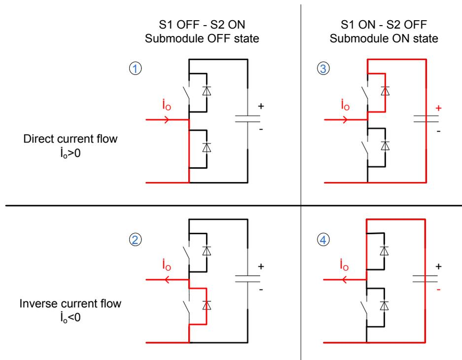
Figure 2.9 States of half-bridge (chopper) circuit and current paths
