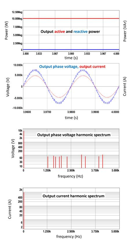
Figure 7.3 Simulation results for S&S-RS method with N+1 level  $V_{ph}$ , full load
