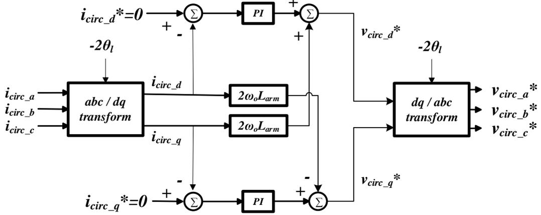
Figure 6.12 Circulating current second harmonic controller block diagram
