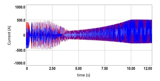
Figure 8.6 Phase a upper and lower arm currents of MMC motor drive
