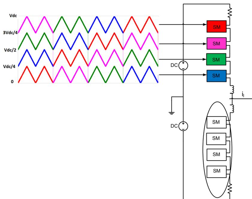
Figure 6.10 Carrier rotation method for submodule capacitor voltage balancing
