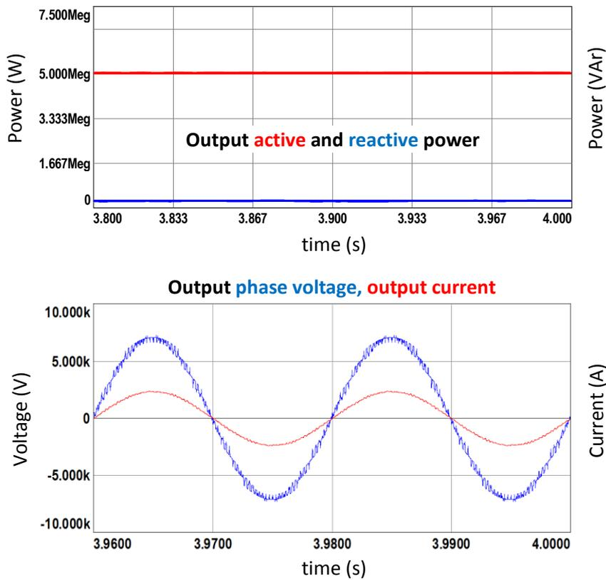
Figure 7.15 Simulation results for S&S-RS method with  $2N+1$  level  $V_{ph}$ , half load
