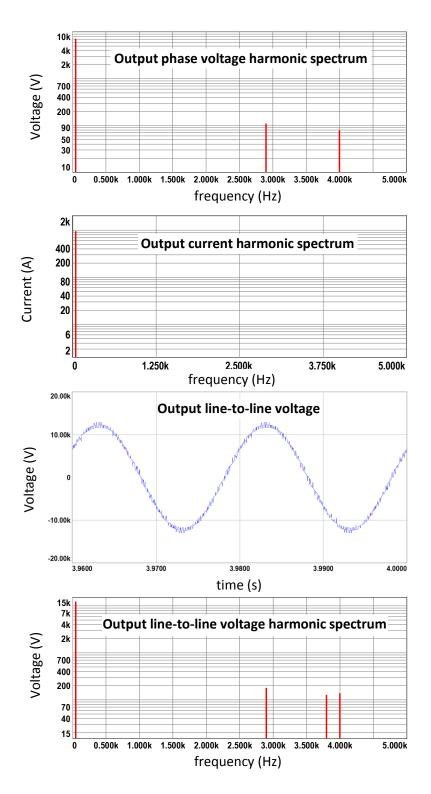
Figure 7.9 (continued) Simulation results for PSCB method with 2N+1 level  $V_{\mbox{\ ph}}$  , full load
