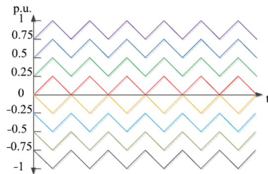
Figure 4.3 Phase opposition disposition (POD) method
