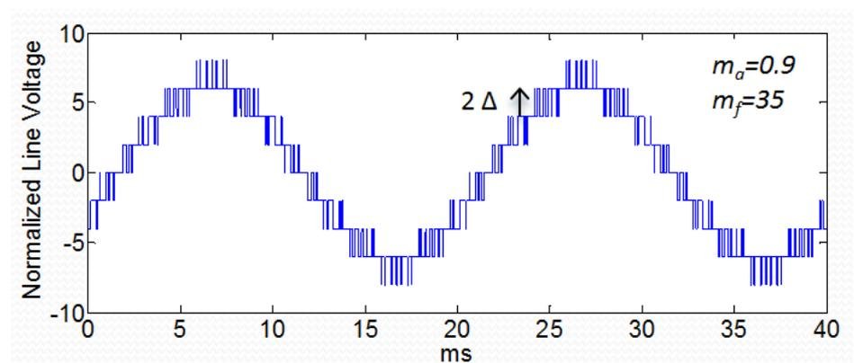
Figure 4.30 Normalized line voltage of PD for N+1 level  $V_{ph}$
