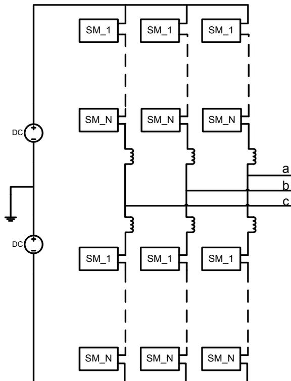
Figure 1.1 Modular multilevel converter
