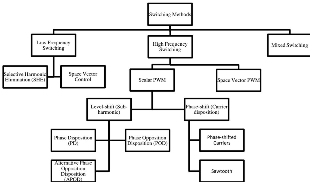
Figure 4.1 Switching methods for modular multilevel converters
