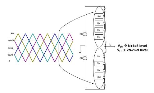
Figure 4.13 Carrier set for N+1 level phase voltage of phase-shift method with even number of submodules
