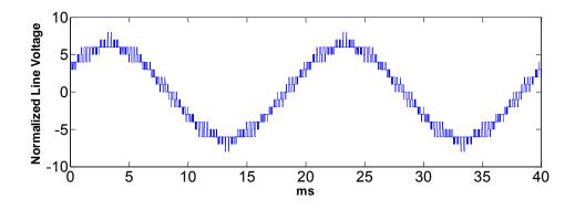
Figure 4.42 Normalized line voltage of PD for 2N+1 level  $V_{\text{ph}}$
