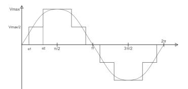
Figure 4.8 Output voltage waveform for a five-level converter, switching angles determined by selective harmonic elimination method
