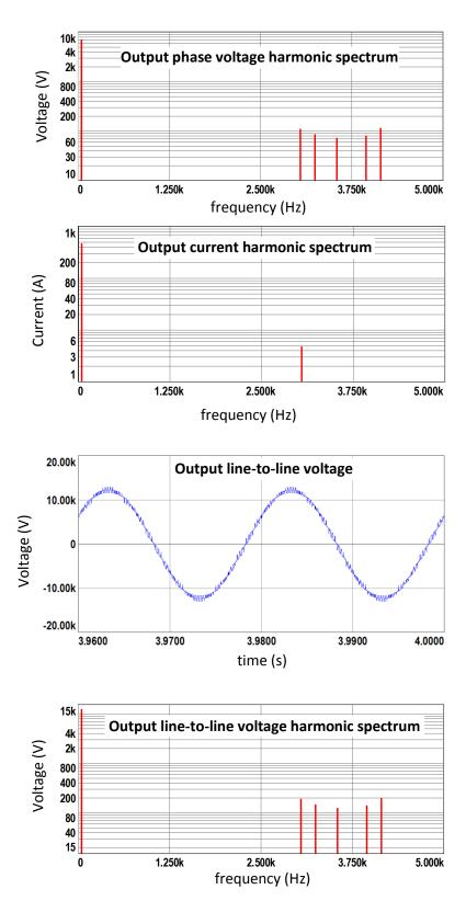
Figure 7.15 (continued) Simulation results for S&S-RS method with 2N+1 level  $V_{\text{ph}}, \\ half load$
