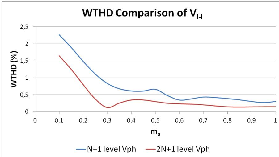
Figure 4.51 WTHD values for changing  $m_f$  and fixed  $m_a=0.9$  at the top and changing  $m_a$  and fixed  $m_f=9$  at the bottom, for N+1 and 2N+1 level  $V_{ph}$
