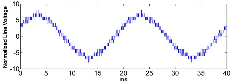
Figure 4.42 Normalized line voltage of PD for  $2N+1$  level  $V_{ph}$
