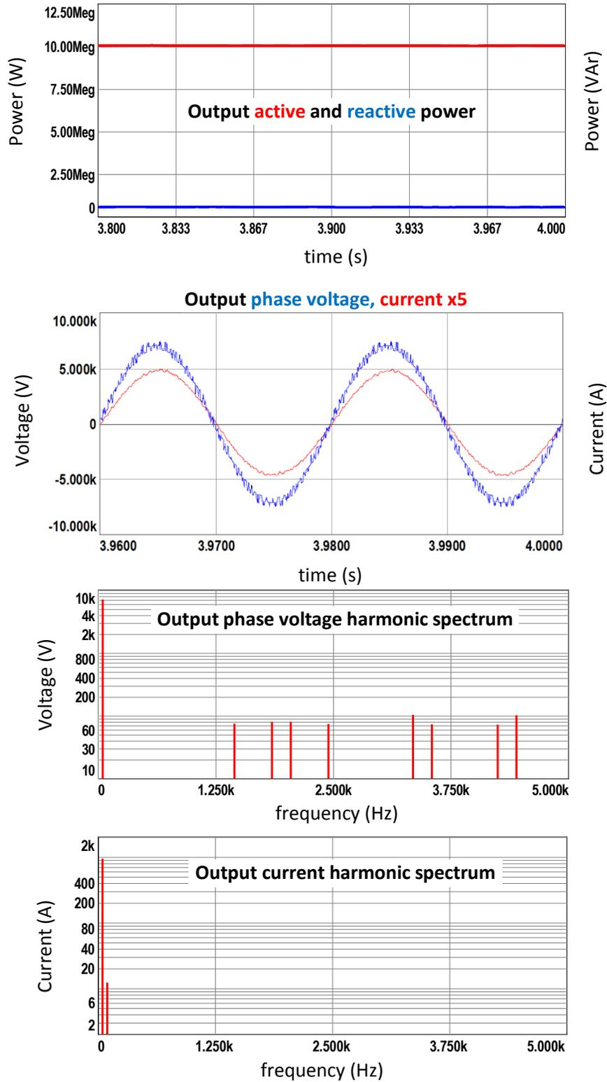
Figure 7.4 Simulation results for CR method with N+1 level  $V_{ph}$ , full load
