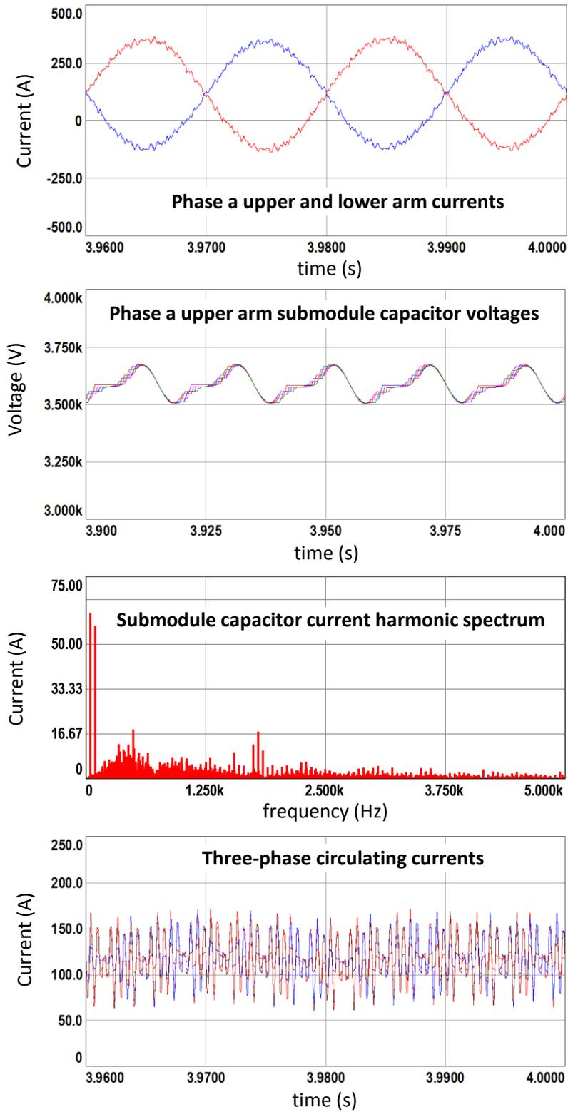
Figure 7.15 (continued) Simulation results for S&S-RS method with  $2N+1$  level  $V_{ph}$ , half load
