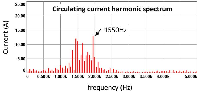
Figure 7.17 (continued) Simulation results for PSCB method with  $2N+1$  level  $V_{ph}$ , half load
