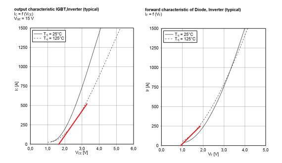
Figure A.1 Linearization of forward voltage and bulk resistance of IGBT at left and diode at right
