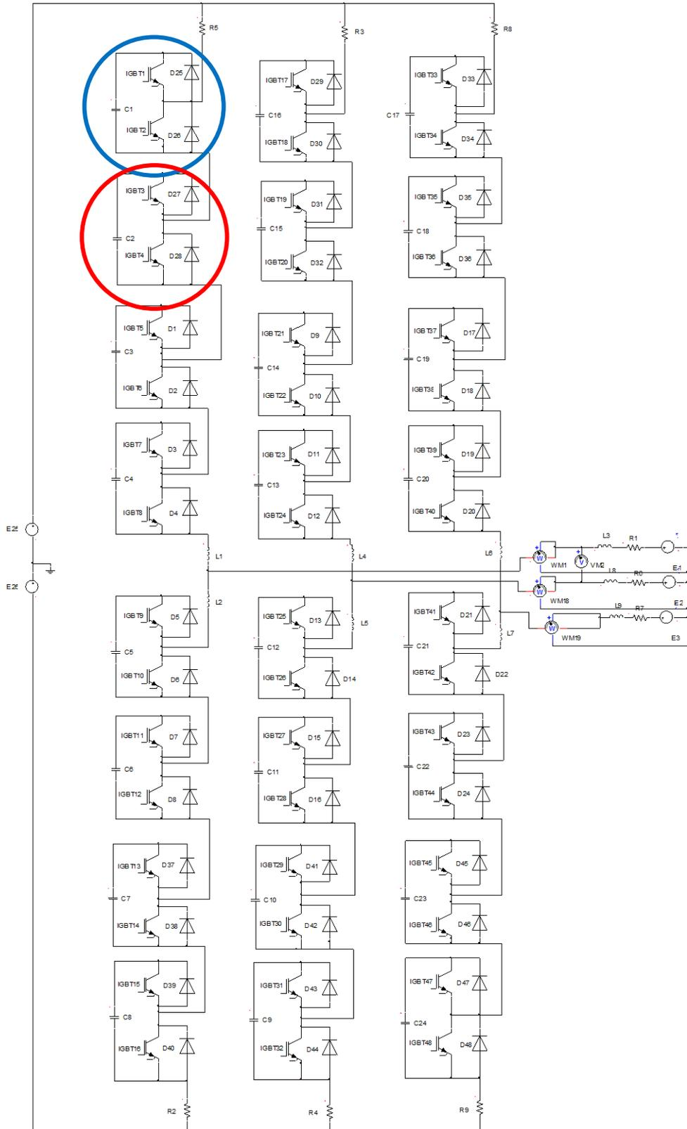
Figure 7.1 Circuit structure of the simulated dc/ac conversion step of an HVDC system in Simplorer
