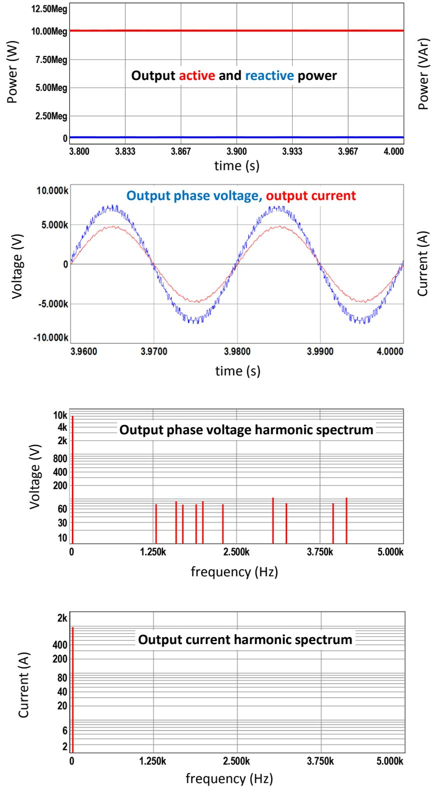
Figure 7.3 Simulation results for S&S-RS method with N+1 level  $V_{ph}$ , full load
