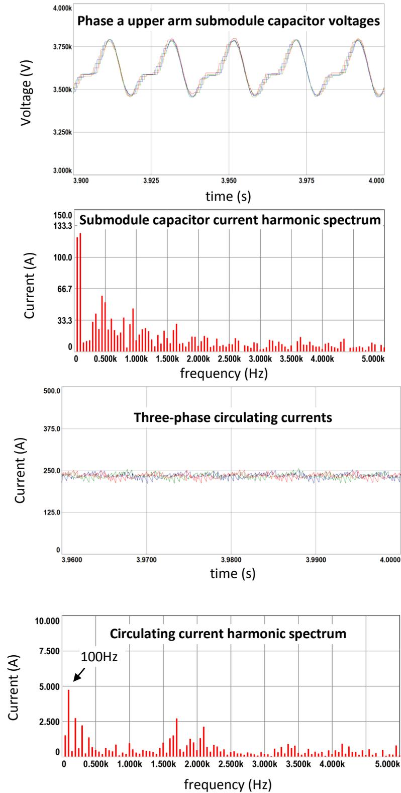
Figure 7.5 (continued) Simulation results for PSCB method with N+1 level  $V_{ph}$ , full load
