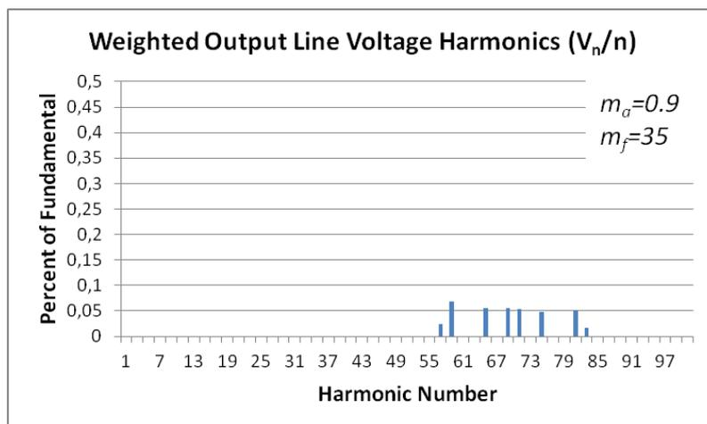
Figure 4.46 Weighted line voltage harmonics of PD for  $2N+1$  level  $V_{ph}$
