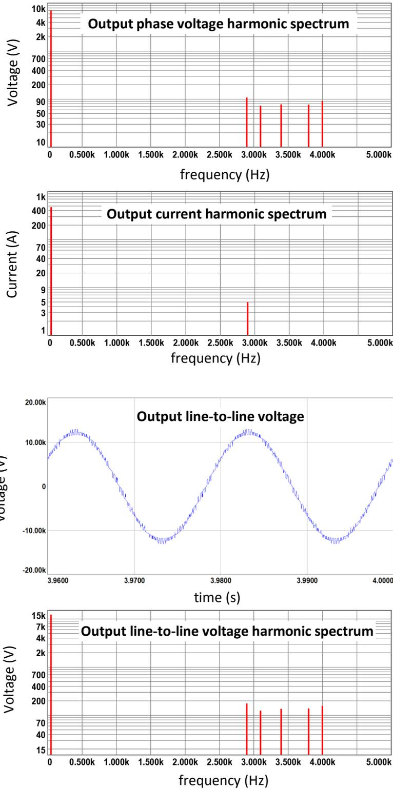
Figure 7.17 (continued) Simulation results for PSCB method with 2N+1 level  $V_{ph}$ , half load
