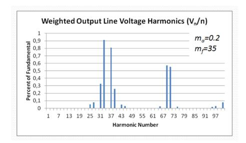
Figure 4.37 Weighted line voltage harmonics of PD for N+1 level V<sub>ph</sub>
