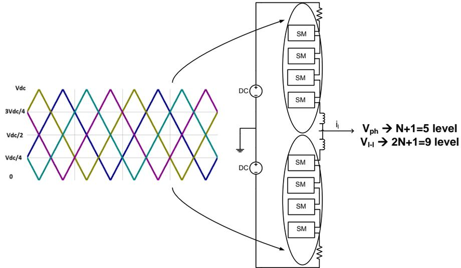
Figure 4.13 Carrier set for  $N+1$  level phase voltage of phase-shift method with even number of submodules
