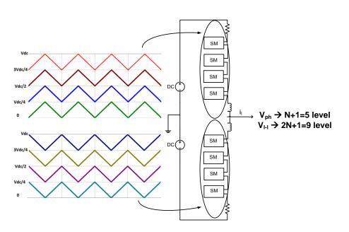
Figure 4.9 Carrier sets for N+1 level phase voltage of PD method
