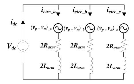
Figure 6.11 Circulating current equivalent circuit of MMC
