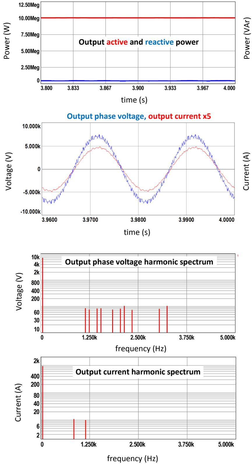
Figure 7.2 Simulation results for S&S method with N+1 level  $V_{ph}$ , full load
