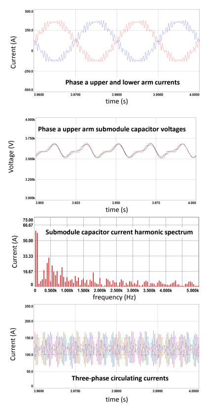
Figure 7.17 (continued) Simulation results for PSCB method with 2N+1 level  $V_{\text{ph}}, \\ \text{half load}$
