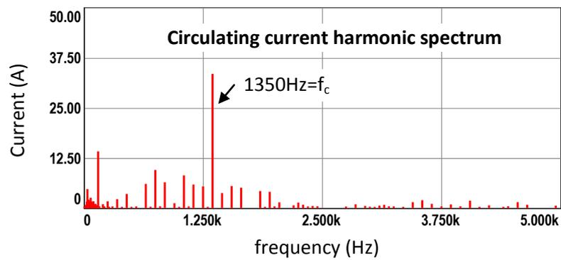
Figure 7.14 (continued) Simulation results for S&S method with  $2N+1$  level  $V_{ph}$ , half load
