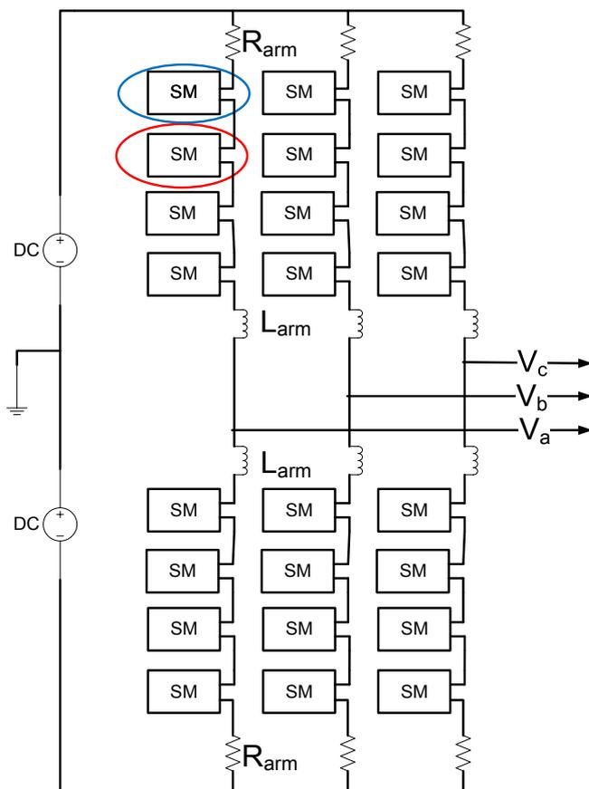
Figure 4.19 MMC with four submodules per arm
