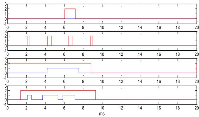
Figure 4.22 Switching pulse patterns of PD for  $(ma=0.1, mf=3)$ ,  $(ma=0.1, mf=9)$ ,  $(ma=0.9, mf=3)$  and  $(ma=0.9, mf=9)$  from the top to the bottom
