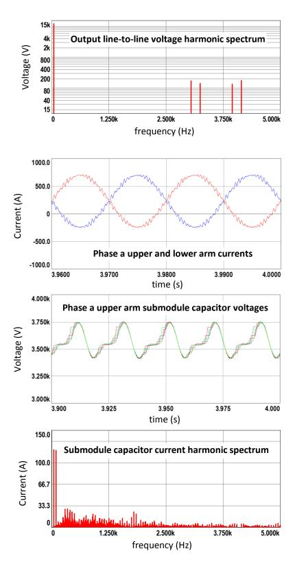
Figure 7.7 (continued) Simulation results for S&S-RS method with 2N+1 level  $V_{\text{ph}}, \\ full \ load$
