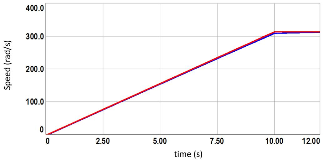
Figure 8.4 Speed reference and speed of the induction machine
