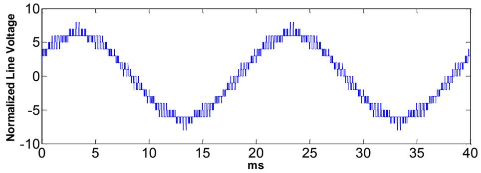
Figure 4.43 Normalized line voltage of POD for  $2N+1$  level  $V_{ph}$
