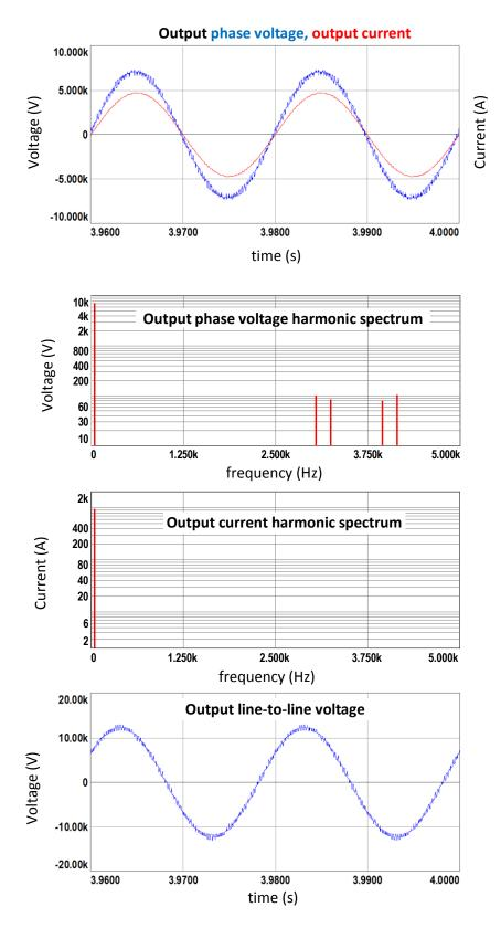
Figure 7.7 (continued) Simulation results for S&S-RS method with 2N+1 level  $V_{\text{ph}}, \\ full \ load$
