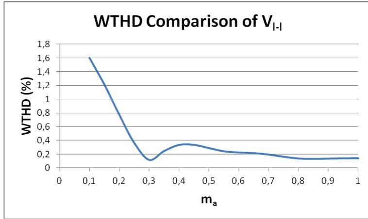
Figure 4.49 WTHD values for changing  $m_a$  and fixed  $m_f=3$  and  $m_f=9$  at the top and at the bottom, valid for all the LS and PS methods for  $2N+1$  level  $V_{ph}$
