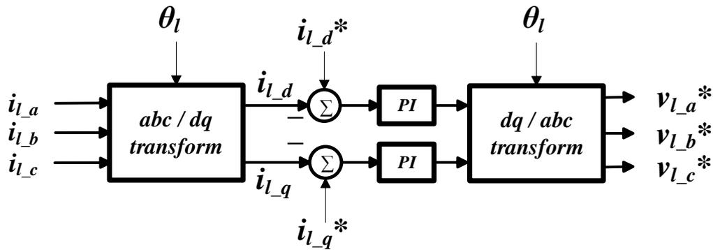
Figure 6.1 Block diagram of active and reactive power control for MMC
