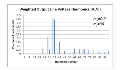
Figure 4.35 Weighted line voltage harmonics of POD for N+1 level  $V_{ph}$
