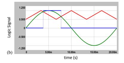
Figure 4.20 Carrier, reference and switching pulse signals for (a) PS and (b) PD methods for  $m_a=1$  and  $m_f=3$
