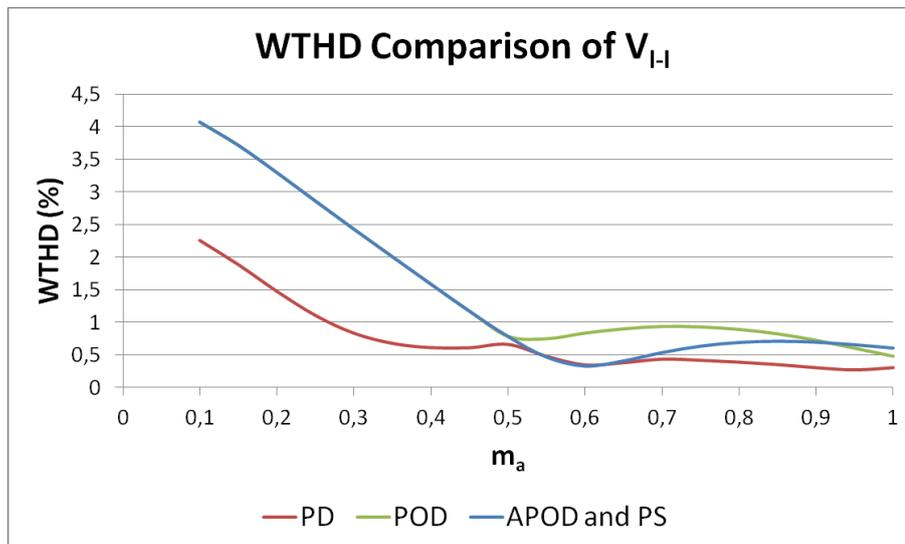
Figure 4.39 WTHD values for changing  $m_a$  and fixed  $m_f=3$  and  $m_f=9$  at the top and at the bottom, for  $N+1$  level  $V_{ph}$
