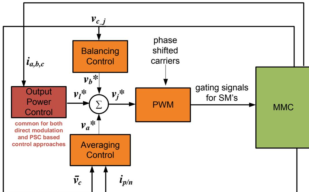
Figure 6.14 Block diagram of phase-shifted carrier based control
