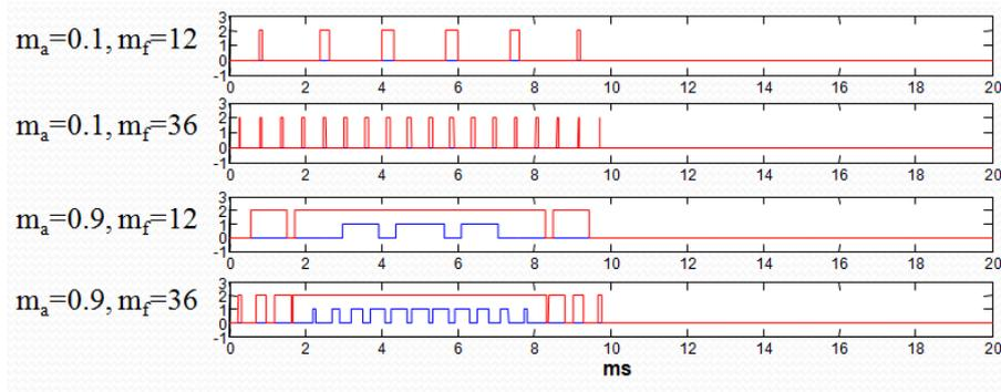
Figure 4.28 Switching pulse patterns of APOD
