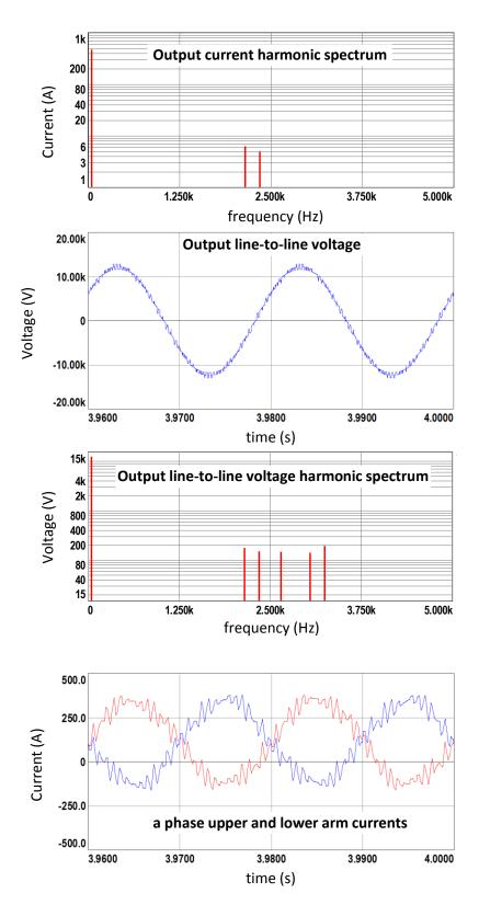
Figure 7.14 (continued) Simulation results for S&S method with 2N+1 level  $V_{\text{ph}}, \\ half load$
