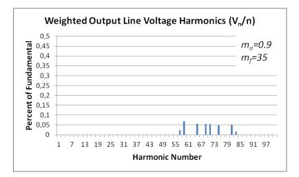
Figure 4.46 Weighted line voltage harmonics of PD for 2N+1 level V<sub>ph</sub>
