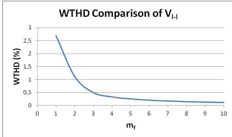
Figure 4.50 WTHD values for changing  $m_f$  and fixed  $m_a=0.6$  and  $m_a=0.9$  at the top and at the bottom, valid for all the LS and PS methods for  $2N+1$  level  $V_{ph}$
