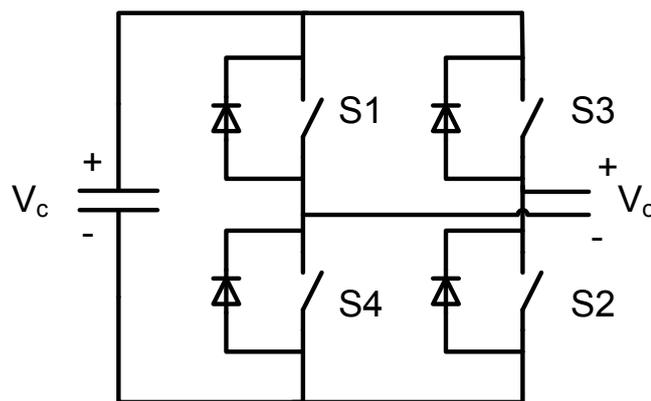
Figure 2.5 The full-bridge circuit topology
