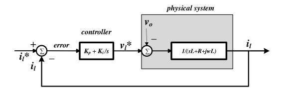
Figure 6.4 Overview of the output current PI controller and physical system with output voltage
