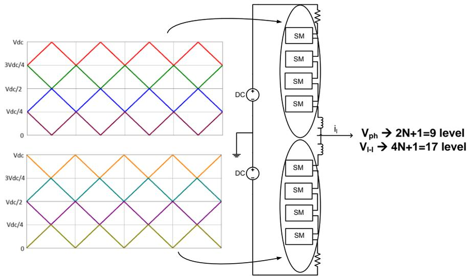
Figure 4.16 Carrier set for  $2N+1$  level phase voltage of APOD method
