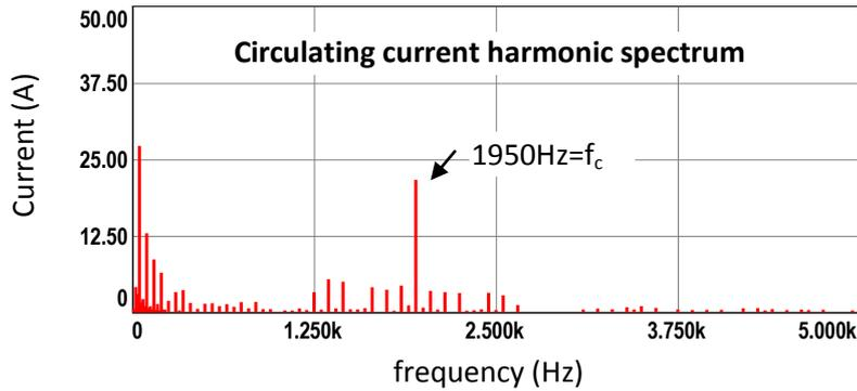
Figure 7.8 (continued) Simulation results for CR method with  $2N+1$  level  $V_{ph}$ , full load
