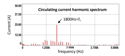
Figure 7.15 (continued) Simulation results for S&S-RS method with 2N+1 level  $V_{\text{ph}}, \\ half load$
