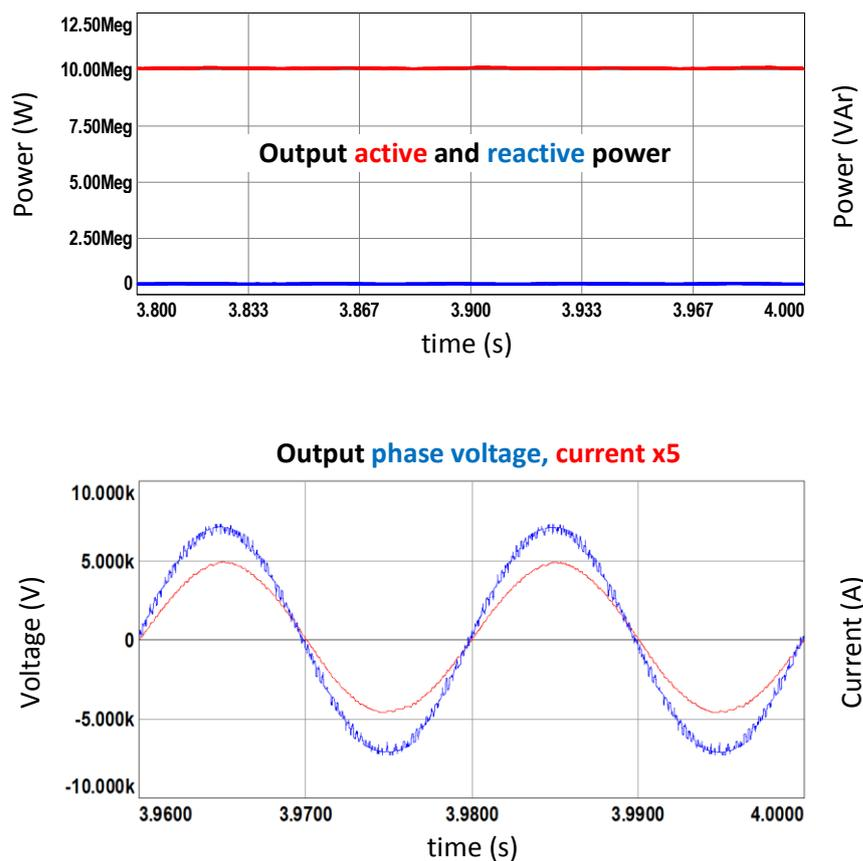
Figure 7.8 Simulation results for CR method with 2N+1 level  $V_{ph}$ , full load
