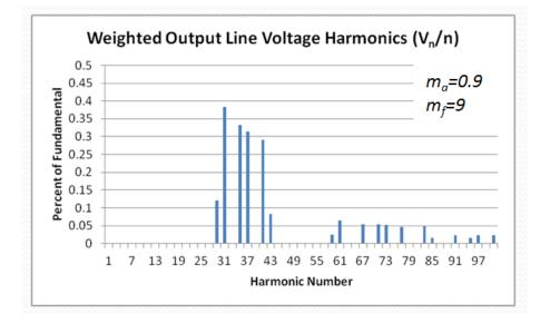
Figure 4.33 Weighted line voltage harmonics of PS for N+1 level V<sub>ph</sub>
