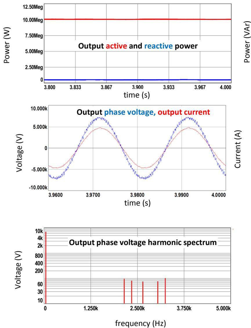
Figure 7.6 Simulation results for S&S method with 2N+1 level  $V_{ph}$ , full load
