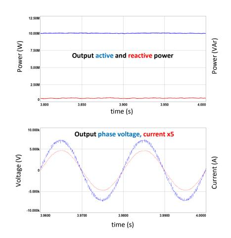
Figure 7.9 Simulation results for PSCB method with 2N+1 level V<sub>ph</sub>, full load
