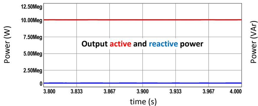
Figure 7.7 Simulation results for S&S-RS method with  $2N+1$  level  $V_{ph}$ , full load
