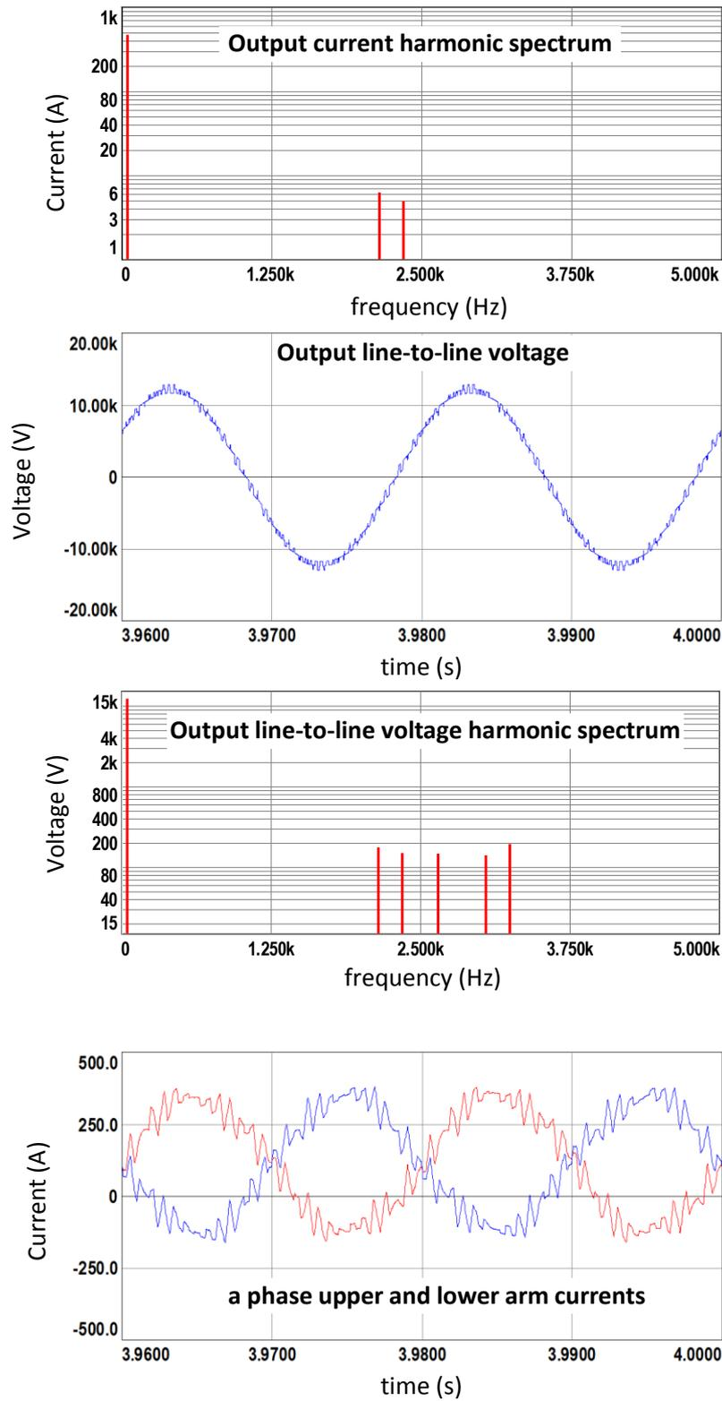
Figure 7.14 (continued) Simulation results for S&S method with  $2N+1$  level  $V_{ph}$ , half load
