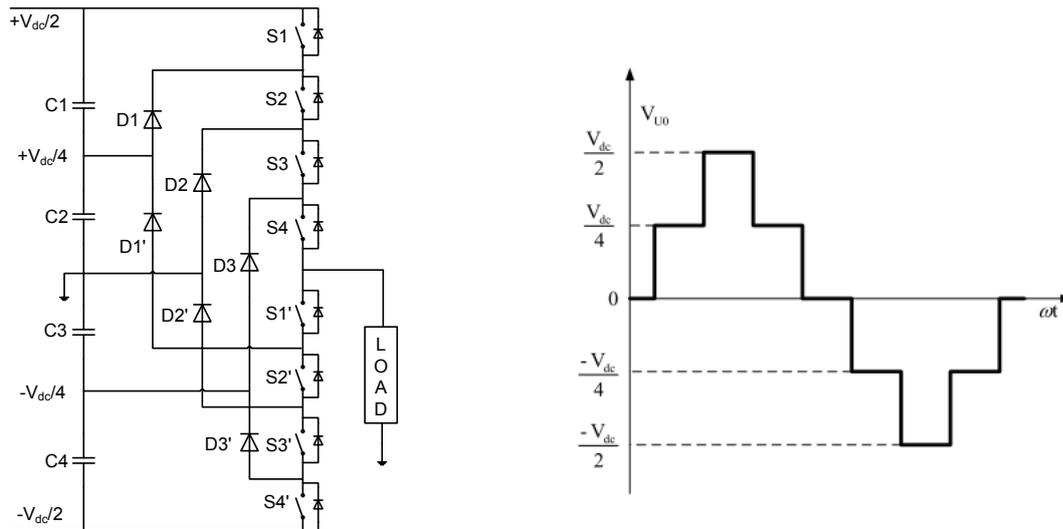
Figure 2.1 Single-phase five-level diode-clamped converter at left and output voltage waveform at right
