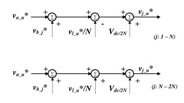
Figure 6.17 Reference signal generation for upper and lower arm submodules
