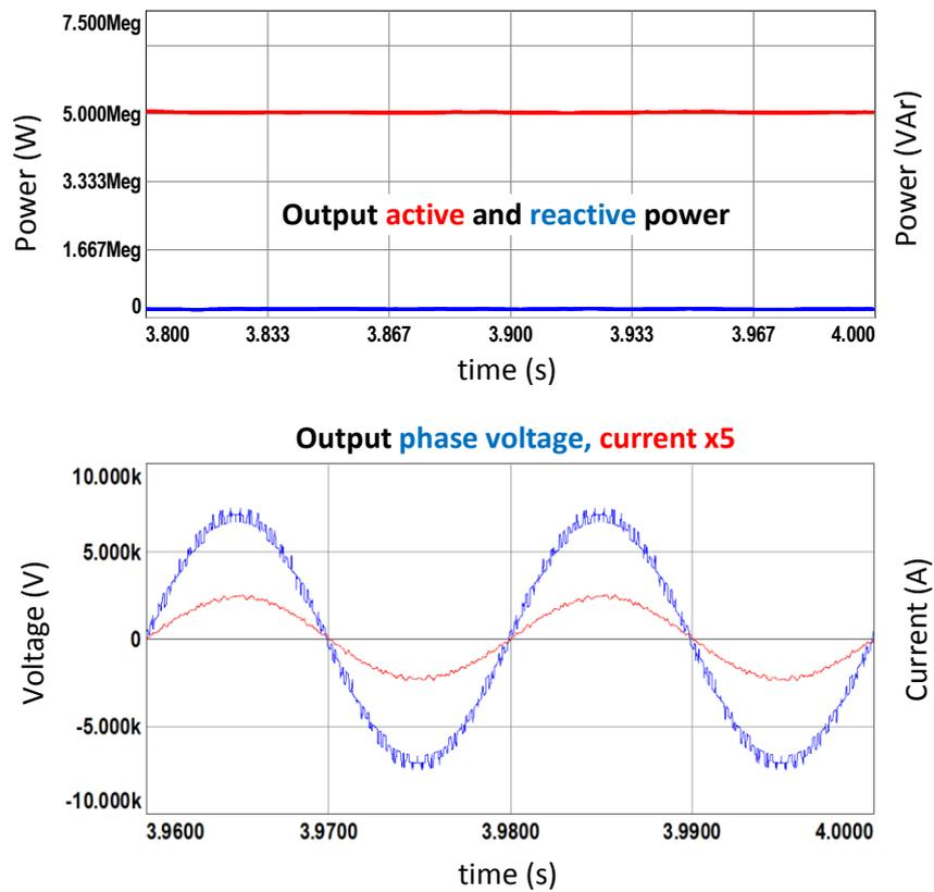
Figure 7.12 Simulation results for CR method with N+1 level  $V_{ph}$ , half load
