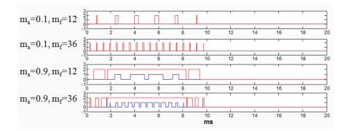
Figure 4.27 Switching pulse patterns of POD
