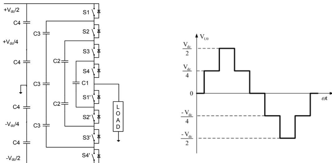
Figure 2.2 Single-phase five level flying capacitor converter at left and output voltage waveform at right
