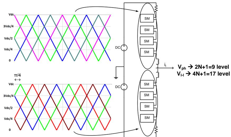
Figure 4.18 Carrier sets for  $2N+1$  level phase voltage of phase-shift method with even number of submodules
