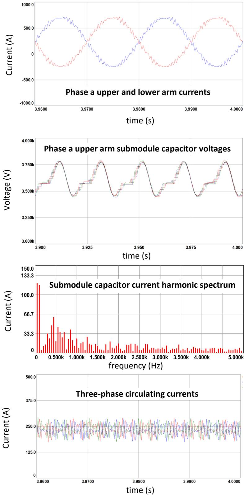
Figure 7.9 (continued) Simulation results for PSCB method with  $2N+1$  level  $V_{ph}$ , full load
