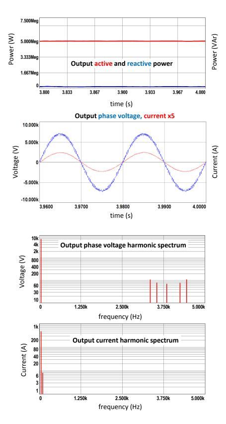
Figure 7.16 Simulation results for CR method with 2N+1 level  $V_{ph}$ , half load
