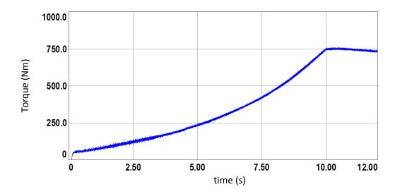
Figure 8.2 Torque reference and output of the induction machine
