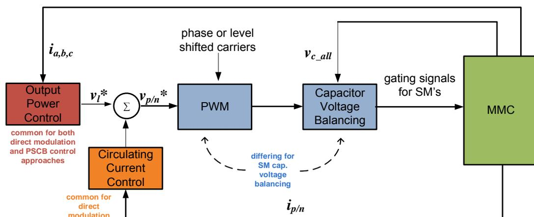
Figure 6.6 Block diagram of direct modulation method
