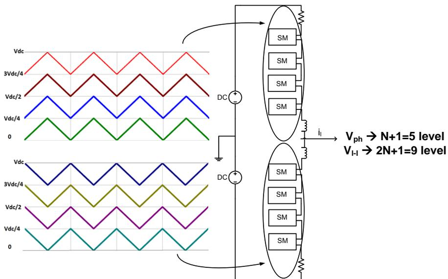
Figure 4.9 Carrier sets for N+1 level phase voltage of PD method
