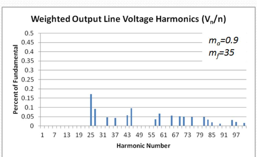
Figure 4.34 Weighted line voltage harmonics of PD for N+1 level  $V_{ph}$
