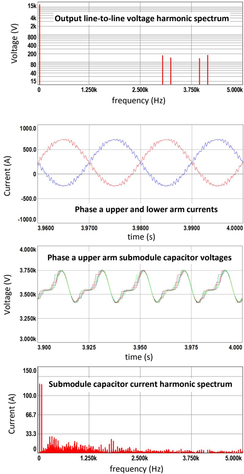
Figure 7.7 (continued) Simulation results for S&S-RS method with  $2N+1$  level  $V_{ph}$ , full load
