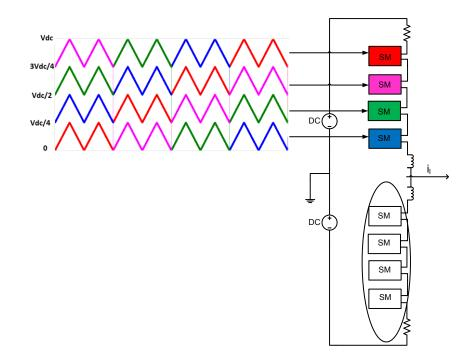
Figure 6.10 Carrier rotation method for submodule capacitor voltage balancing
