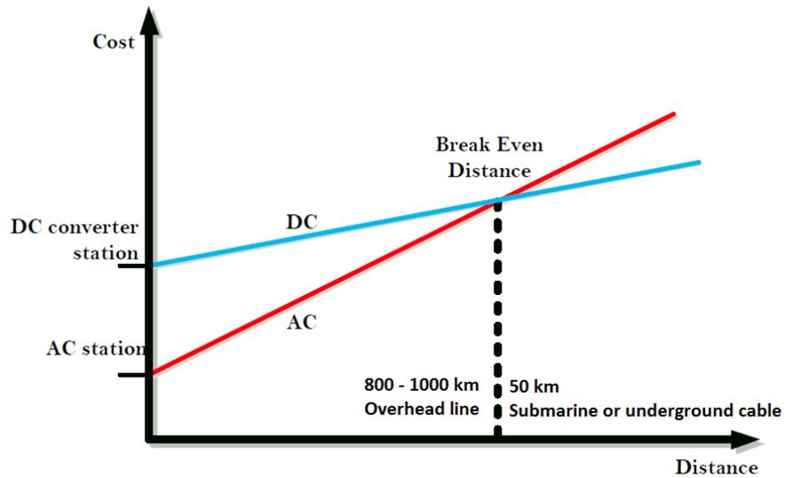
Figure 1.3 Cost estimations for ac and HVDC transmission by distance [3]
