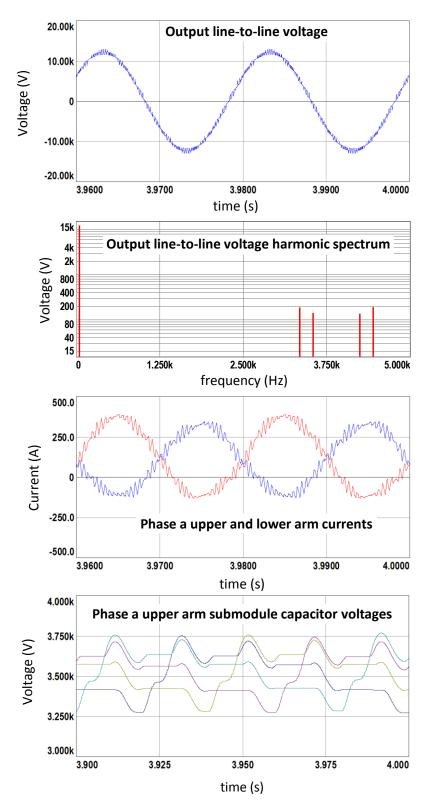
Figure 7.16 (continued) Simulation results for CR method with 2N+1 level  $V_{\text{ph}},$  half load
