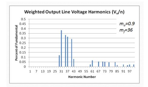
Figure 4.36 Weighted line voltage harmonics of APOD for N+1 level V<sub>ph</sub>
