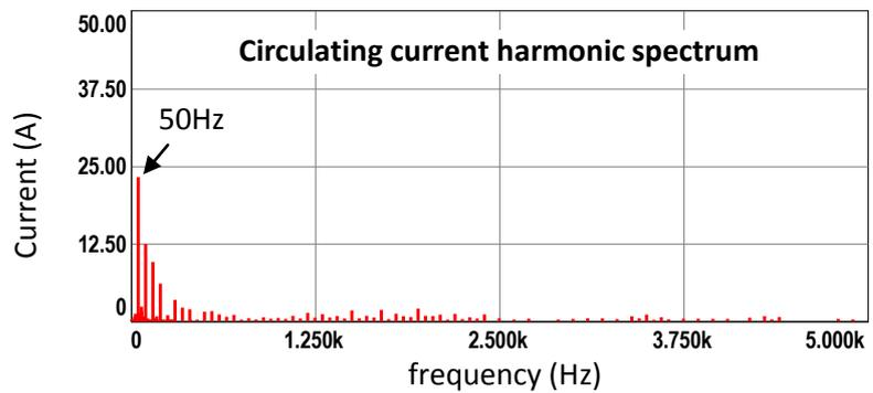
Figure 7.4 (continued) Simulation results for CR method with  $N+1$  level  $V_{ph}$ , full load
