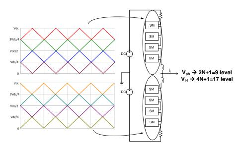
Figure 4.16 Carrier set for 2N+1 level phase voltage of APOD method
