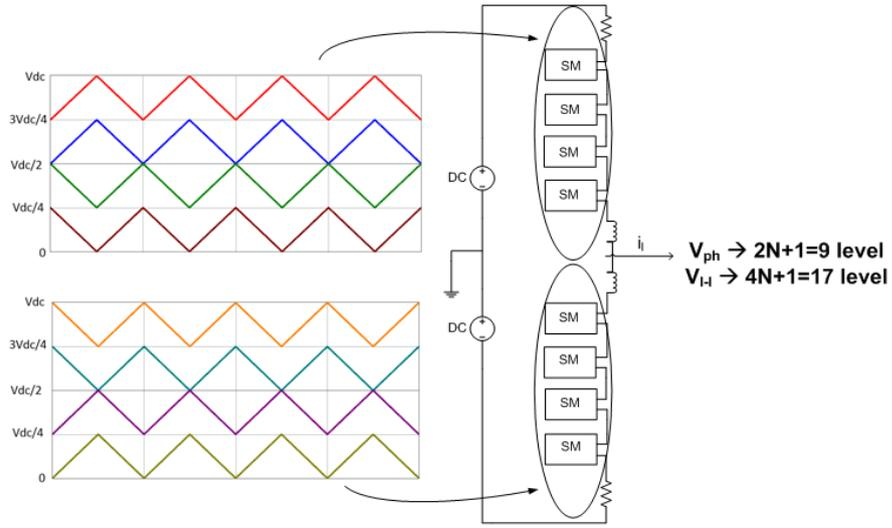
Figure 4.15 Carrier sets for  $2N+1$  level phase voltage of POD method
