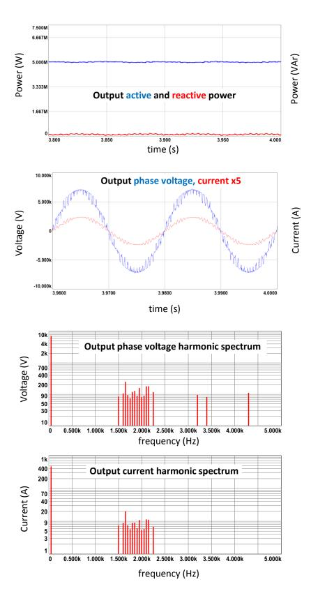
Figure 7.13 Simulation results for PSCB method with N+1 level  $V_{\text{ph}},$  half load
