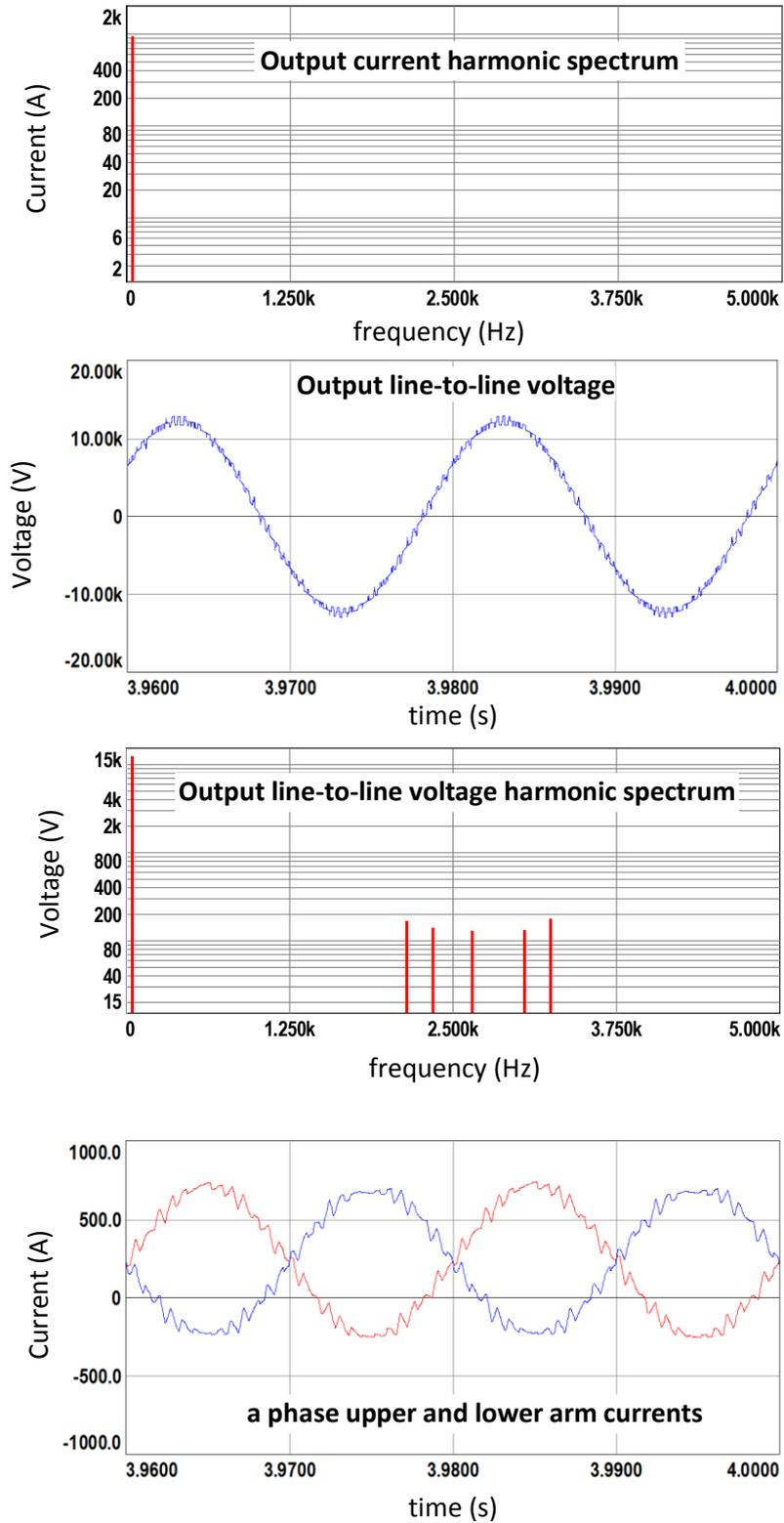
Figure 7.6 (continued) Simulation results for S&S method with  $2N+1$  level  $V_{ph}$ , full load
