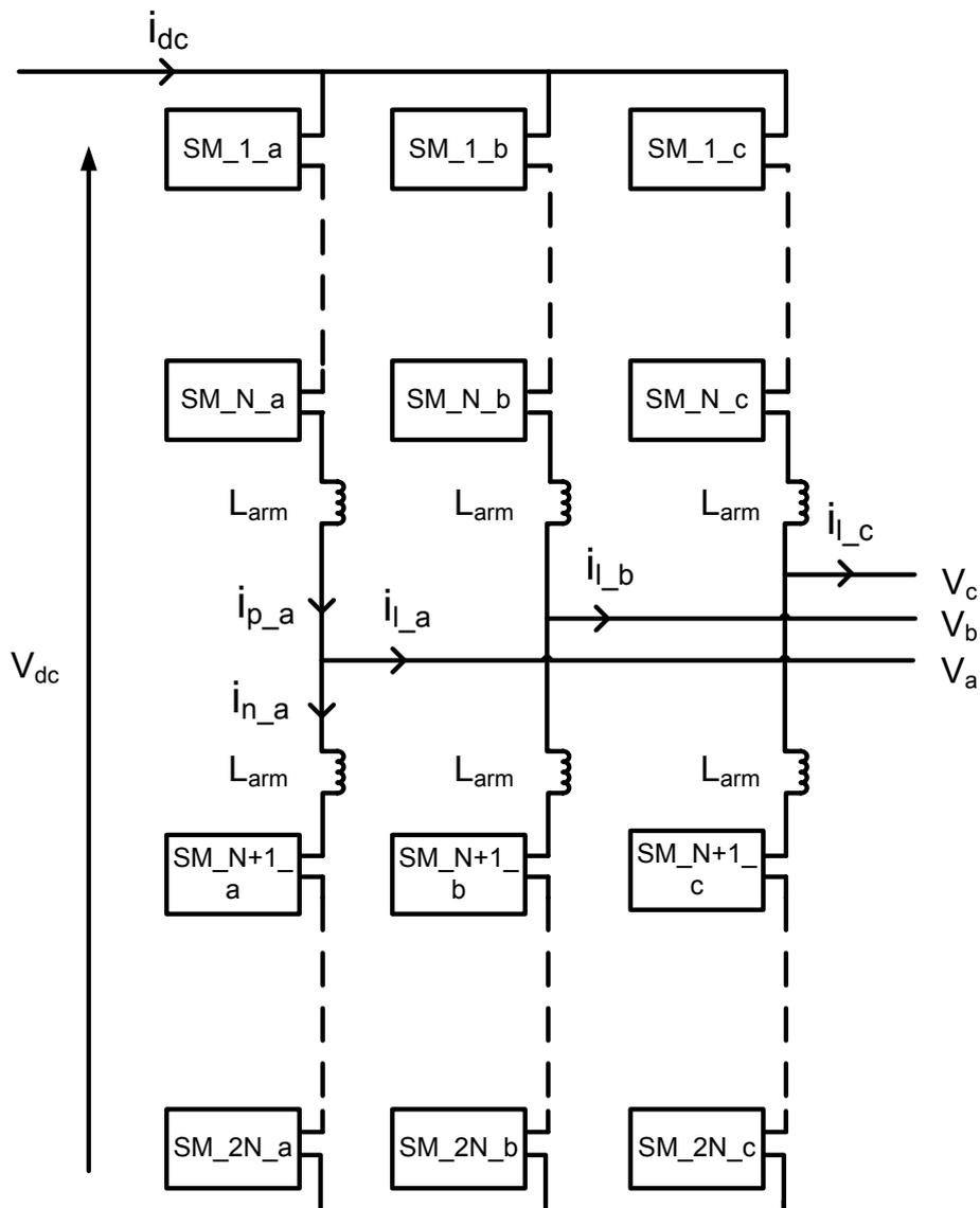
Figure 2.7 Circuit topology of modular multilevel converter
