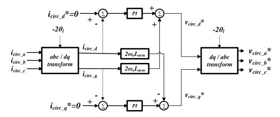
Figure 6.12 Circulating current second harmonic controller block diagram
