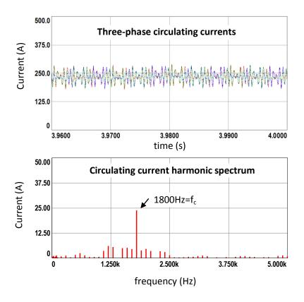
Figure 7.7 (continued) Simulation results for S&S-RS method with 2N+1 level  $V_{\text{ph}}, \\ full \ load$
