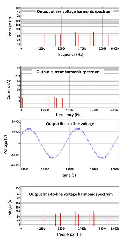
Figure 7.12 (continued) Simulation results for CR method with N+1 level  $V_{\text{ph}},$  half load
