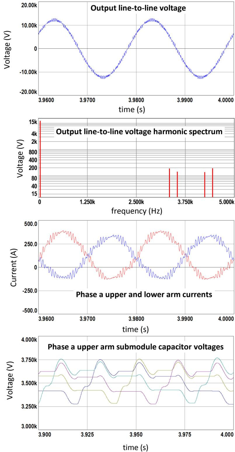
Figure 7.16 (continued) Simulation results for CR method with  $2N+1$  level  $V_{ph}$ , half load
