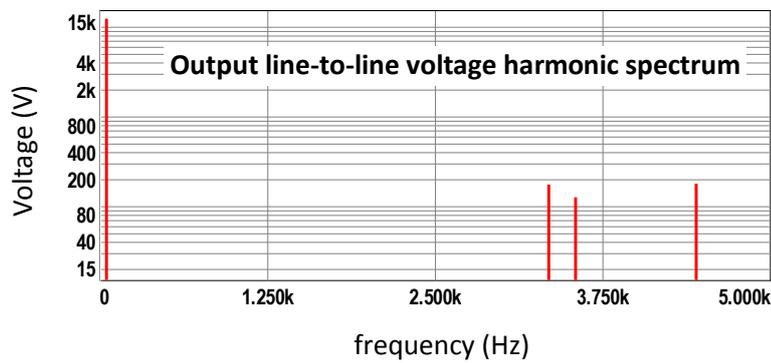
Figure 7.8 (continued) Simulation results for CR method with  $2N+1$  level  $V_{ph}$ , full load
