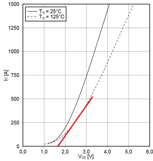
**forward characteristic of Diode, Inverter (typical)**
