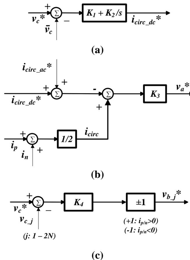
Figure 8.1 Block diagrams for (a) averaging control, (b) circulating current control and (c) balancing control while low frequency operation of MMC
