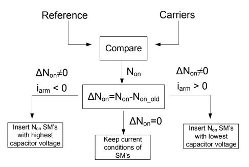
Figure 6.8 Determination of inserted submodules to the current path for sort and select method
