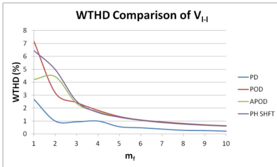
Figure 4.40 WTHD values for changing  $m_f$  and fixed  $m_a=0.6$  and  $m_a=0.9$  at the top and at the bottom, for  $N+1$  level  $V_{ph}$
