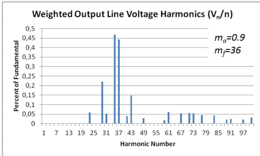
Figure 4.35 Weighted line voltage harmonics of POD for N+1 level  $V_{ph}$
