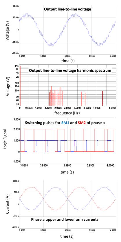
Figure 7.5 (continued) Simulation results for PSCB method with N+1 level  $V_{\text{ph}}\text{, full load}$
