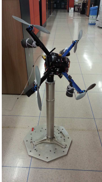
Figure 6.1: Test Setup for Attitude Control
