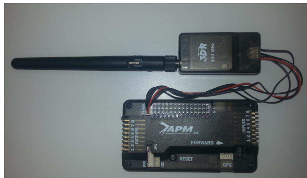
Figure 5.5: Connection of Wireless Telemetry Kit to APM 2.6
