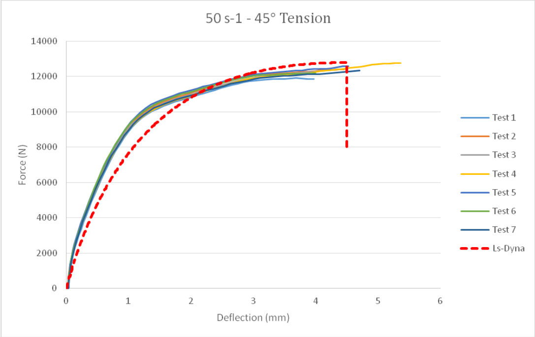
Figure 5-23 Force-Deflection Curves of the Coupon Test and the FE Simulation ( 50 \text{ s}^{-1} , 45^\circ Tension)
