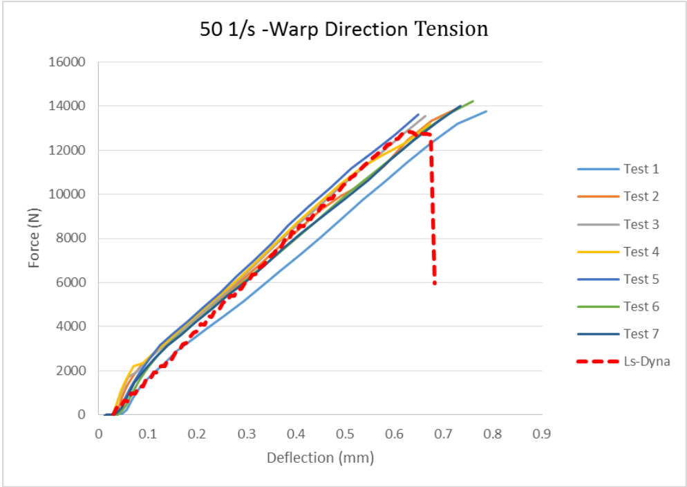
Figure 5-19 Force-Deflection Curves of the Coupon Test and the FE Simulation (50 s-1, Warp Direction Tension)
