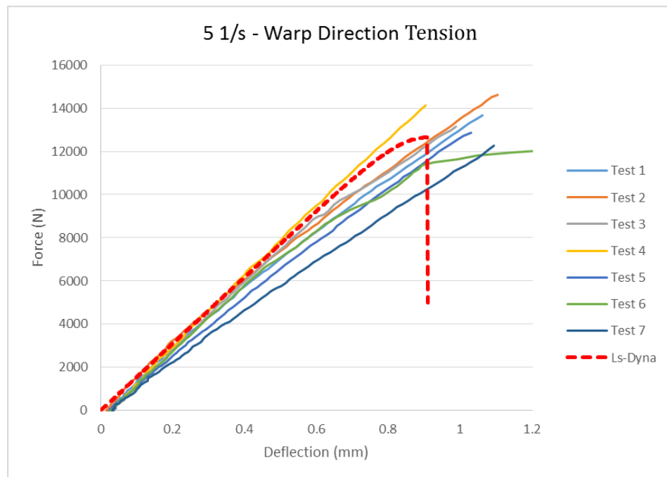
Figure 5-18 Force-Deflection Curves of the Coupon Test and the FE Simulation ( 5 \text{ s}^{-1} , Warp Direction Tension)
