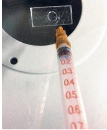
Figure 3.8 Injection of liquid metal inside the microchannels
