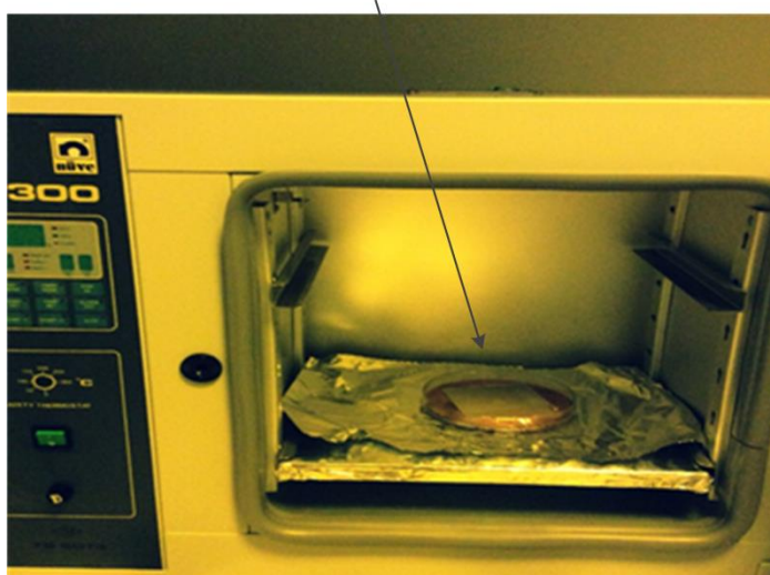
Figure 2.6 Curing the PDMS in the oven.
