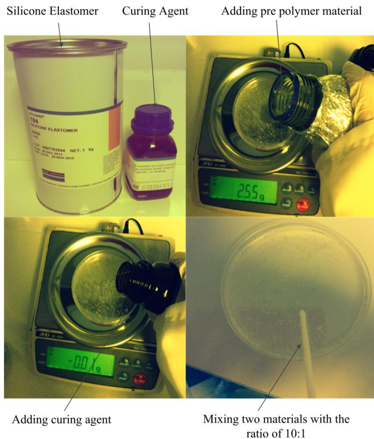
Figure 2.2 (a) Prepolymer base material and curing agent, (b) Pouring prepolymer,
