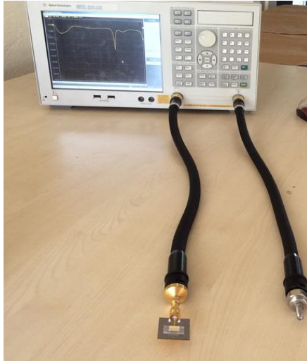
Figure 4.11 Measurement of reflection coefficient with network analyzer.
