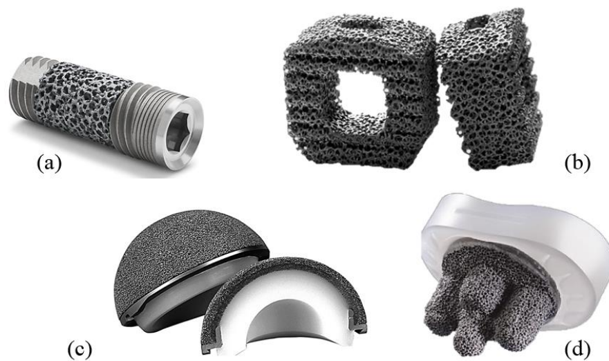
Figure 2.8 Porous metallic materials used in various biomedical application areas; (a) trabecular metal dental implant, (b) fusion device, (c) continuum acetabular system and (d) trabecular metal glenoid fixation [37].
