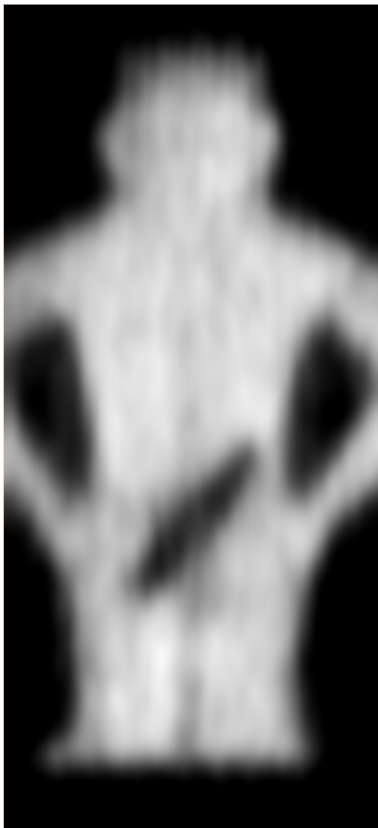
Figure 5.12: Image obtained from built-in algorithm of the passive imaging system, resolution is 271 x 124 pixels
