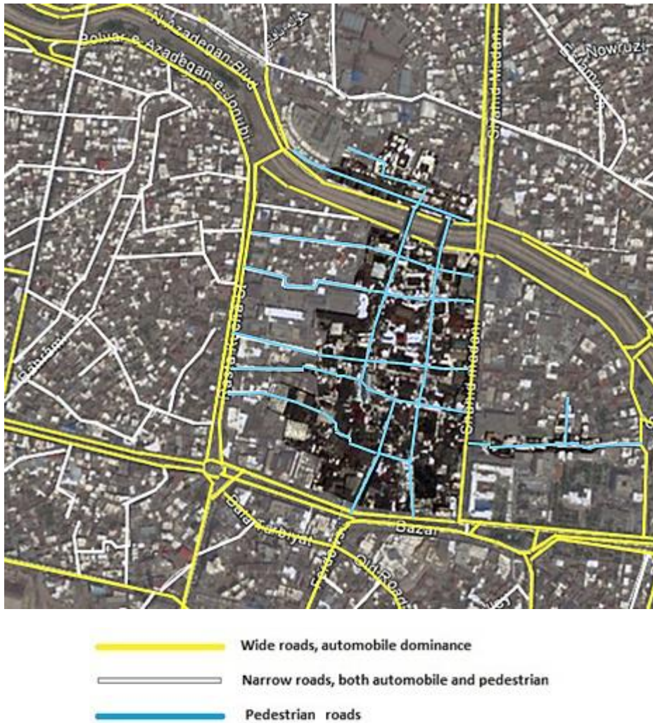
Figure 3.35. The access ways between Tabriz Bazaar and the city. In this district, most of the access ways are local roads with pedestrian dominance. In addition, the figure presents the continuity between covered streets of the bazaar and the cities' local roads. Source: Provided by the author after Google map
