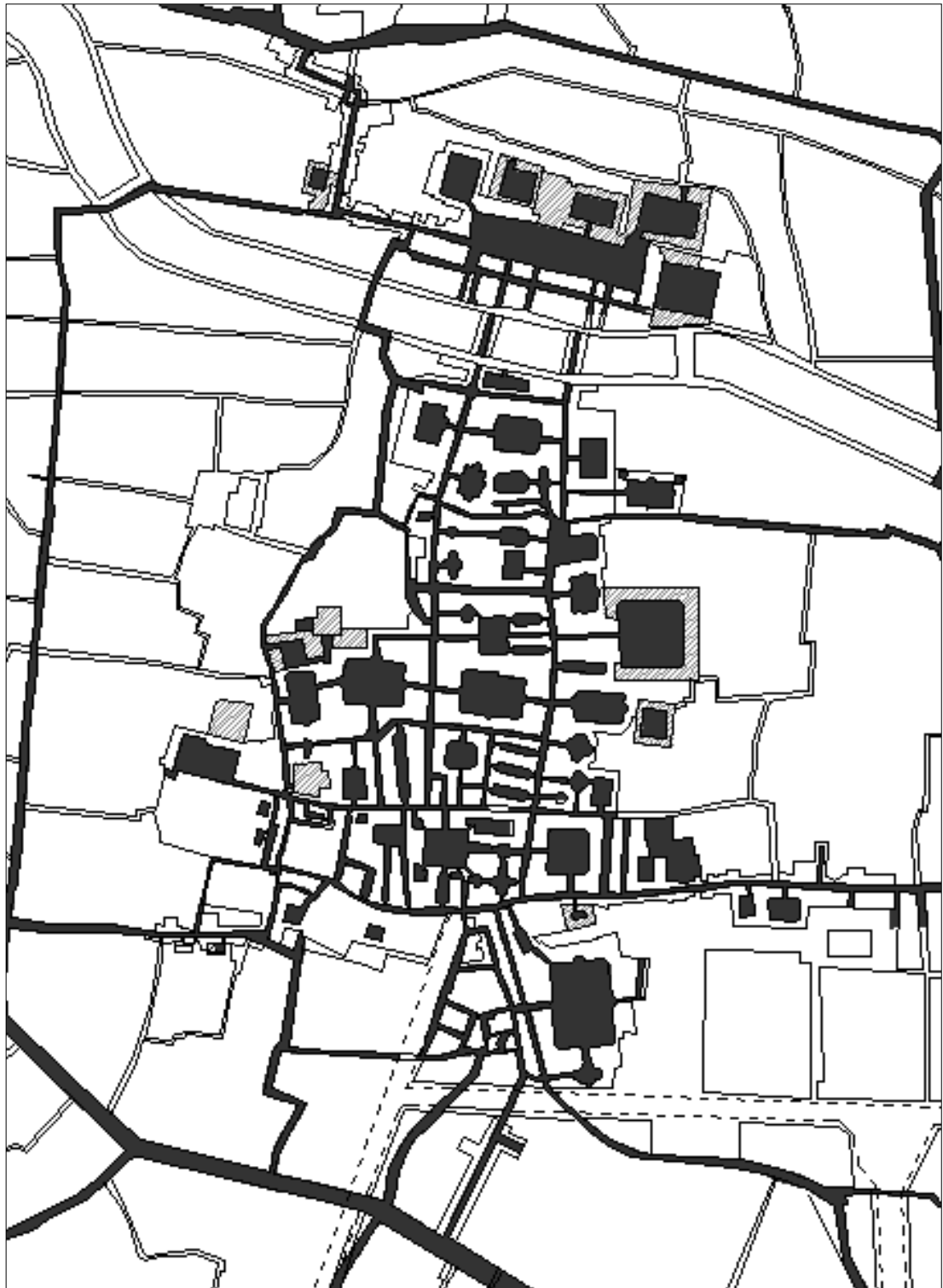
Figure 3.36. The connections of Tabriz Bazaar with the city. The map presents that the integration between inside and outside of the bazaar. This figure shows the continuity between bazaar and city structure. Source: Provided by the author after Soltanzade, H. 2001, p.65.
