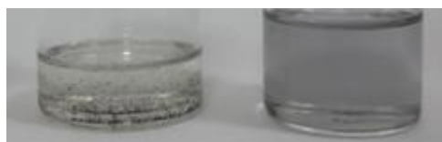
Figure 3. 37 Image of CTAB capped GNRs (left), ODT capped GNRs (right) in chloroform media
