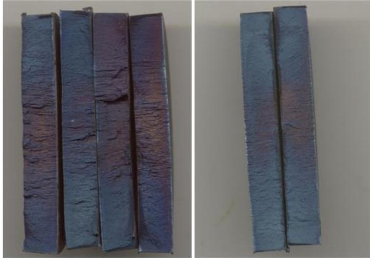
**Figure 4. 2** Blue fracture samples taken from defected areas which does not contain inclusion (left) Exp. Heat 07 - Ø72 mm, (right) Exp. Heat 06 – Ø 75 mm
