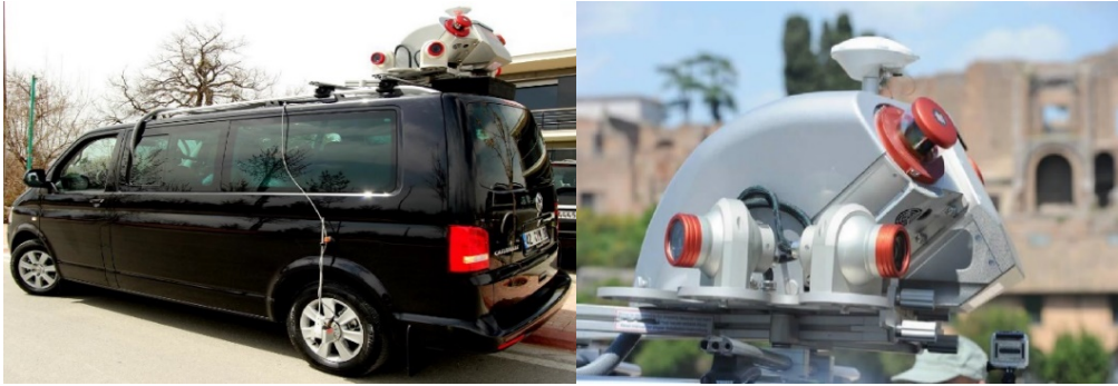
Figure 1-4 Mobile Laser Scanner System mounted on top of a vehicle
