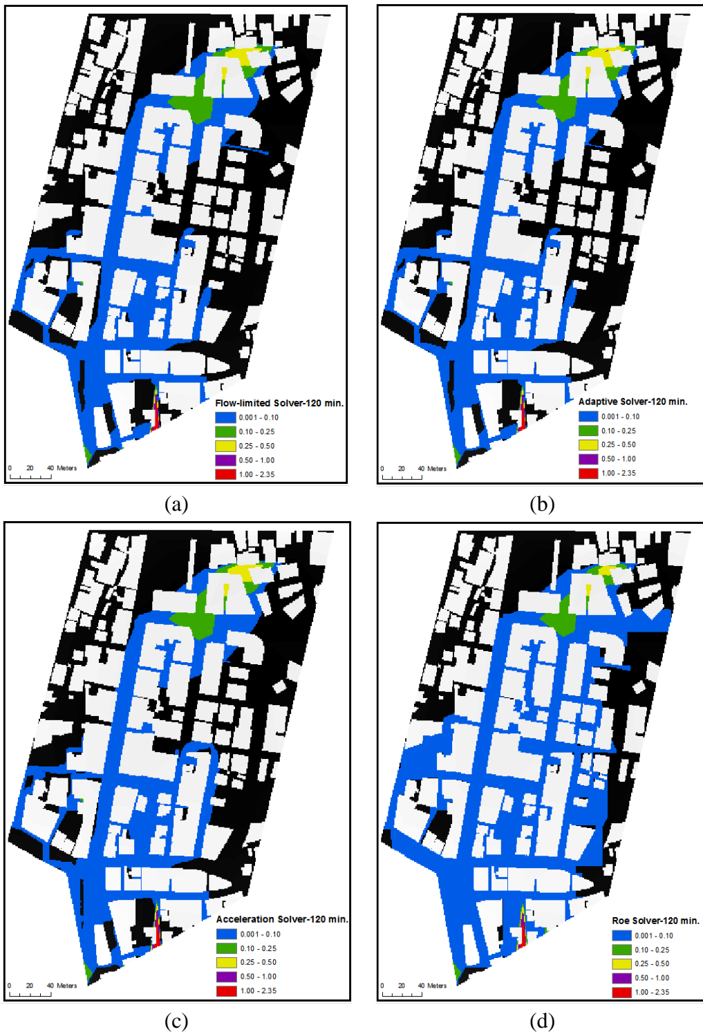
Figure 3-9 Results of Inundation Extents of (a) Flow-limited, (b) Adaptive, (c) Acceleration and (d) Roe solvers at t=120 min.
