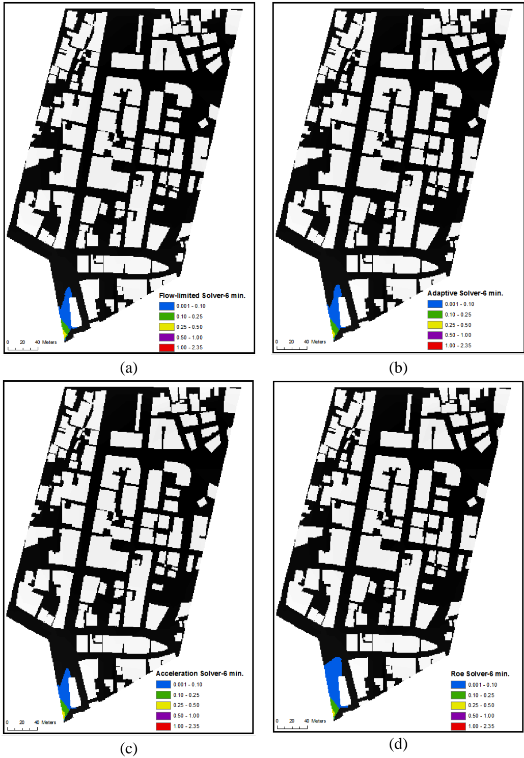
Figure 3-5 Results of Inundation Extents of (a) Flow-limited, (b) Adaptive, (c) Acceleration and (d) Roe solvers at t=6 min.
