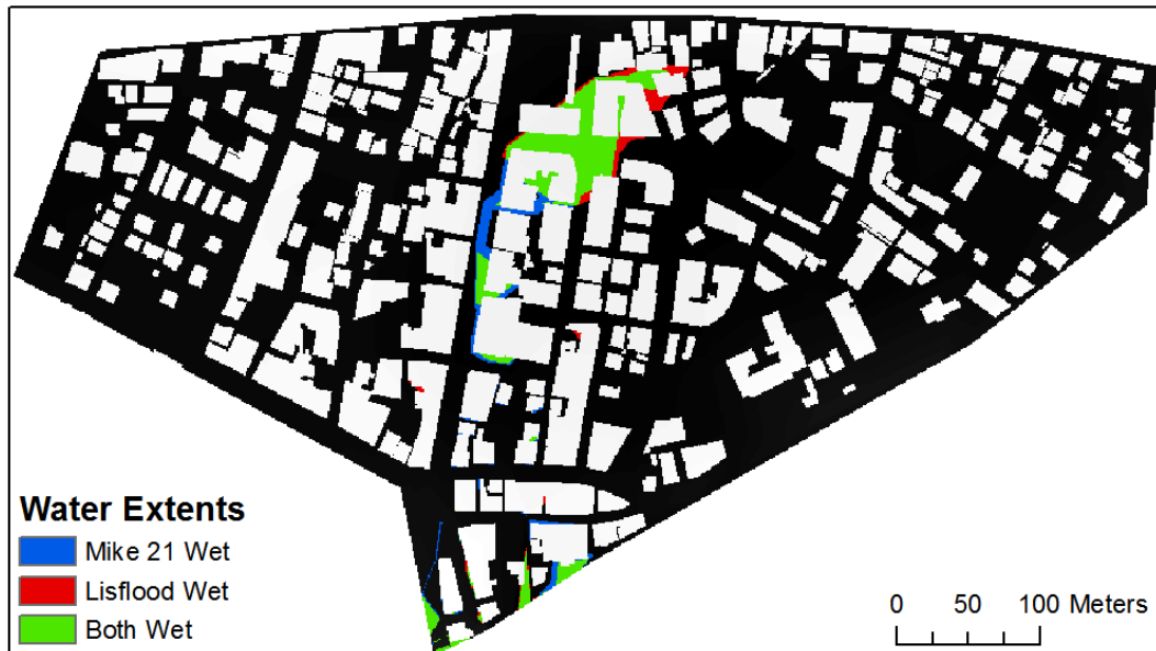
Figure 4-14 Graphical representation of differences between Lisflood-FP and Mike 21 models in terms of inundation extents at t=120 min.
