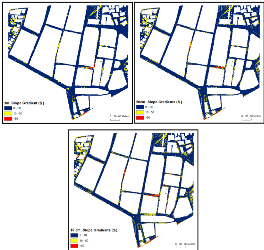
Figure 5-2 Slope Gradients of the DEMs
