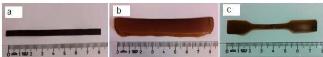
Figure 14. The images of the extruded strip (a), the rolled film (b) and the dog bone shaped film before the tensile testing.
