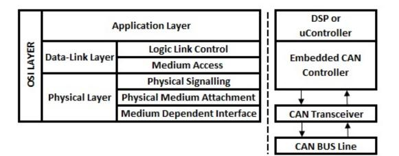
Figure 2.1: The Layered ISO 11898 Standard Architecture
