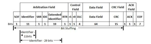
Figure 2.2: std CAN Frame Format
