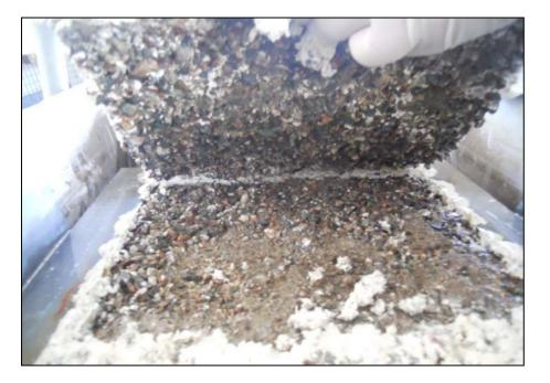
Figure 3.9 Gravel-Clay Interface in Large Shear Box Tests
