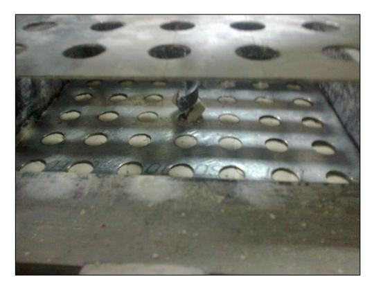
Figure 5.2 Filling Clay up to Dowel Installation Level
