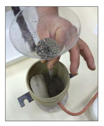
Figure 4.13 Filling Upper Part of Sand-Clay Interface Specimen with Sand
