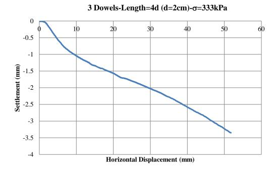
Figure C.19 Settlement vs. Displacement Graph-Experiment 10
