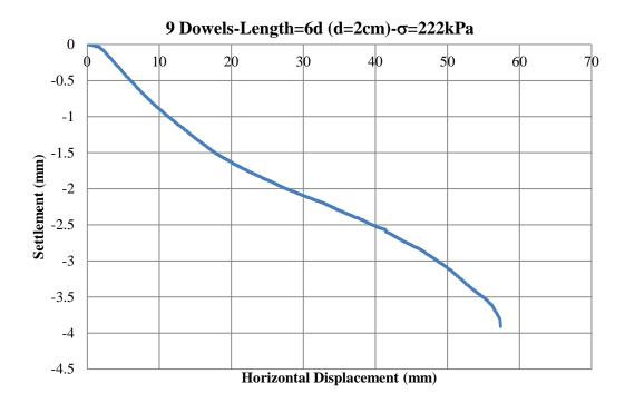
Figure C.47 Settlement vs. Displacement Graph-Experiment 24
