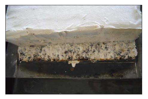
Figure 3.8 Large Shear Box Tests of Gravel-Clay Interface
