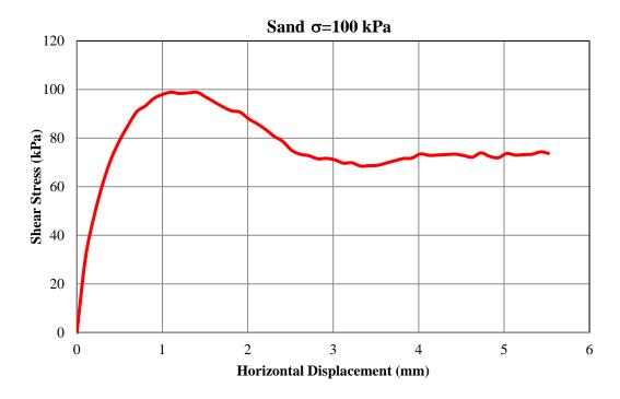
Figure A.57 Shear Stress vs. Displacement Graph-Experiment 4
