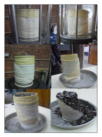
Figure 4.24 Gravel-Clay Interface Triaxial Tests during and after Experiments
