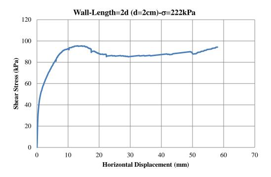
Figure C.74 Shear Stress vs. Displacement Graph-Experiment 3
