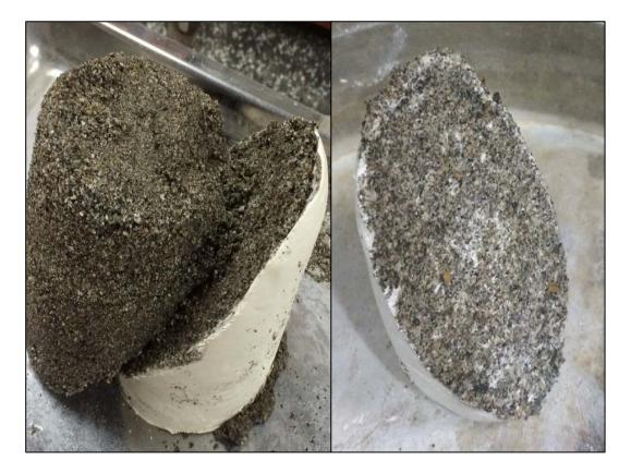
Figure 4.31 Sand-Clay Interfaces after Triaxial Tests
