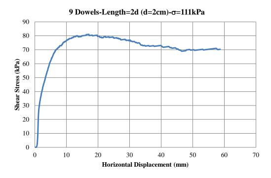
Figure C.36 Shear Stress vs. Displacement Graph-Experiment 19
