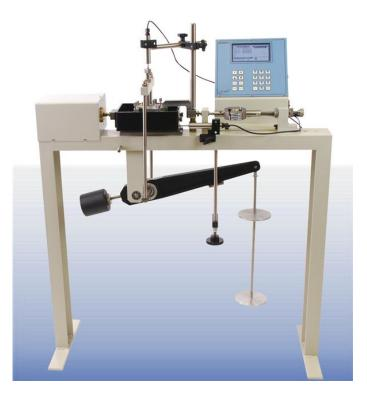
Figure 3.16 General View of Small Shear Box Machine
