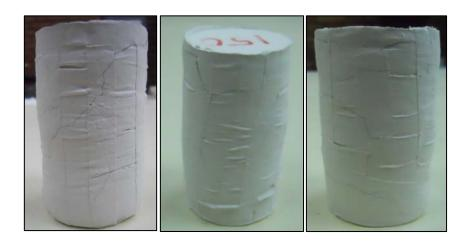
Figure 4.2 Clay Specimens after Triaxial Tests
