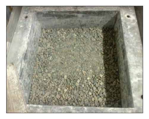
Figure 5.1 Gravel in the Lower Part of the Large Shear Box
