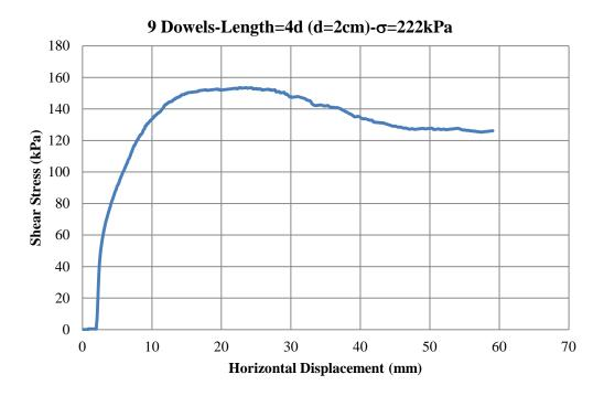
Figure C.26 Shear Stress vs. Displacement Graph-Experiment 14
