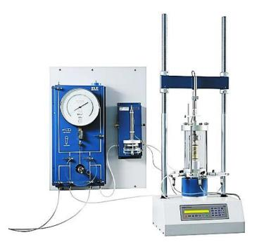
Figure 4.1 Triaxial Testing Apparatus
