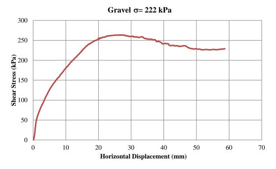
Figure A.3 Shear Stress vs. Displacement Graph-Experiment 2
