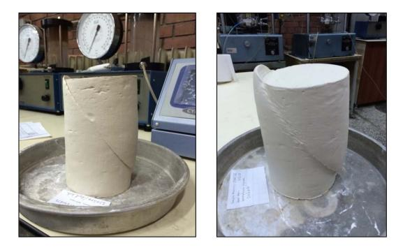
Figure 4.16 Clay-Clay Specimen after Triaxial Tests
