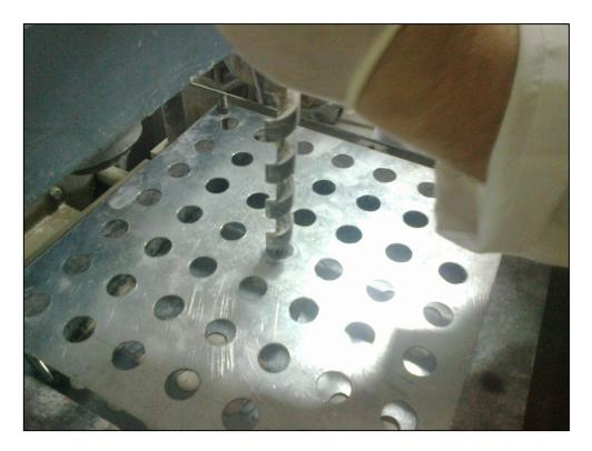
Figure 5.3 Drilling Model Dowel Holes
