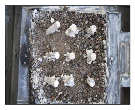
Figure 5.8 Improvement Tests with 9 Model Dowels-Dowel Length=8cm (I-3)
