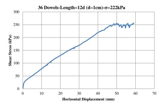
Figure C.68 Shear Stress vs. Displacement Graph-Experiment 35
