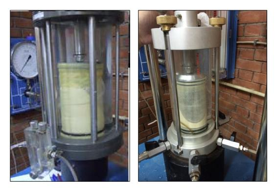
Figure 4.14 Triaxial Testing of Interfaces
