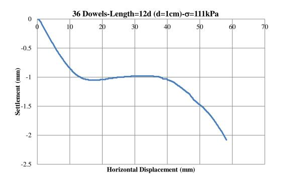
Figure C.61 Settlement vs. Displacement Graph-Experiment 31
