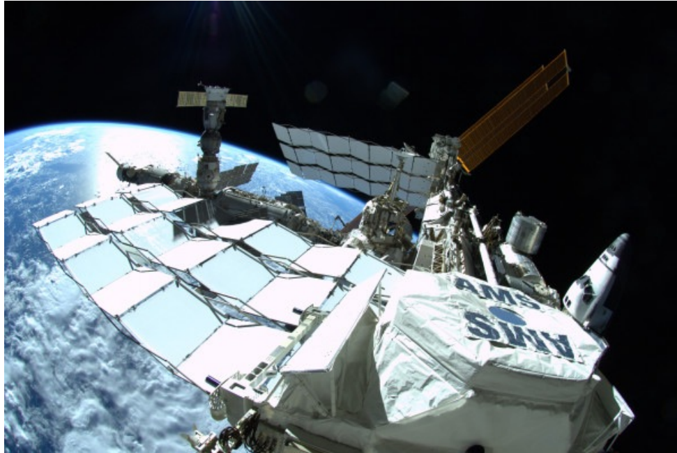
Figure 1.1: A photo of AMS-02 (right bottom) after it was installed on the ISS. In this picture, taken on July 12 ,2011, radiators and solar panels of ISS can be seen as well. This photo was taken during a space walk by the astronauts living on ISS [48].
