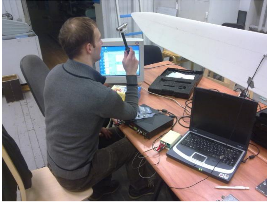
Figure 2.17. An Experimental Modal Analysis Setup Example [25]
