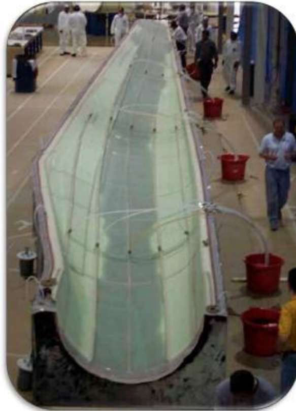
Figure 2.12. A Blade Production Setup [13]
