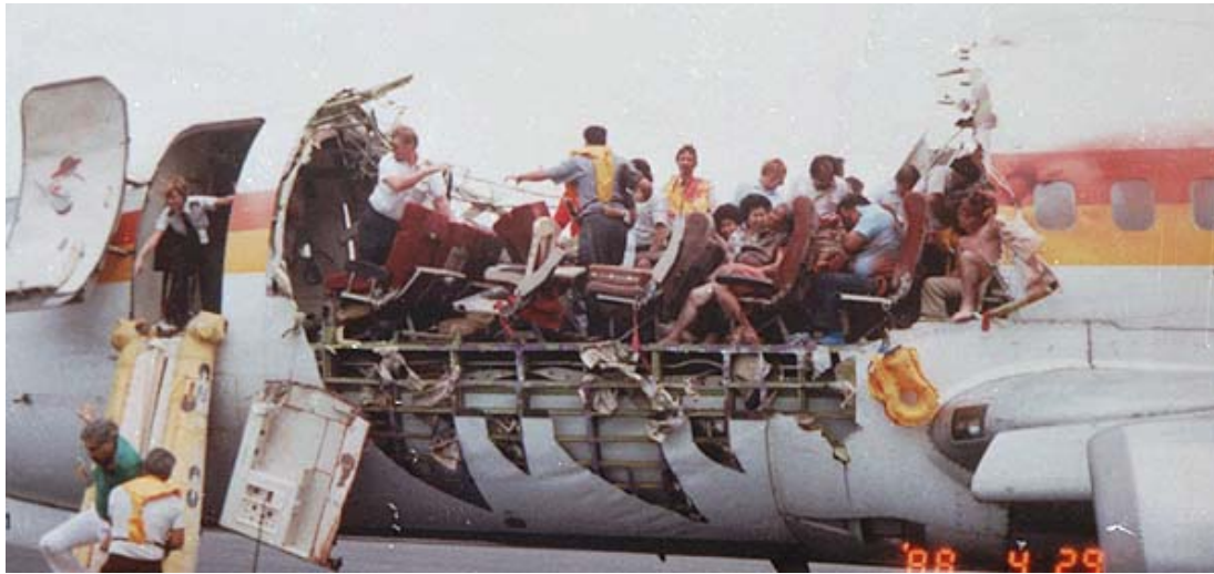
Figure 1.1. The Aloha Airlines Boeing 737 at Honolulu International Airport, Hawaii, following the accident on April 28, 1988.
