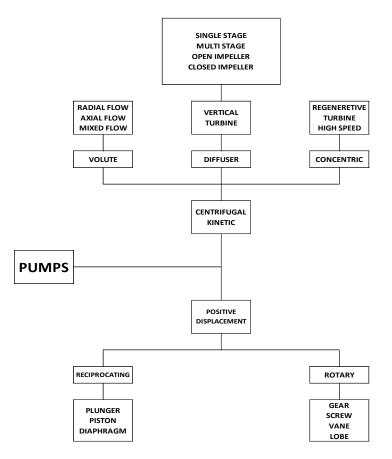
Figure 2.10 General Pump Classification (Modified after Bachus and Custodio,
