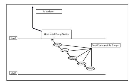
Figure 2.2 Underground Mine Dewatering
