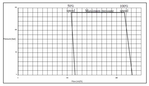
Figure 2.11 Positive Displacement Pump Curve (Kuenen, 2010)
