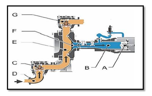
Figure 2.8 Suction Position of Positive Displacement Pump (Weir Minerals, 2012) A: Piston, B: Propelling Liquid, C: Suction Valve, D: Suction Line, E: Slurry Chamber, F: Diaphragm, G: Discharge Valve
