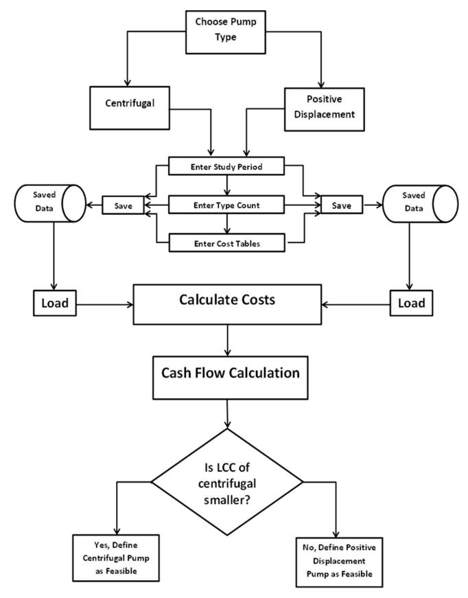
Figure 3.1 Flow chart algorithm of program
