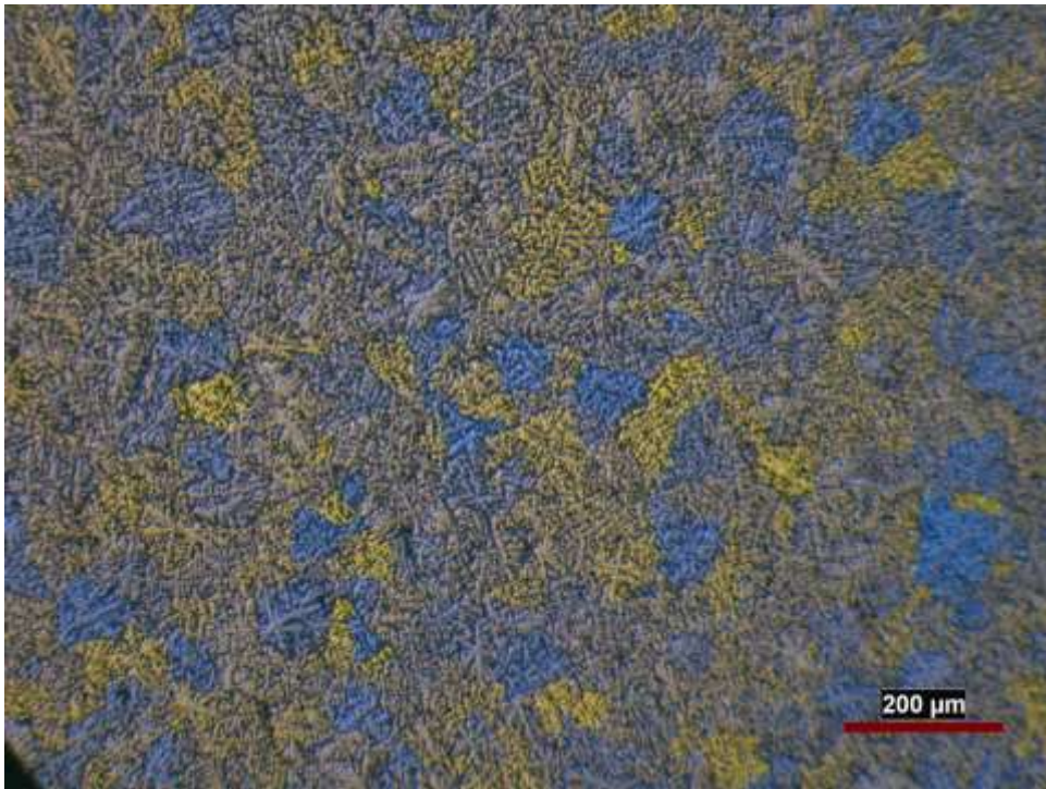
Figure 4. 16 Weld Zone - 5x Magnification
