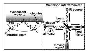
Figure 14: The schematic illustration of an ATR-FTIR instrument (Thomas, 2009)
