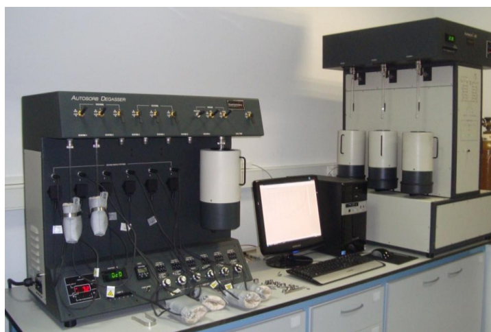
Figure 3.3. Surface area and pore size analyzer (right) and degassing unit (left) (Central Laboratory, METU)
