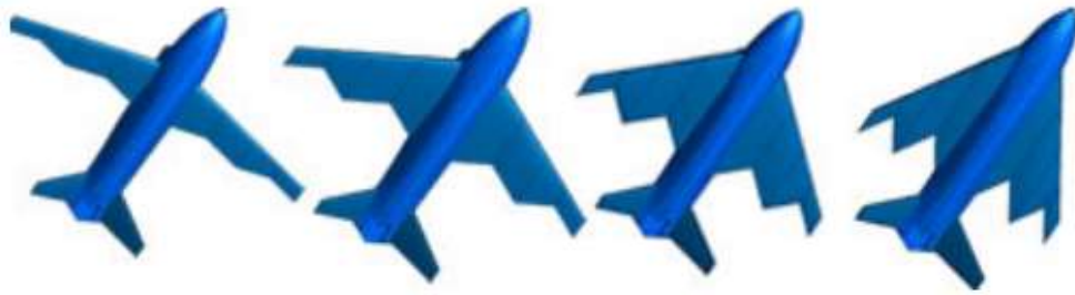
Figure 1-15 Nextgen aeronautics' design of the morphing wing [23]
