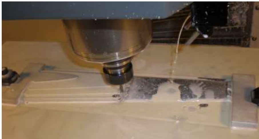
Figure 2-12 Manufacturing of the wings with CNC milling method
