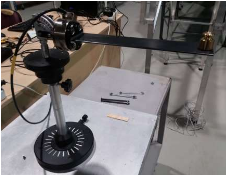
Figure 2-26 Eccentric load sensitivity test
