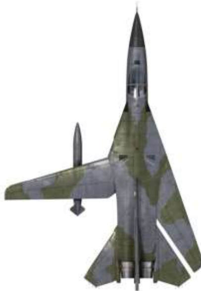
Figure 1-11 F-111 Different sweep orientation [19]
