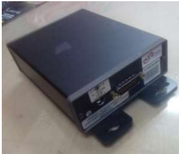
Figure 2-24 Load Power Amplifier/Supply
