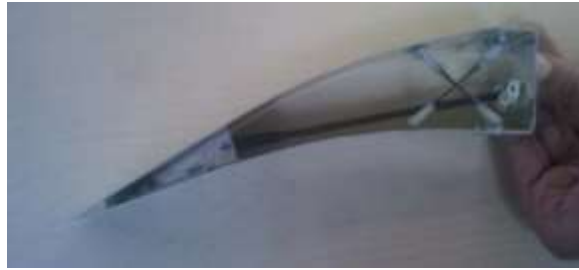
Figure 1-22 Hingeless control surface: increased camber [27]
