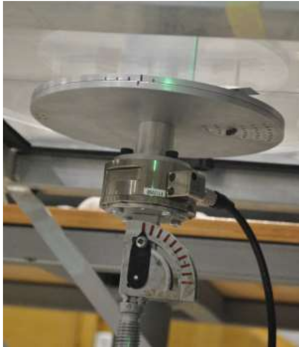
Figure 2-23 6-Axis Loadcell mounted on test setup
