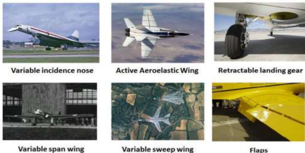
Figure 1-3 Discrete morphing mechanisms [6]
