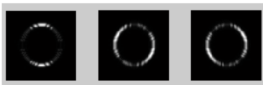
Figure 4.21: Gabor filtered images whose edges are detected depending on the orientation of the filter. (3 orientation)
