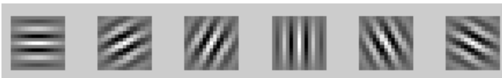
Figure 4.19: Gabor filter bank having fixed scale, but different orientations.
