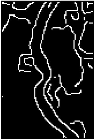
Figure 4.29: PMAD is applied prior to the application of Canny edge detector.
